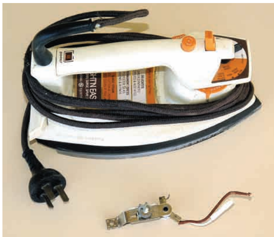
Every discarded electric iron has a thermostat mounted inside. These snap-action thermostats can be used to switch at temperatures from about 60°C to 200°C.
