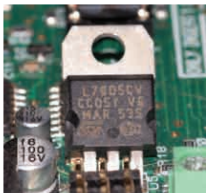
Fig.1. This voltage regulator is a 7805, which means it is a +5V regulator that can handle a maximum current of one amp. The other markings are of no practical importance to users and should be ignored
