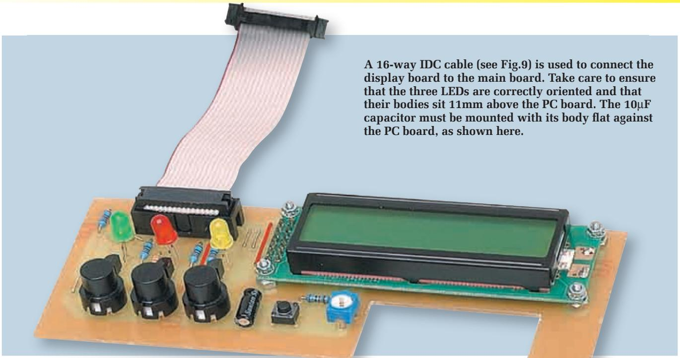
A 16-way IDC cable (see Fig.9) is used to connect the display board to the main board. Take care to ensure that the three LEDs are correctly oriented and that their bodies sit 11mm above the PC board. The 10 $\mu$ F capacitor must be mounted with its body flat against the PC board, as shown here.
