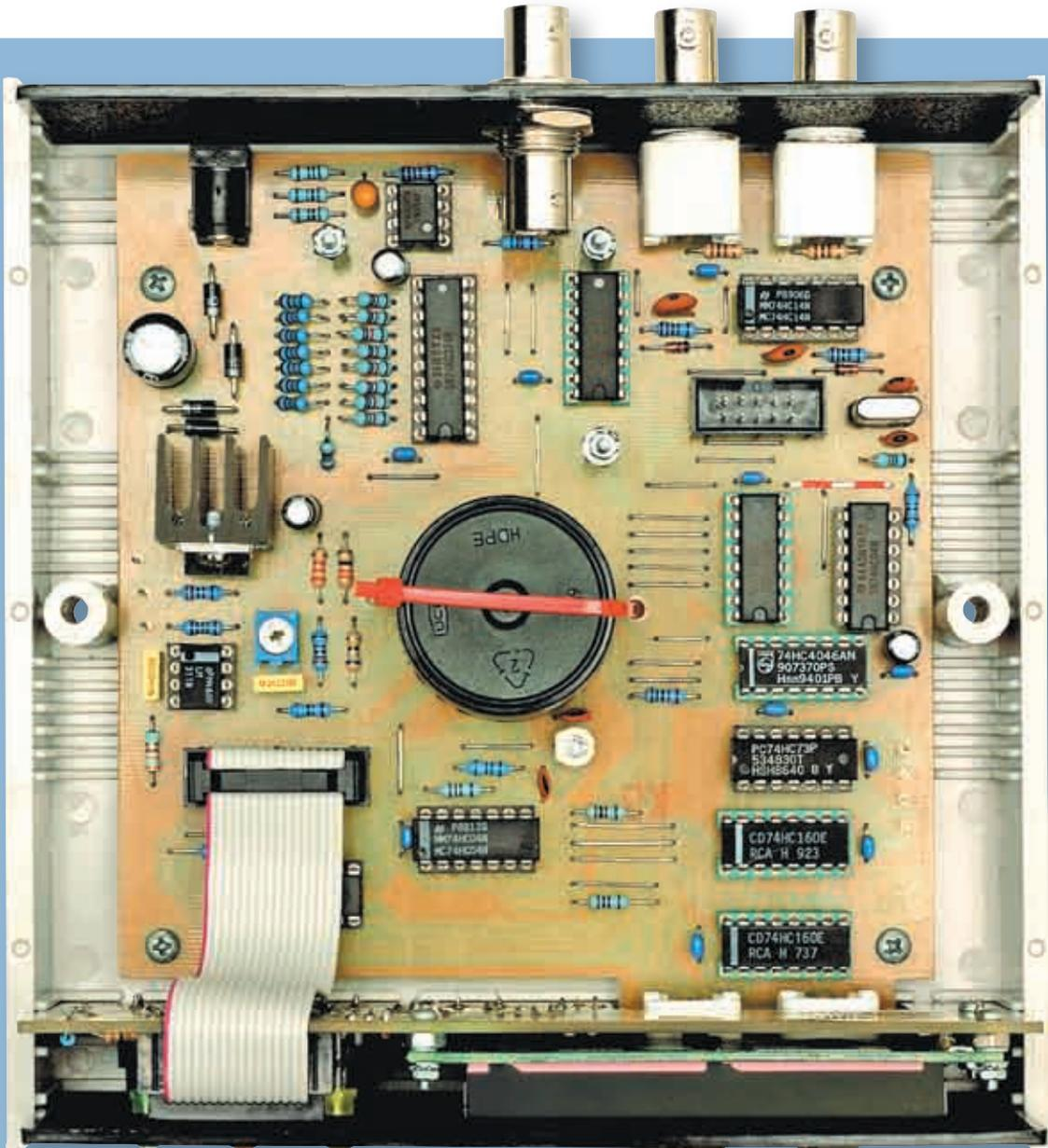
The main PC board is secured to integral spacers on the base of the case, while the display board slides into one of the case slots. Note that the front and rear panels must be attached to the BNC sockets on the main board before mounting it in the case.
