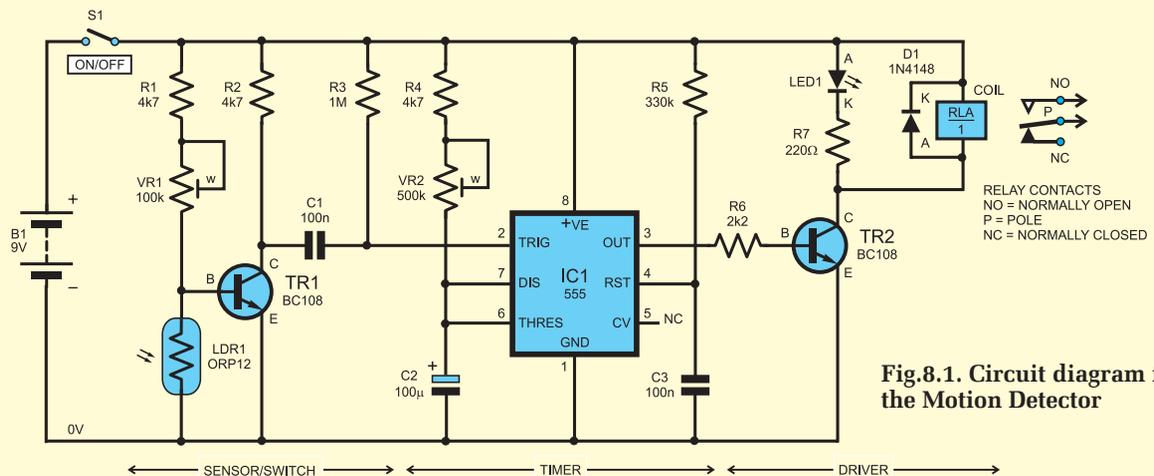
Fig.8.1. Circuit diagram for the Motion Detector
