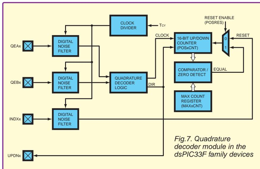
Fig.7. Quadrature decoder module in the dsPIC33F family devices
