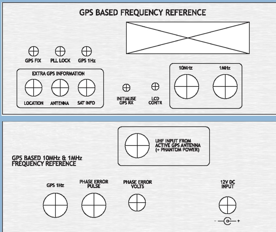
Fig.12: these full-size artworks can be copied and used to make the front and rear panels.
