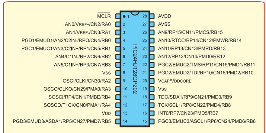
Fig.1. PIC24HJ128GP202 pinout
