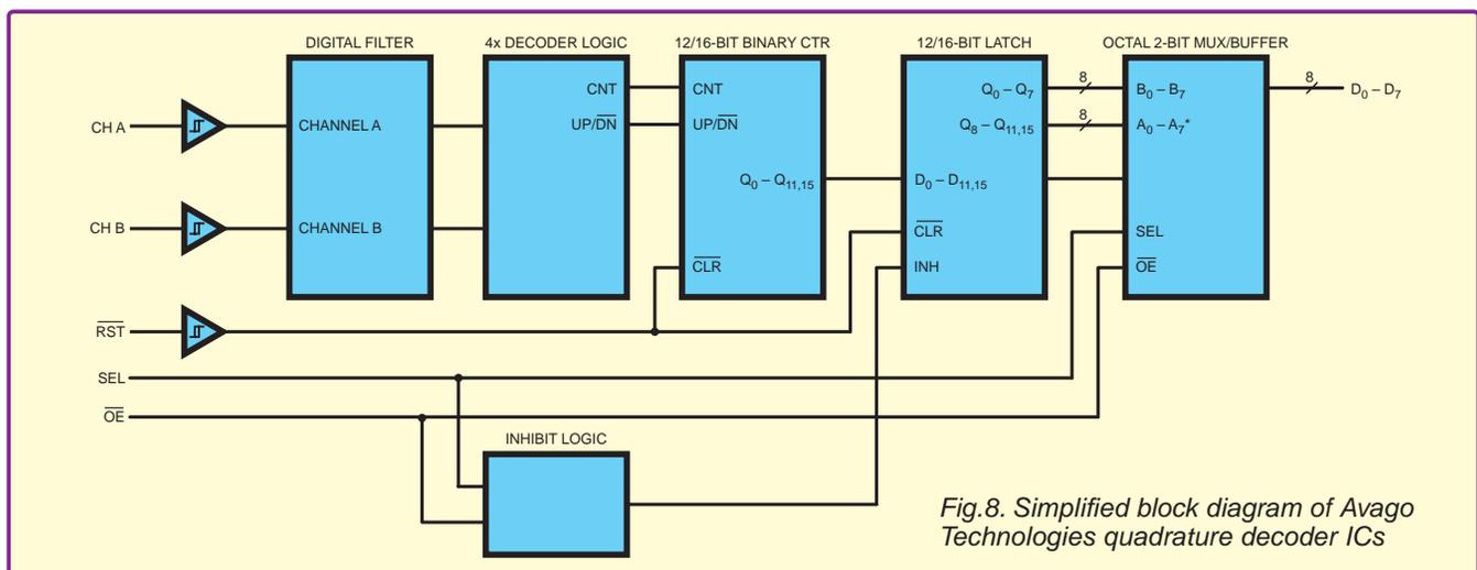
Fig.8. Simplified block diagram of Avago Technologies quadrature decoder ICs
