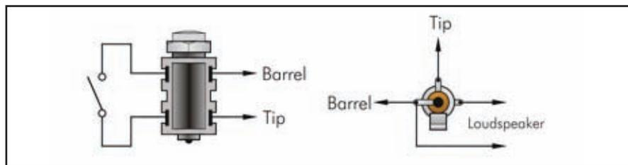
Fig.3. Connection details for an insulated jack socket (left) and an open construction miniature jack socket (right). With most projects, the extra tags for the switch contacts are left unused
