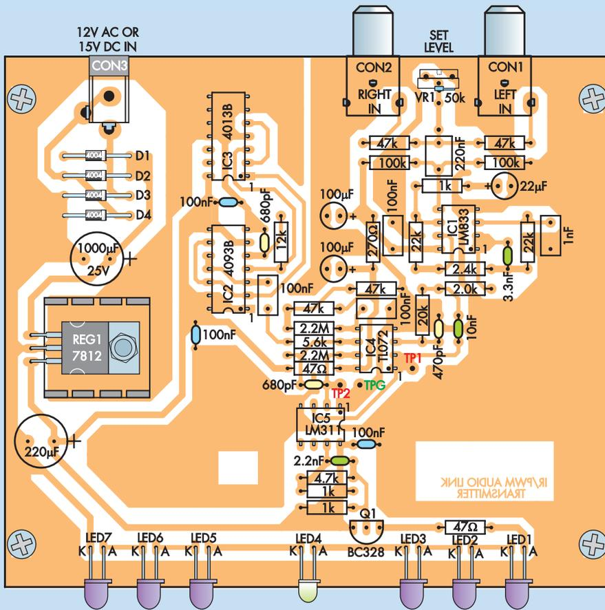
Fig.7: install the parts on the transmitter board as shown here, taking care to ensure that all polarised parts are correctly orientated. Below is a full-size photo of the assembled PC board.
