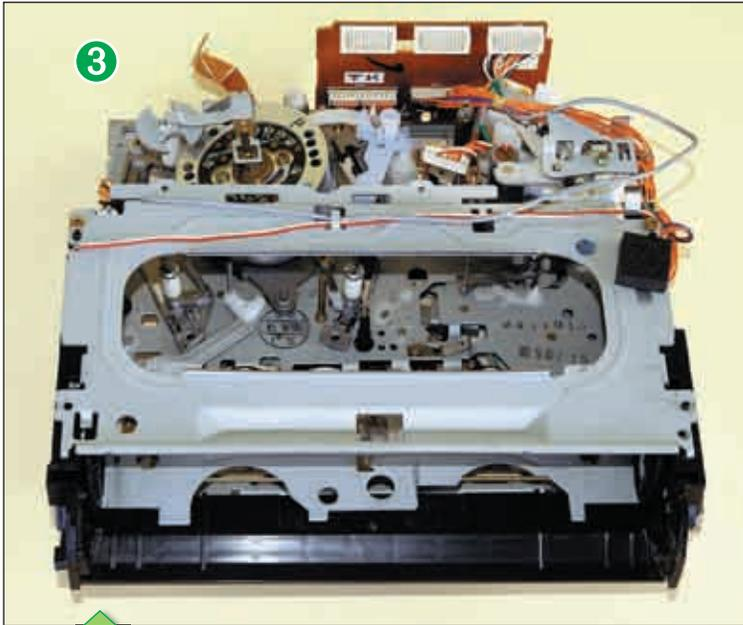
Here's the inner chassis on its own. At this stage, the contents of the VCR have already been narrowed down to just this and the PC boards. Throw the rest away as you remove it – ie, the top and bottom covers, the front cover and the inner plastic chassis.
