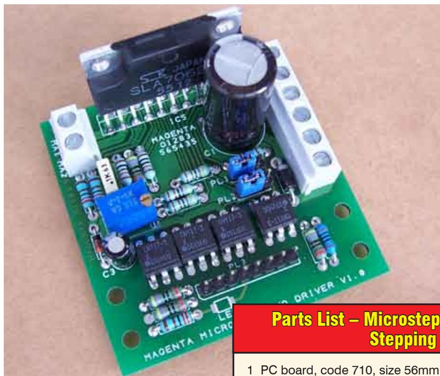
Components mounted on the topside of the printed circuit board. Stepper motor driver IC5 is mounted on the PCB with its 'thermal tab' pointing away from the top edge of the board
