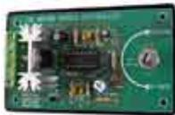
Control the speed of almost any common DC motor rated up to 100V/7.5A. Pulse width modulation output for maximum motor torque at all speeds. Supply: 5-15Vdc. Box supplied.
