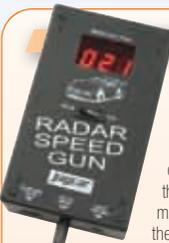
simply with two coffee tins fitted end to end. The circuit needs 12VDC at only 130mA so you can use a small SLA or rechargeable battery pack.
