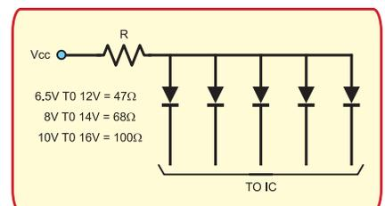
Fig. 8.4. When using a higher supply voltage, insert a resistor in series with the LEDs
