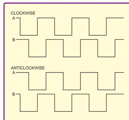
Fig.5. Quadrature signals from the incremental encoder shown in Fig.4a, starting from sensor positions shown in Fig.4b (With logic 0 for black and logic 1 for white)
