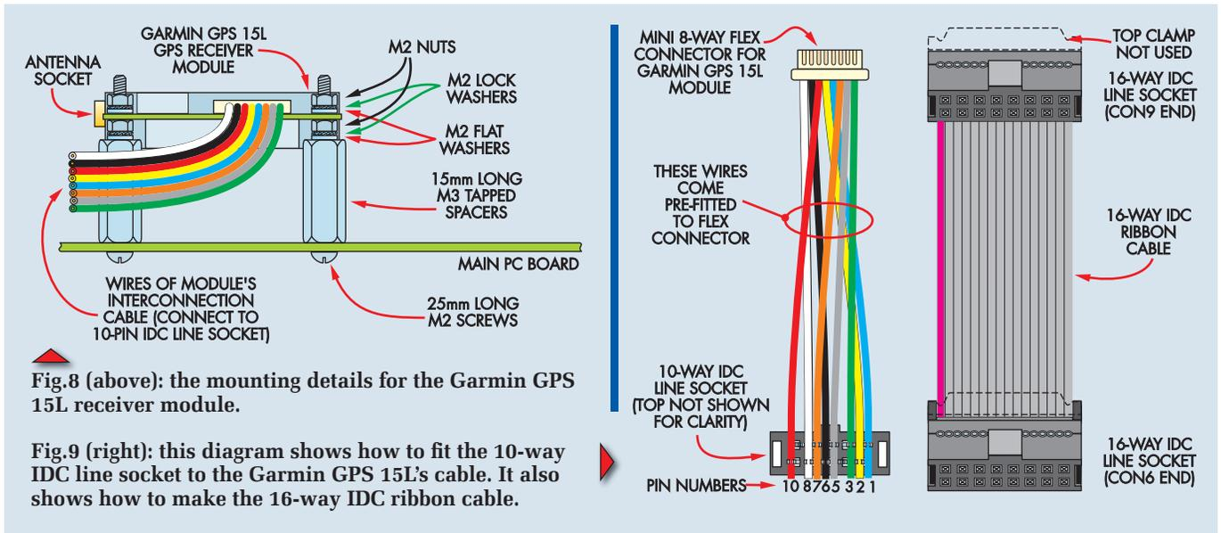
Fig.8 (above): the mounting details for the Garmin GPS 15L receiver module.
