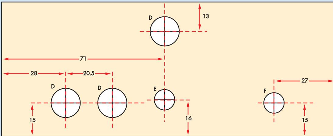
Fig.11: these diagrams show the drilling details for the front and rear panels.
