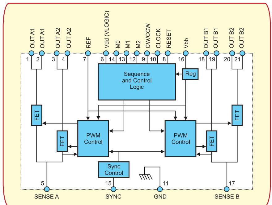
Fig.1: Simplified internal block schematic and functional diagram for the SLA7062M stepper motor translator/driver IC
