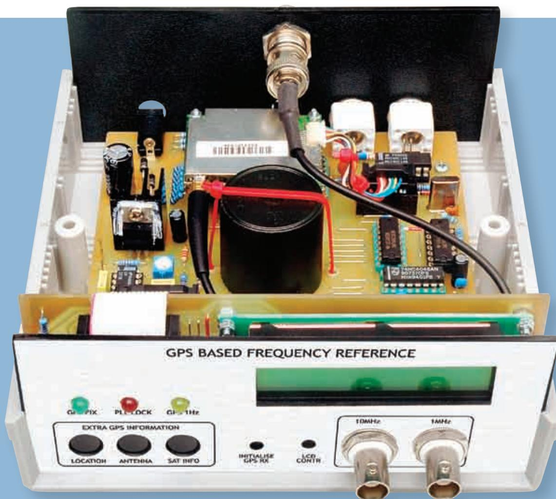
This view shows the fully-assembled unit, with both the Garmin receiver and the oven cover in place. Note the internal antenna connection from the Garmin GPS 15L receiver's socket to the BNC-to-BNC adapter on the rear panel (see also picture on facing page).
