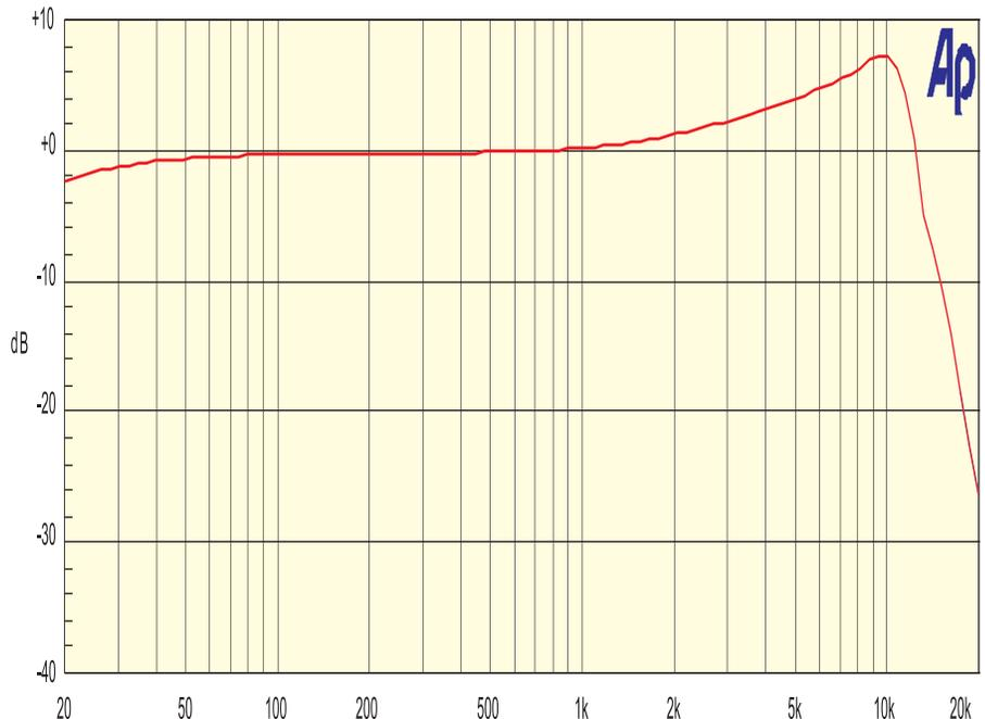
**Fig.6:** this graph plots the audio frequency response of the system. Note that a small amount of treble boost is applied from about 1kHz (rising to a maximum of 7dB at 8kHz) to improve intelligibility on speech.
