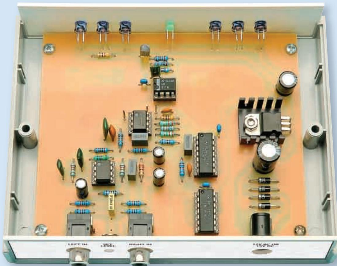
Here's another view inside the completed transmitter. Note the lead dress on the infrared LEDs and the green indicator LED, so that they protrude through their matching holes in the front panel.
