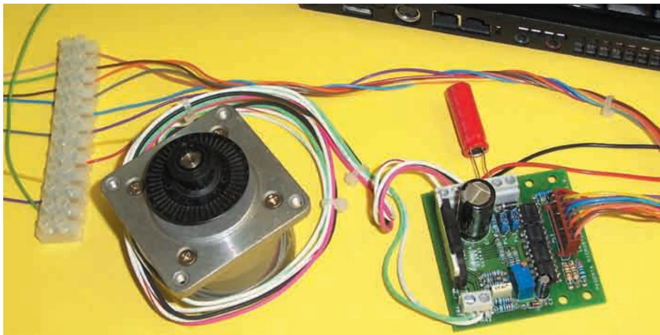
The completed circuit board linked to a small 200 step motor. Note the motor decoupling electrolytic capacitor wired directly between terminal blocks TB3 and TB4. It should have a *minimum* value of  $470\mu\text{F}$ , see text
