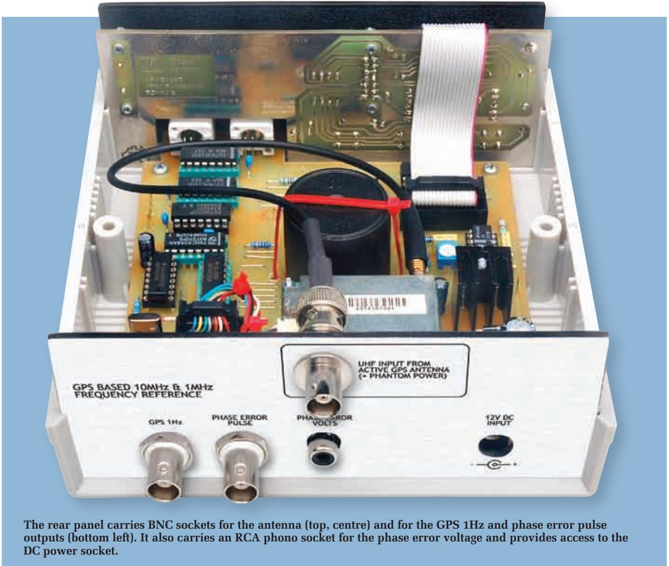
The rear panel carries BNC sockets for the antenna (top, centre) and for the GPS 1Hz and phase error pulse outputs (bottom left). It also carries an RCA phono socket for the phase error voltage and provides access to the DC power socket.
