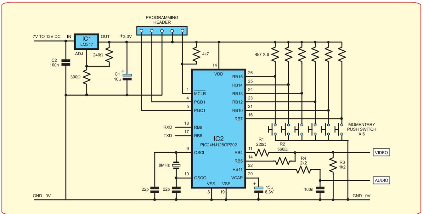
Fig.2. Video generation circuit diagram
