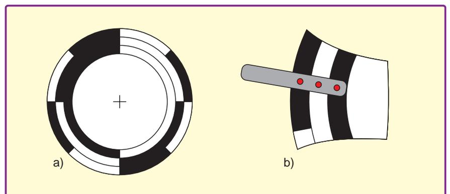
Fig. 2. (a) Disc patterned with binary code, (b) arrangement of sensors
