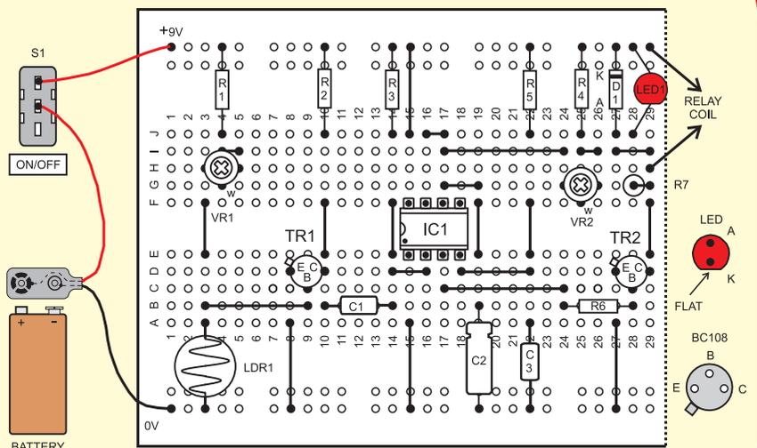
Fig.8.2. Motion Detector breadboard component layout
