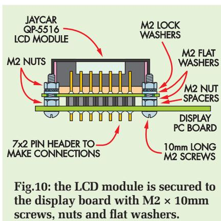
Fig.10: the LCD module is secured to the display board with  $M2 \times 10\text{mm}$  screws, nuts and flat washers.
