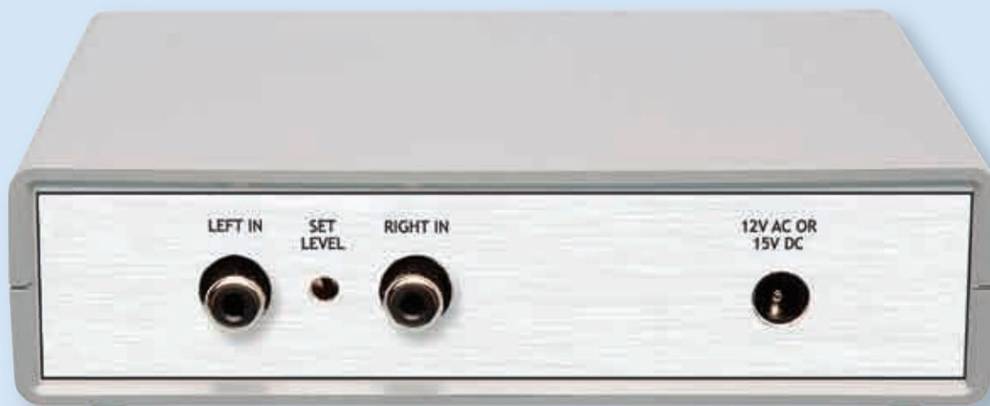
The rear panel of the receiver has clearance holes for the two audio input phono sockets, plus access holes for the 'Set Level' trimpot and the power socket. Power can come from a 12V AC or 15V DC (regulated) plugpack.
