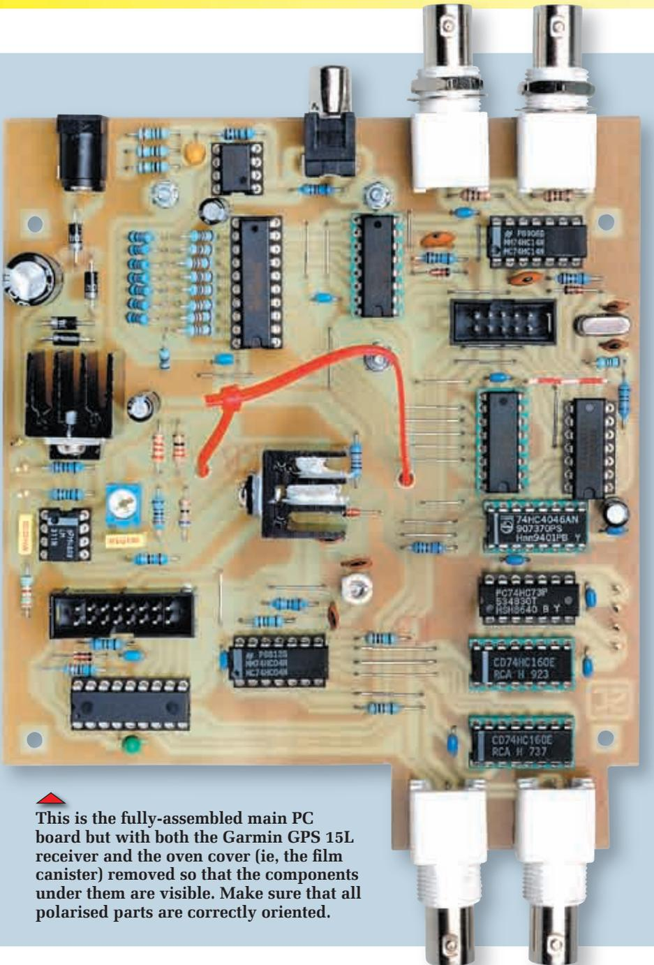
▲ This is the fully-assembled main PC board but with both the Garmin GPS 15L receiver and the oven cover (ie, the film canister) removed so that the components under them are visible. Make sure that all polarised parts are correctly oriented.
