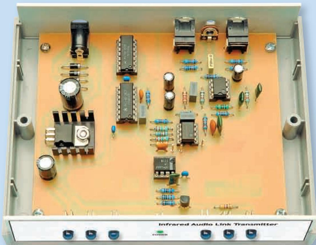
The completed transmitter PC board is installed in a low-profile instrument case and secured using four self-tapping screws that go into integral mounting posts in the base. We used IC sockets for the prototype, but you can solder the ICs directly to the PC board.
