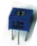
This is a preset type that can be inserted directly into the Protobloc and its value adjusted with a small screwdriver
