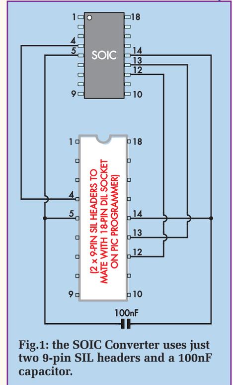
Fig.1: the SOIC Converter uses just two 9-pin SIL headers and a 100nF capacitor.
