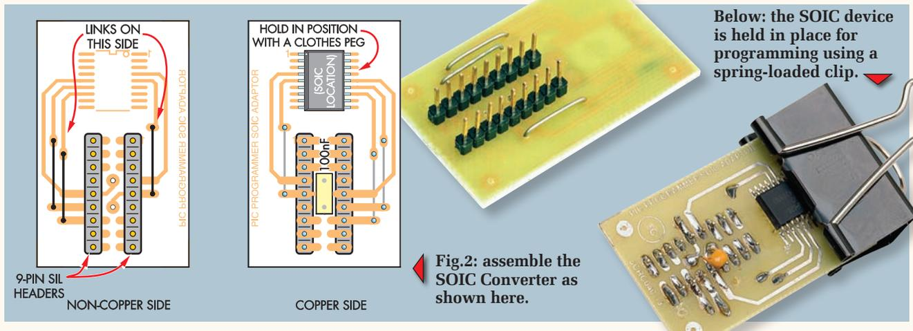
Fig.2: assemble the SOIC Converter as shown here.
