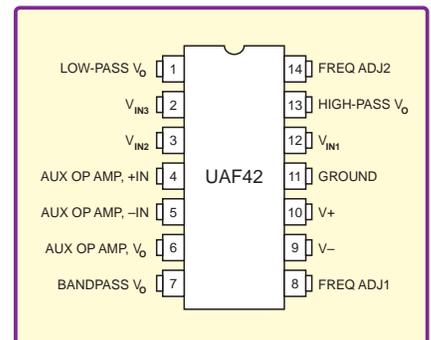
Fig.5. Pinout connections for the UAF42 universal filter IC from Texas Instruments
