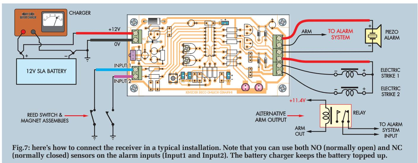
Fig.7: here's how to connect the receiver in a typical installation. Note that you can use both NO (normally open) and NC (normally closed) sensors on the alarm inputs (Input1 and Input2). The battery charger keeps the battery topped up.
