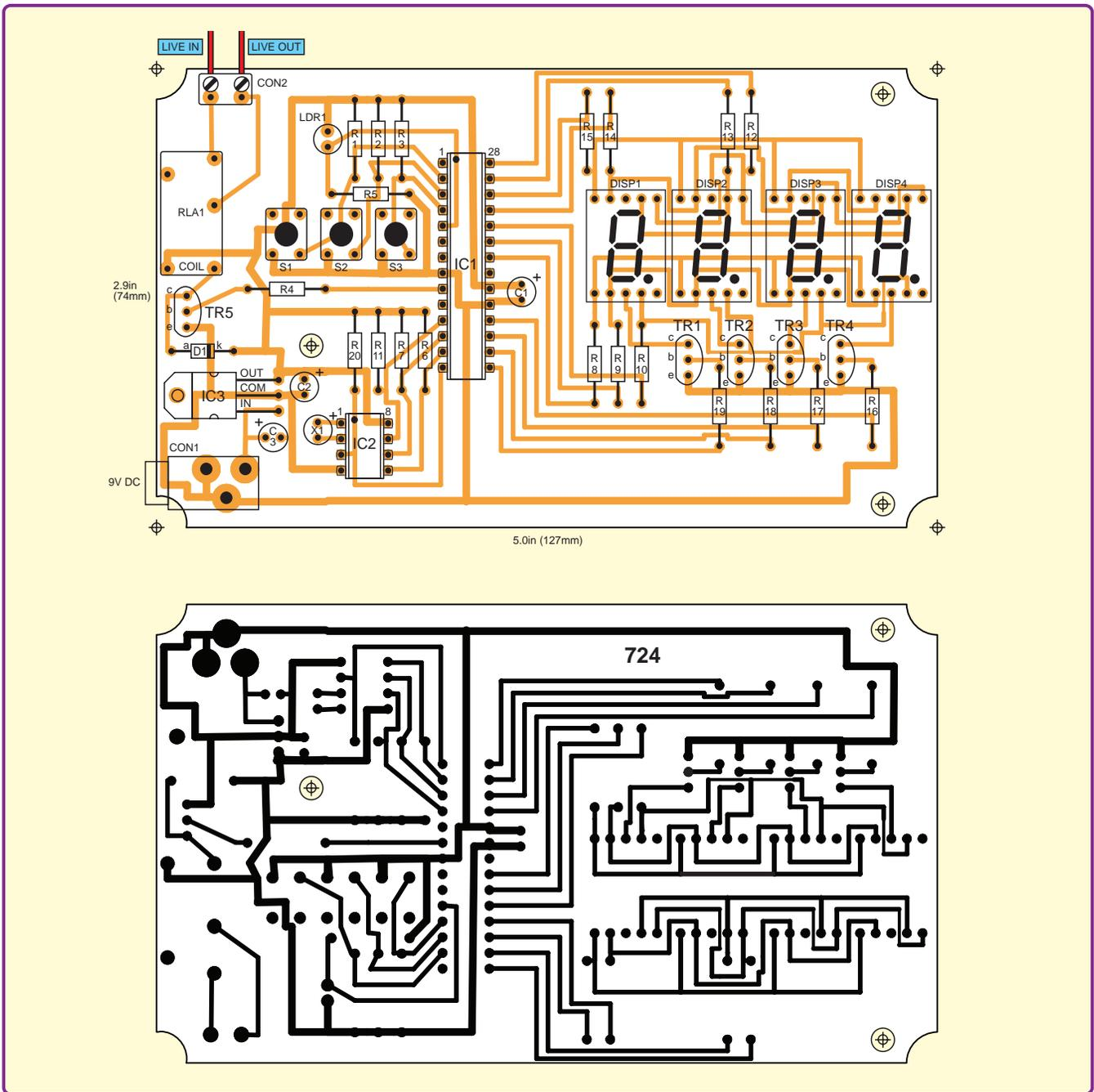
**Fig.6. Topside printed circuit board component layout and full-size copper foil master for the Random Mains Timer. Note: the mains relay contacts must be suitably rated to control the appliance being used**
