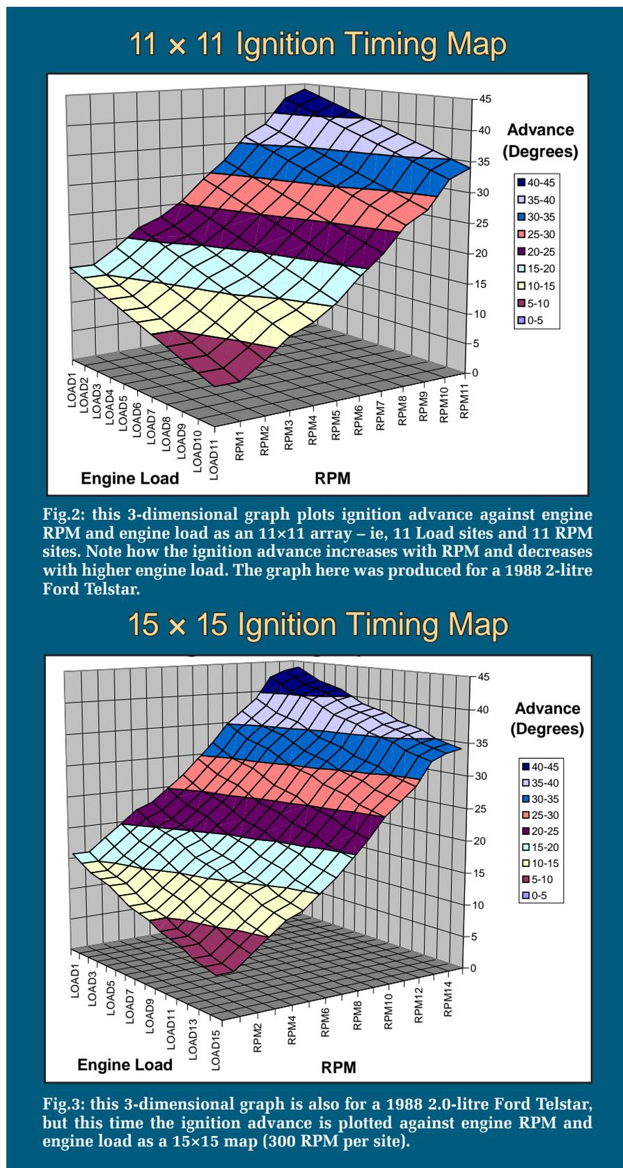
Fig.2: this 3-dimensional graph plots ignition advance against engine RPM and engine load as an 11x11 array – ie, 11 Load sites and 11 RPM sites. Note how the ignition advance increases with RPM and decreases with higher engine load. The graph here was produced for a 1988 2-litre Ford Telstar.
