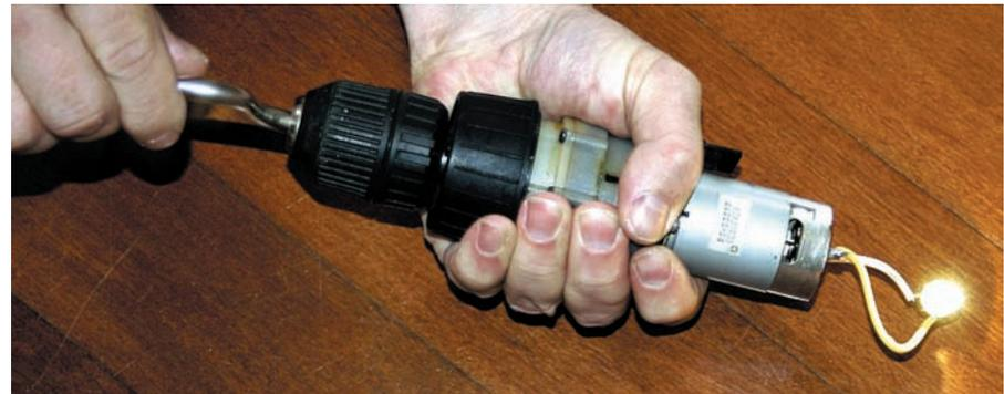
One of the easiest uses of the innards of a discarded cordless electric drill is as a hand-cranked DC generator. In this application, the gearbox steps-up the rotational speed of the chuck, allowing up to 0.5A at 5V to be generated with ease – quite good for such a small generator!
