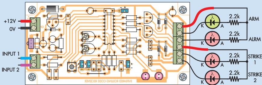
**Fig.6:** the test LEDs are connected to the receiver as shown here. Follow the procedure in the text to synchronise the transmitters and test the receiver.
