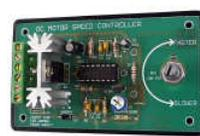
Control the speed of almost any common DC motor rated up to 100V/7.5A. Pulse width modulation output for maximum motor torque at all speeds. Supply: 5-15Vdc. Box supplied. Dimensions (mm): 60Wx100Lx60H.
