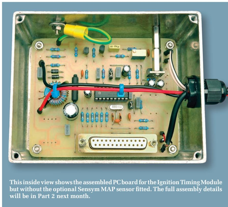
This inside view shows the assembled PC board for the Ignition Timing Module but without the optional Sensym MAP sensor fitted. The full assembly details will be in Part 2 next month.
