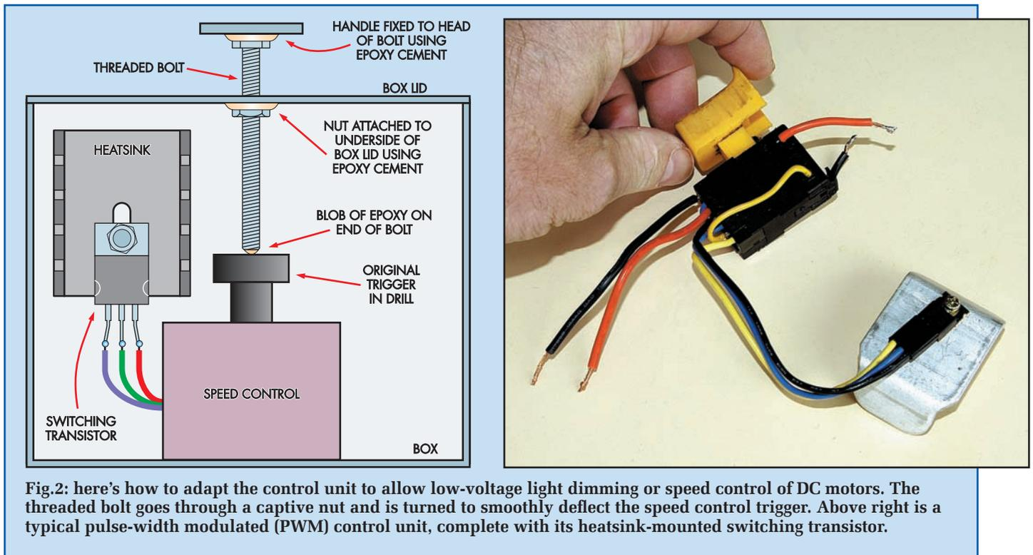
**Fig.2:** here's how to adapt the control unit to allow low-voltage light dimming or speed control of DC motors. The threaded bolt goes through a captive nut and is turned to smoothly deflect the speed control trigger. Above right is a typical pulse-width modulated (PWM) control unit, complete with its heatsink-mounted switching transistor.
