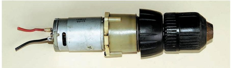
A discarded cordless drill can provide a compact and powerful drive assembly for nothing! The motor/gearbox/clutch/chuck combination can be used to drive robots, power small winches – or even be a portable drill for use on car power.
