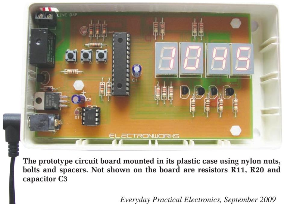
The prototype circuit board mounted in its plastic case using nylon nuts, bolts and spacers. Not shown on the board are resistors R11, R20 and capacitor C3
