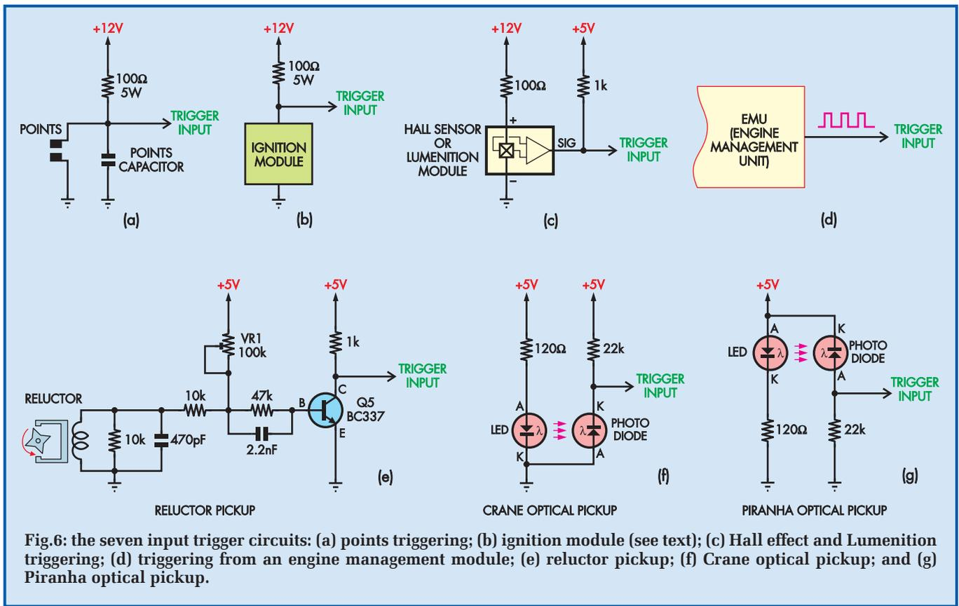
Fig.6: the seven input trigger circuits: (a) points triggering; (b) ignition module (see text); (c) Hall effect and Lumenition triggering; (d) triggering from an engine management module; (e) retractor pickup; (f) Crane optical pickup; and (g) Piranha optical pickup.
