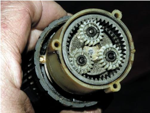
Cordless drills use planetary gearboxes to reduce the chuck speed and increase torque. Usually two back-to-back geartrains are used – this view shows the motor input side. These gearboxes are compact, have a high reduction ratio and are strong for their size.
