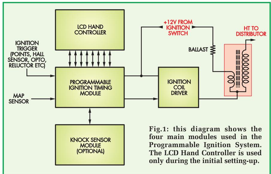
Fig.1: this diagram shows the four main modules used in the Programmable Ignition System. The LCD Hand Controller is used only during the initial setting-up.
