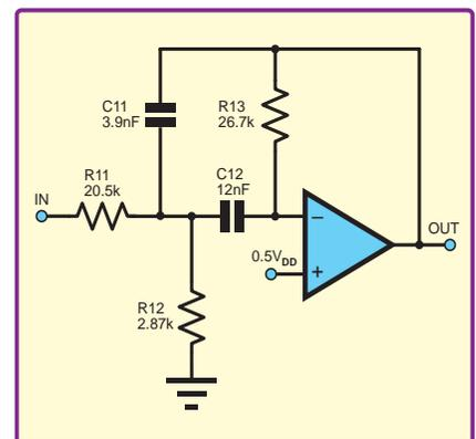
Fig.2. (below). A synthesised 2kHz to 4kHz MFB bandpass filter using Microchip's FilterLab
