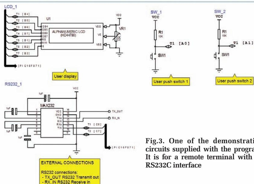
Fig.3. One of the demonstration circuits supplied with the program. It is for a remote terminal with an RS232C interface
