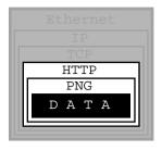
We only need to understand any protocols that tell us how to *interpret the data*, not how to *receive* it from another process, nor how to *send* it to another process.
