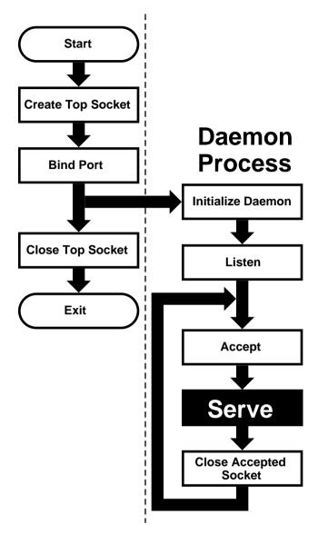
This flowchart is good for *sequential servers*, i.e., servers that can serve one client at a time, just as we were able to with our *daytime* server. This is only possible whenever there is no real "conversation" going on between the client and the server: As soon as the server detects a connection to the client, it sends out some data and closes the connection. The entire operation may take nanoseconds, and it is finished.
