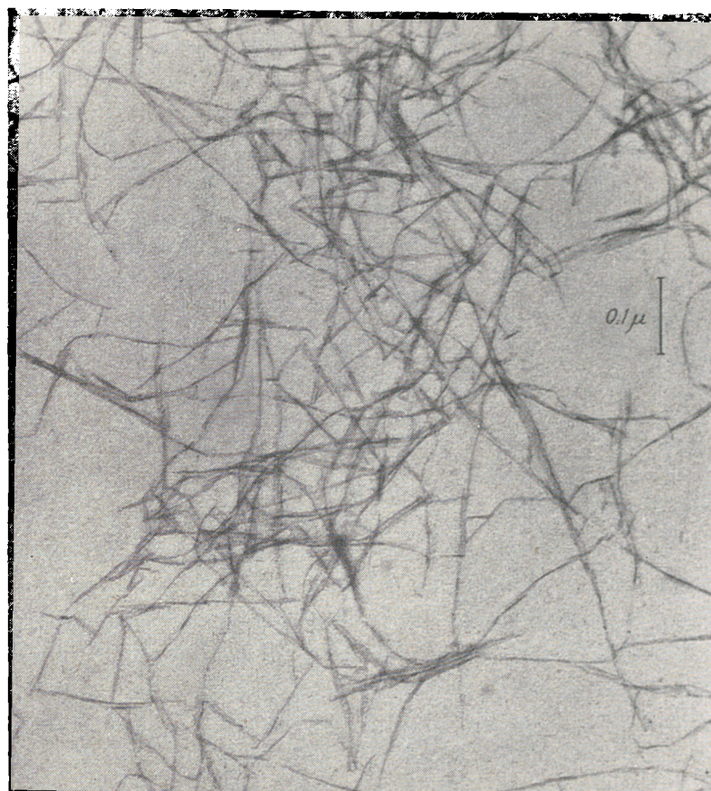
FIG. 47.12. Electron micrograph of freshly prepared vanadium pentoxide fibers. These fibers are about 25\text{\AA} wide. The limit of resolution in this micrograph is about 20\text{\AA} . (Courtesy of Dr. J. Hillier, R.C.A. Laboratories.)
