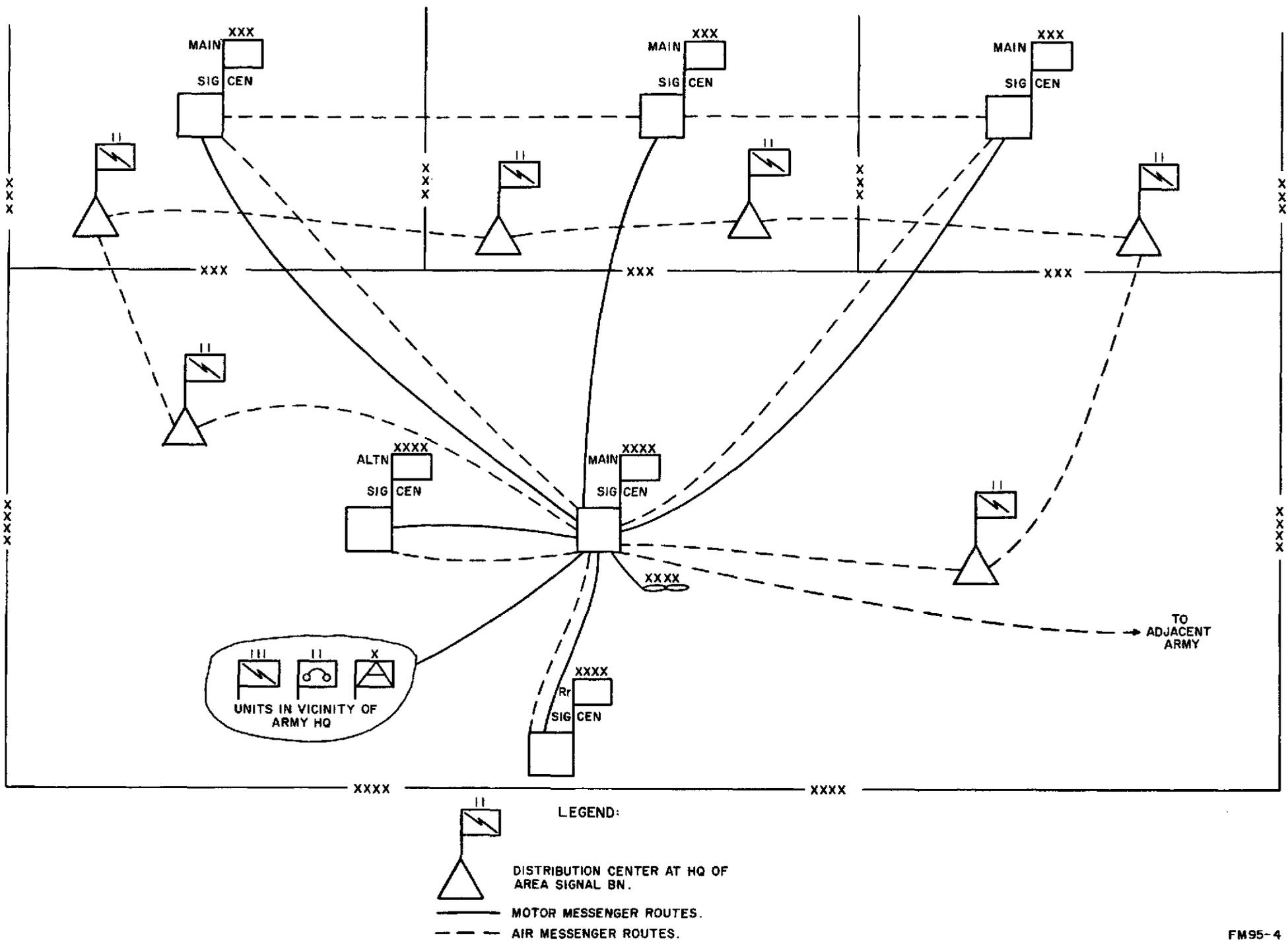
Figure 4. Type signal messenger service (field army).
