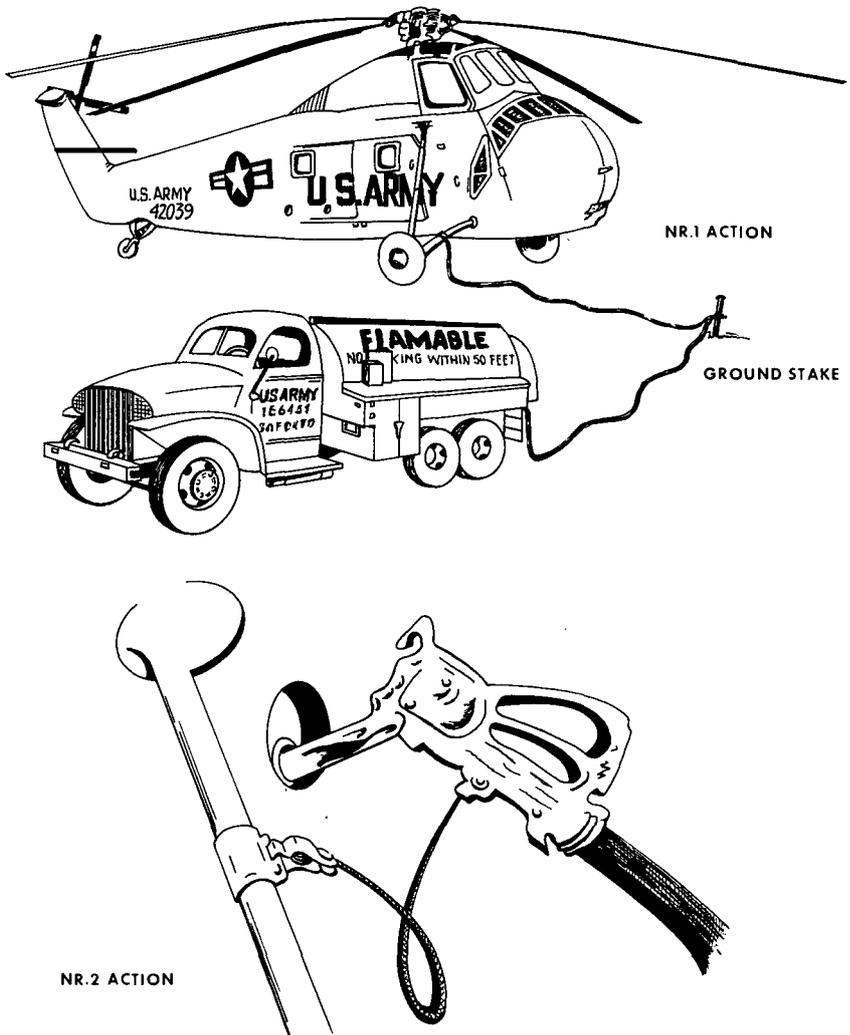
Figure 6-2. Grounding and bonding techniques for refueling operations.
