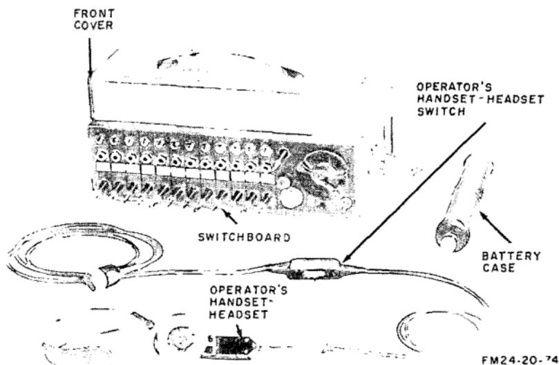
*Figure 115. Manual Telephone Switchboard SB-22/PT.*
