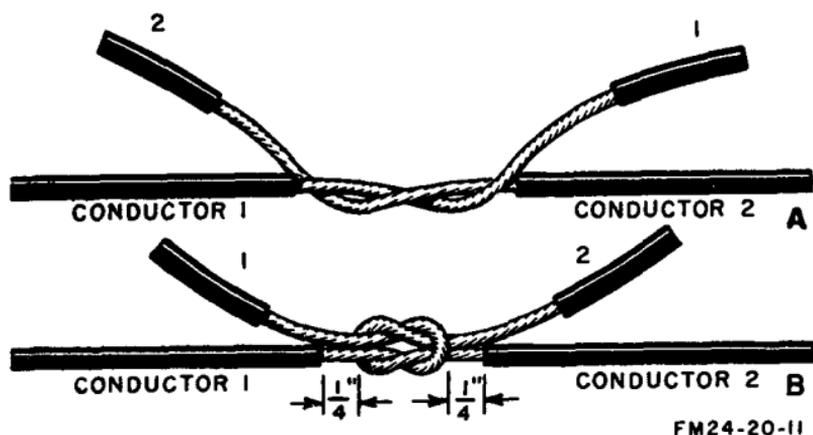
Figure 25. Tying square knot in field wire.
