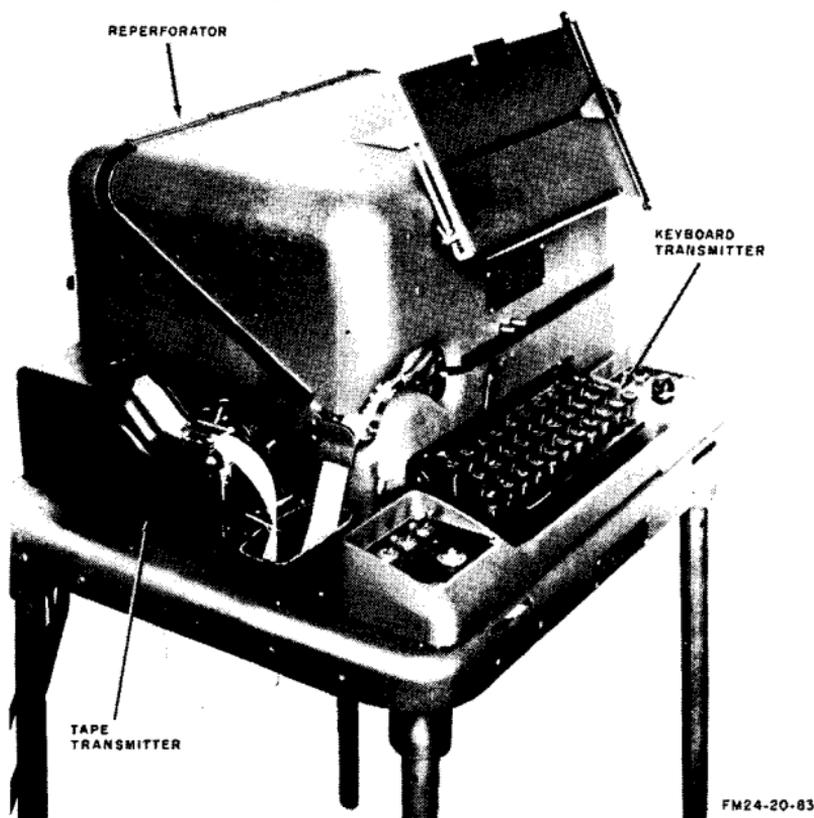
*Figure 118. Teletypewriter Set AN/GGC-3.*
