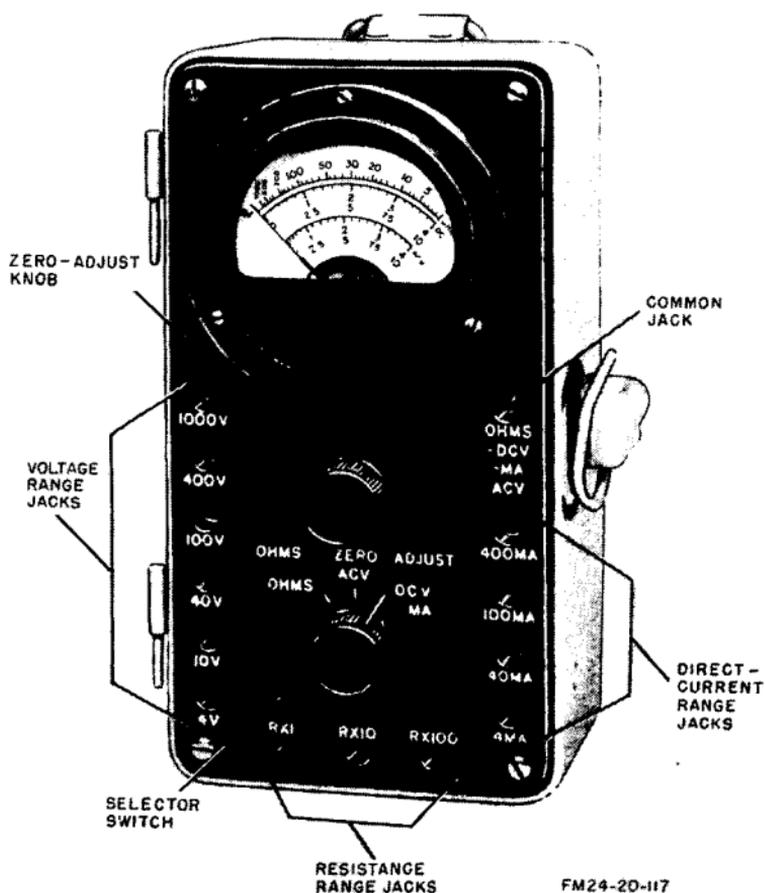
Figure 130. Multimeter TS-297/U.
