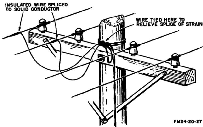
*Figure 44. Tying in field wire to open wire.*
