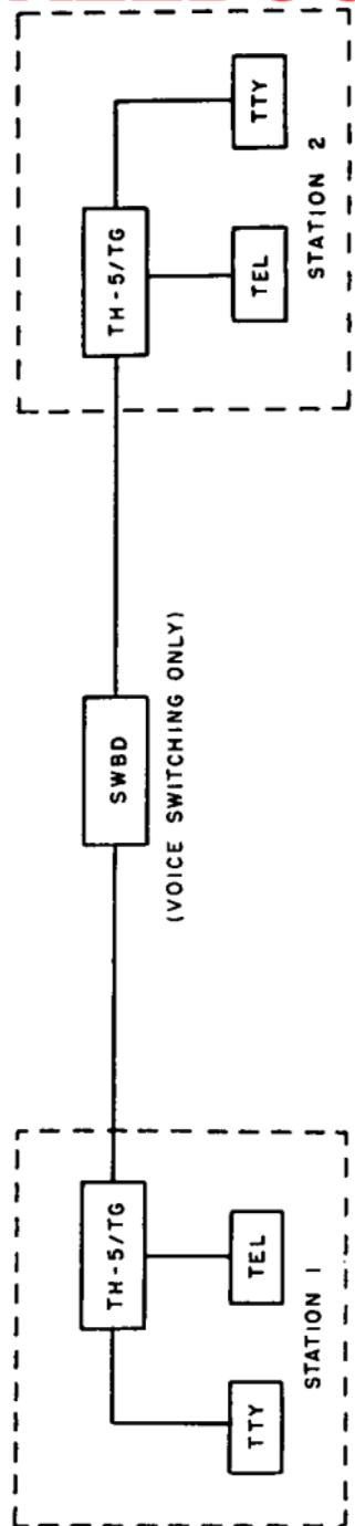
Figure 121. Alternate telegraph-telephone service on switchboard loop circuit, using Telegraph Terminal TH-5/TG. FM24-20-80
