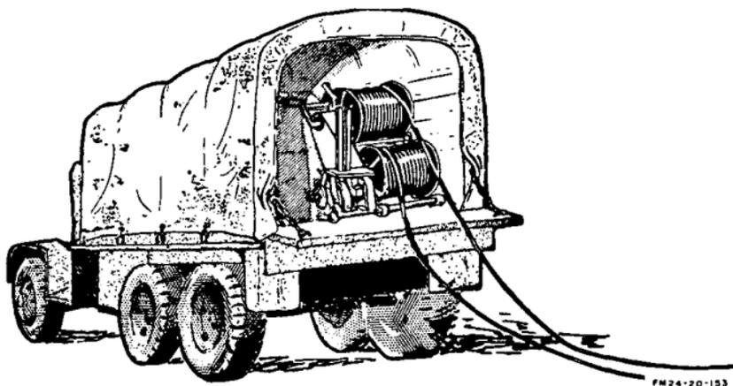
*Figure 92. Laying cable using Reel Unit RL-26-( ).*
