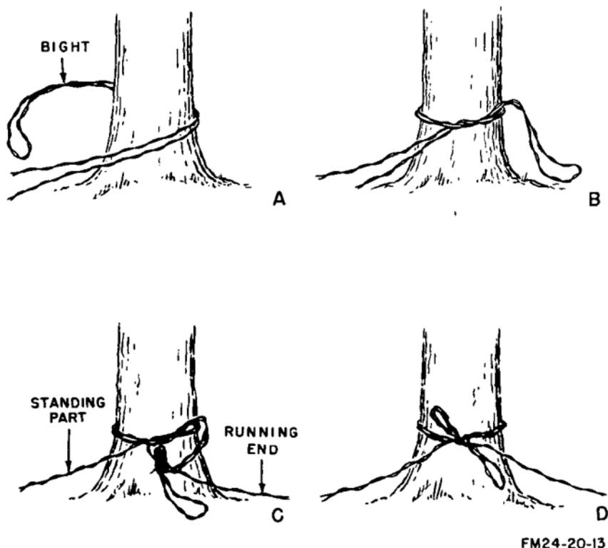
Figure 37. Square knot and loop tie.
