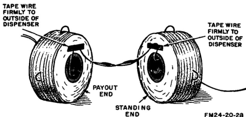
Figure 47. Wire Dispensers MX-306A/G, spliced for tandem operation.
