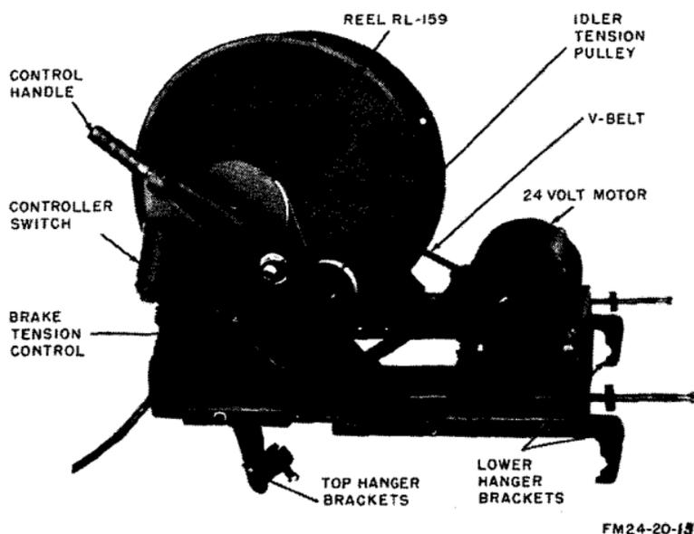
Figure 58. Reeling Machine RL-172( )/G, motor driven.
