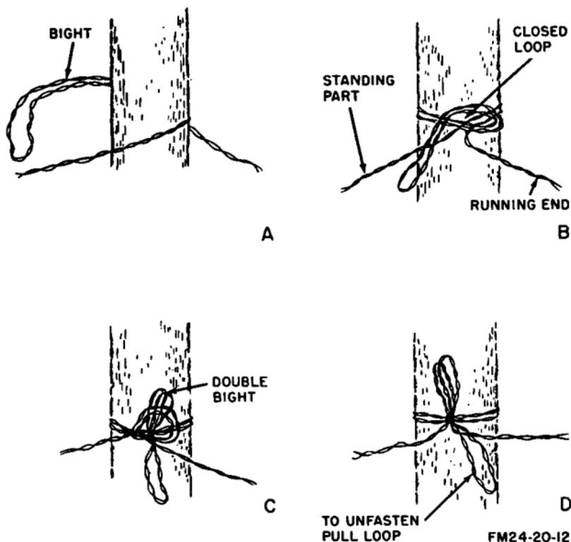
Figure 36. Overhead loop-knot tie.
