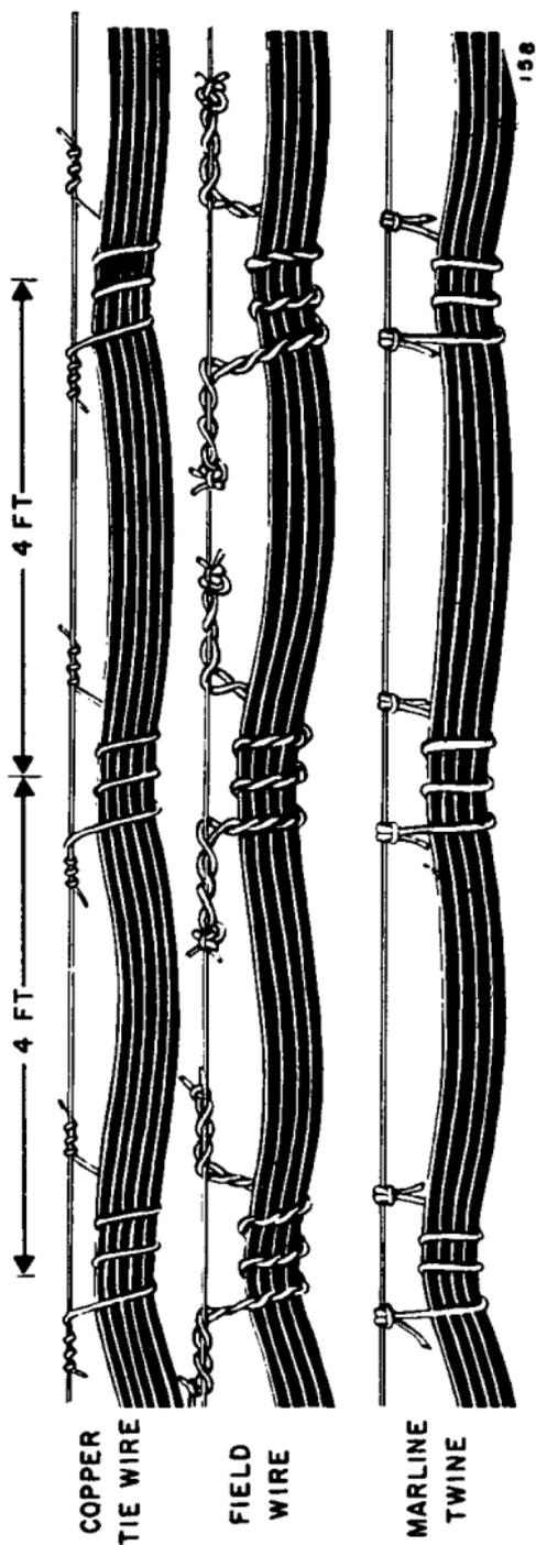
Figure 97. Tying the cables to the support wire.
