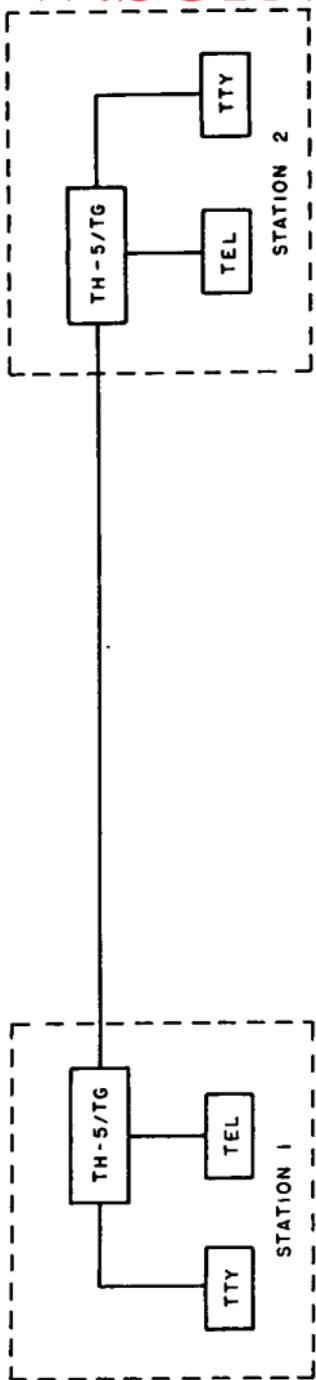
Figure 120. Alternate telegraph-telephone service on point-to-point circuit, using Telegraph Terminal TH-5/TG. FM24-20-97
