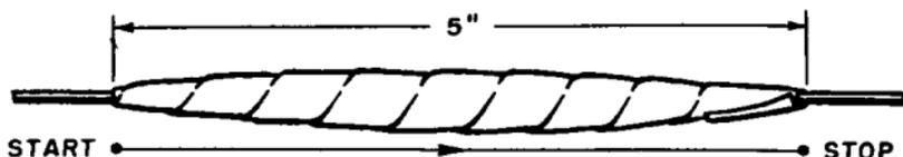
B FRICTION TAPE APPLIED, SHOWING DIRECTION OF WRAPPING.
