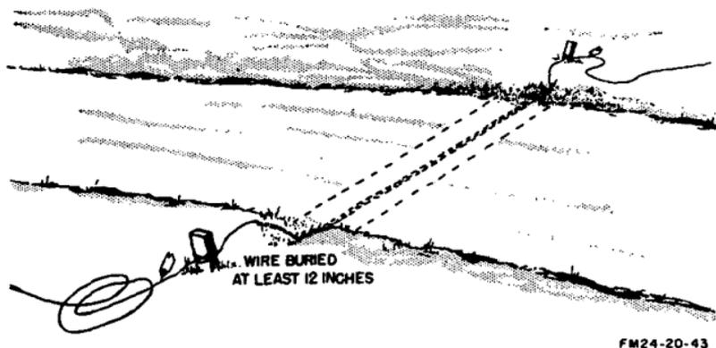
Figure 82. Wire buried in trench to cross roads.
