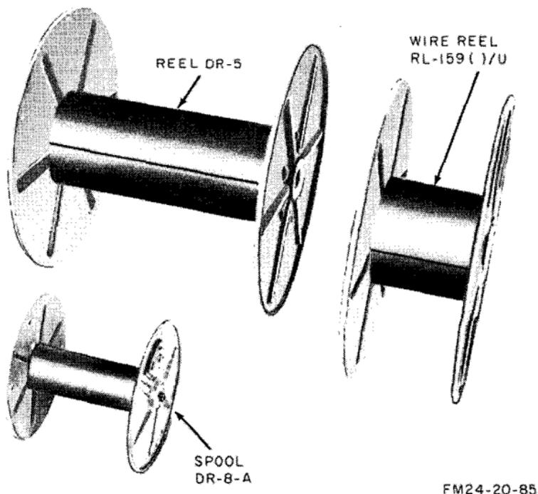
Figure 45. Reels for field wire.
