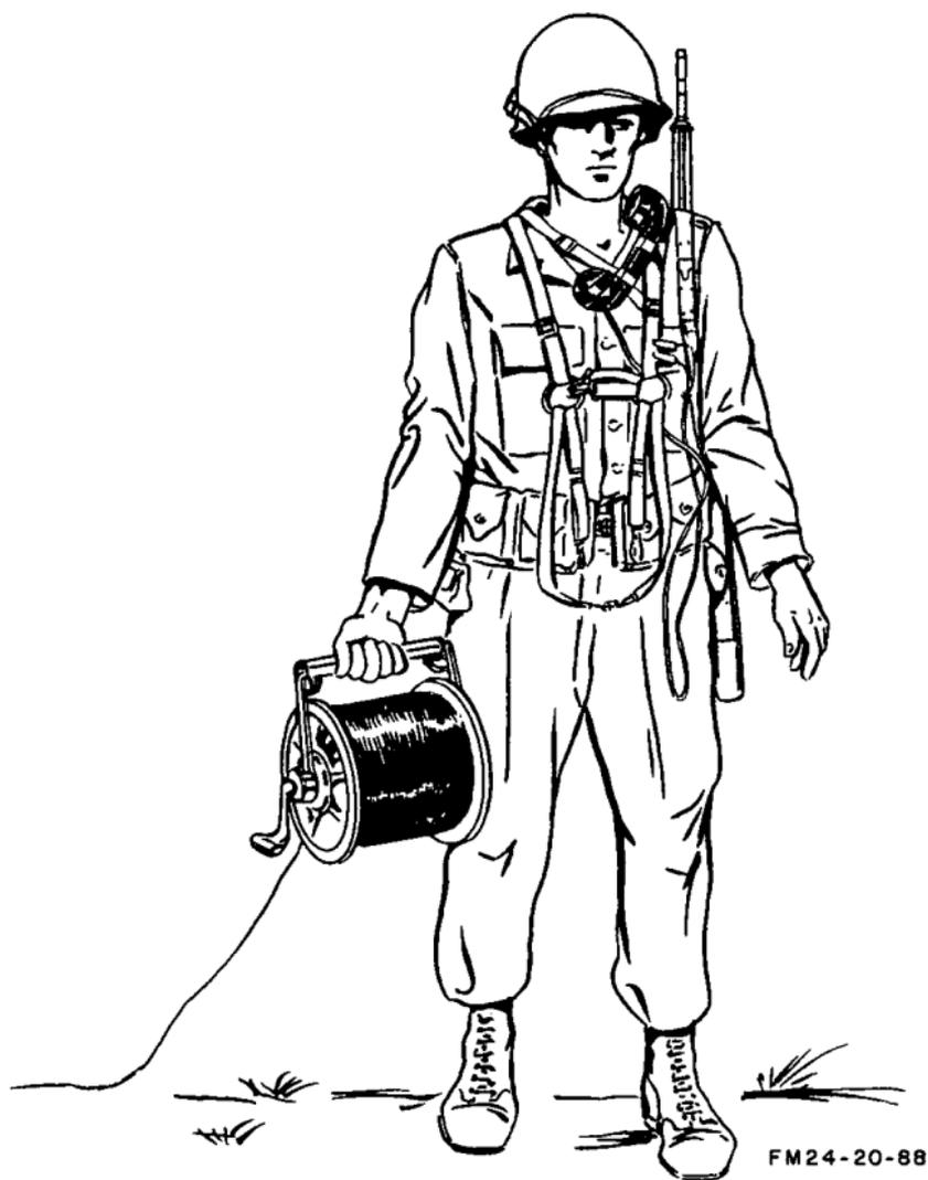
*Figure 56. Laying wire with Reel Equipment CE-11.*
