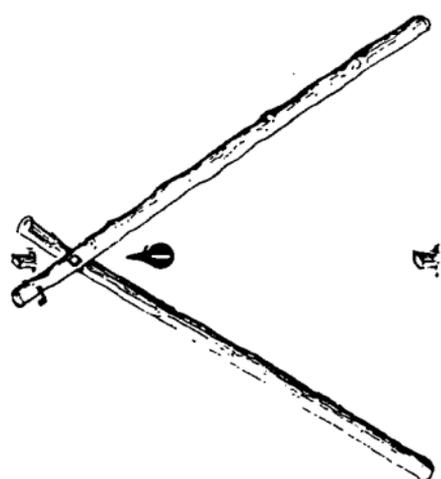
Figure 100. Installing the terminal A-frames.
