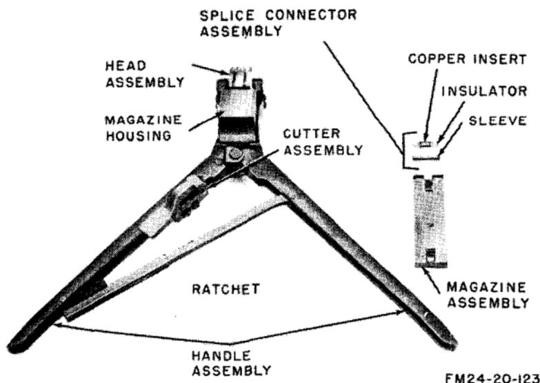
Figure 11. Wire Splicing Tool TL-582( )/U.
