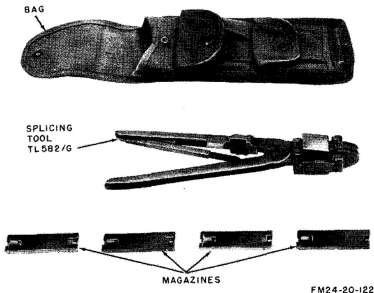
*Figure 10. Wire Splicing Kit MK-356( )/G.*
