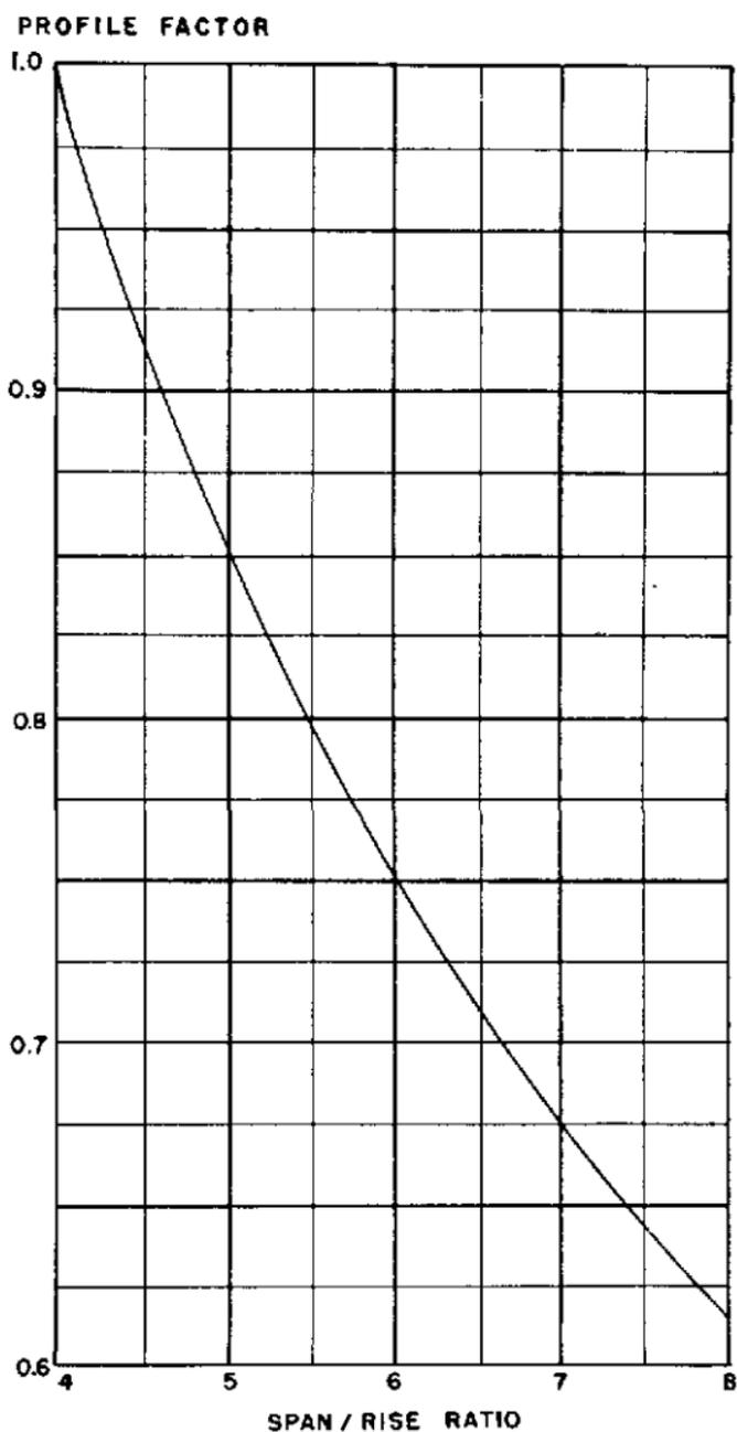
*Figure 113. Profile factors for masonry arch bridges.*
