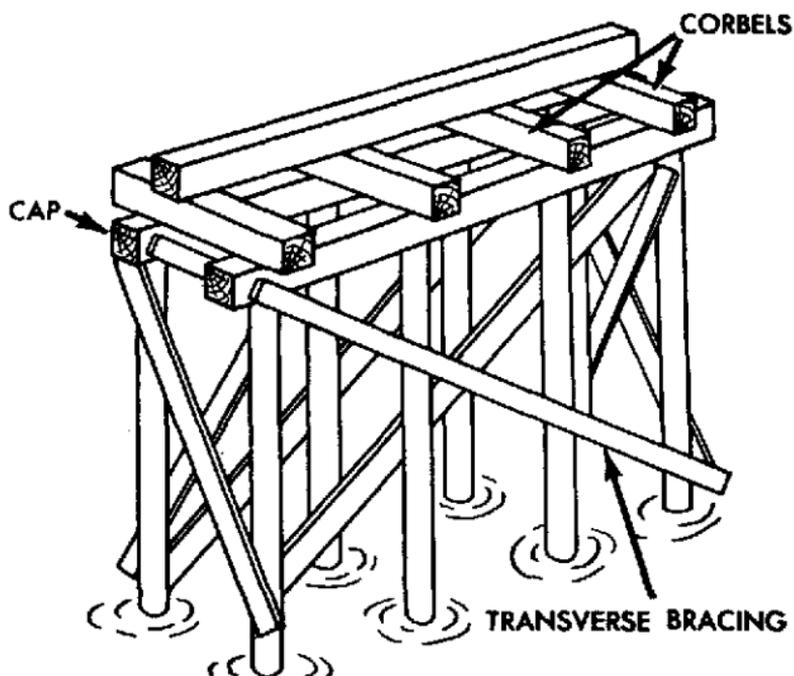
Figure 98. Timber pile pier.
