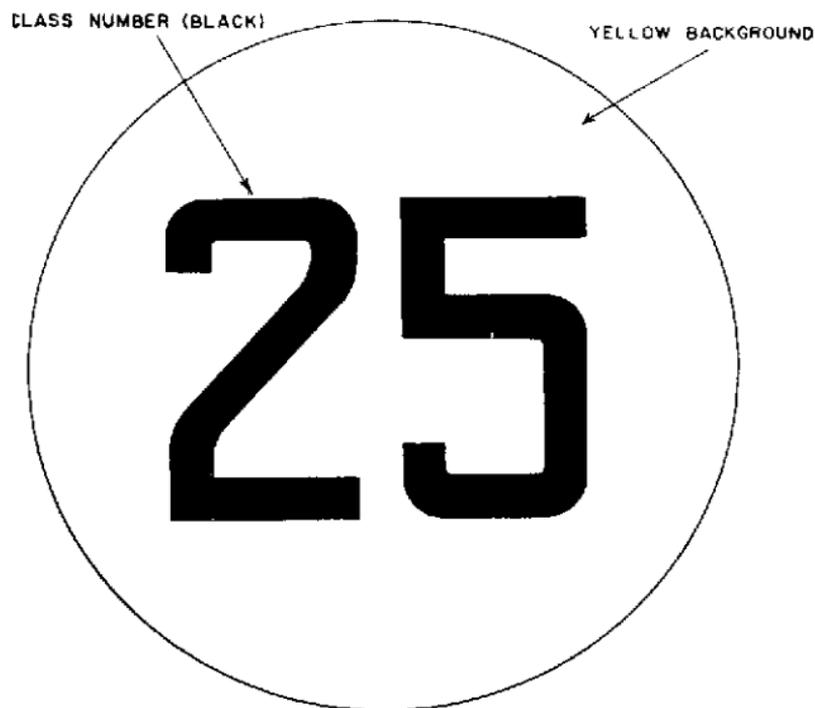
Figure 48. Example of vehicle classification sign.
