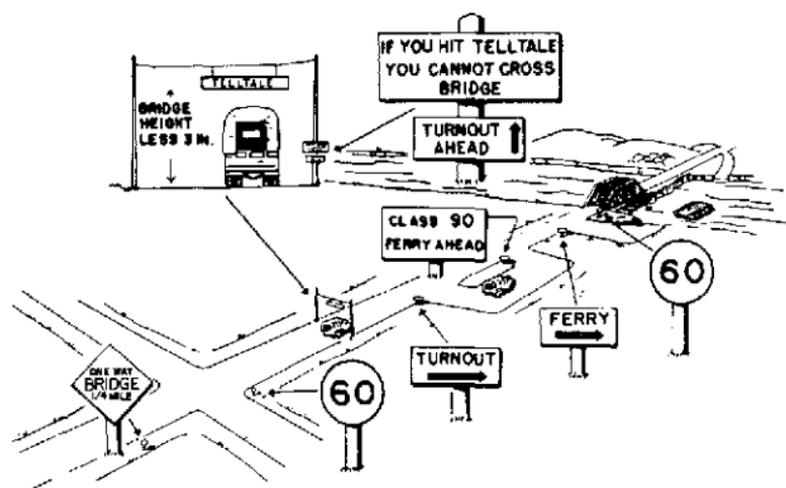
Figure 37. Typical single-lane bridge applications of bridge class and information signs and road guide signs.
