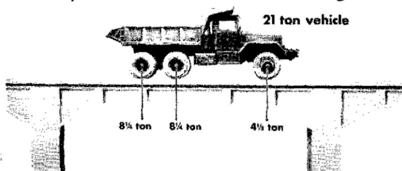
*Figure 25. Effect of vehicle on bridge.*
