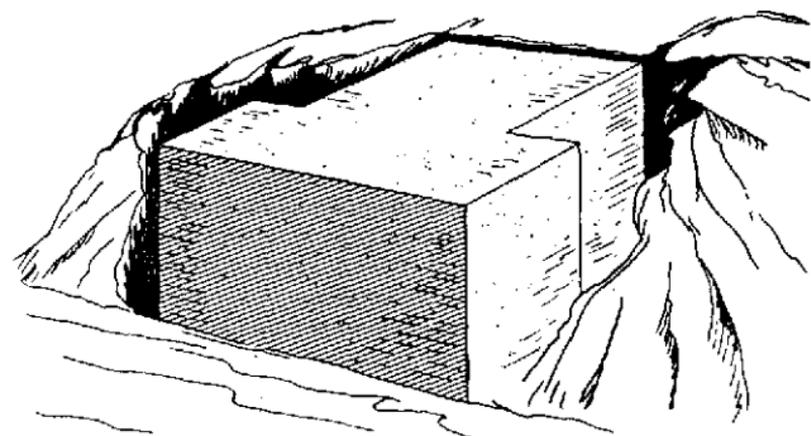
*Figure 106. Typical T-type abutment.*
