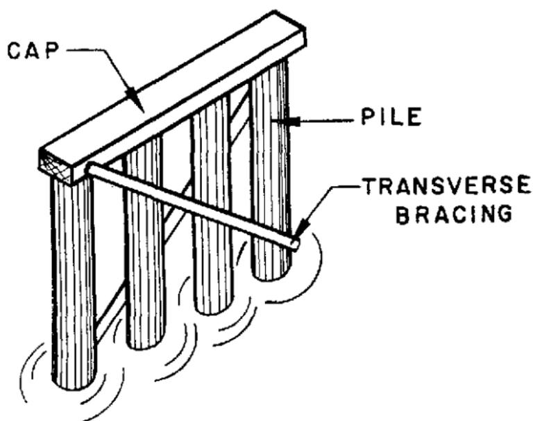
*Figure 94. Pile bent.*
