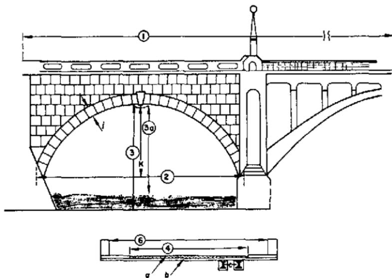
Figure 80. Standard dimension data guide for arch bridges.
