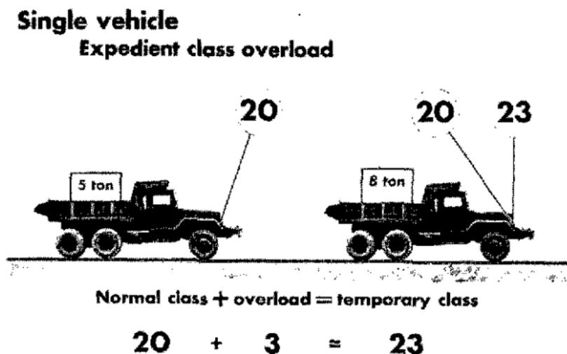
Figure 28. Example of classification of an overload.
