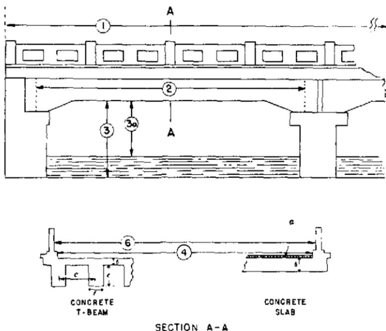
Figure 60. Standard dimension data guide for concrete bridges.
