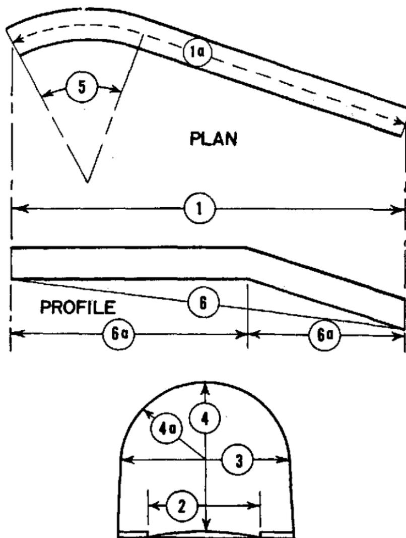
Figure 13. Standard dimensional data for tunnels.
