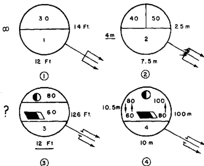
1. This symbol represents a one-way bridge, Class 30, assigned the arbitrary number 1, with an overall length of 14 feet, roadway width of 12 feet, unlimited overhead clearance, and easy bypass conditions.
