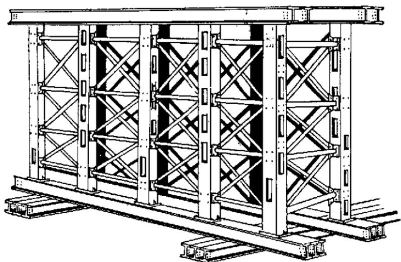
*Figure 101. Typical prefabricated steel trestle pier.*
