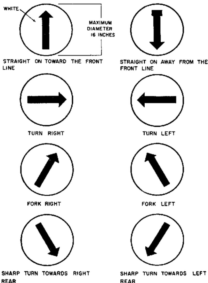
*Figure 46. Examples of directional disks.*
