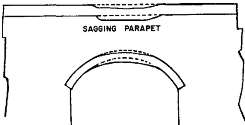
Figure 117. Deformation of arch ring.
