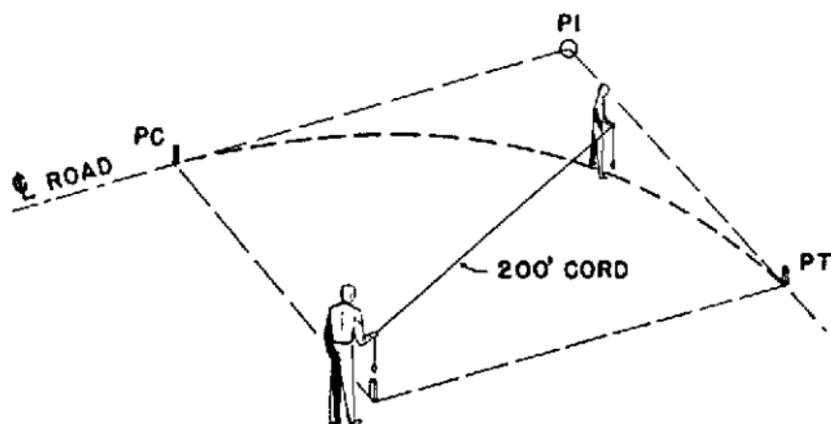
Figure 3. A curve staked by using a cord.
