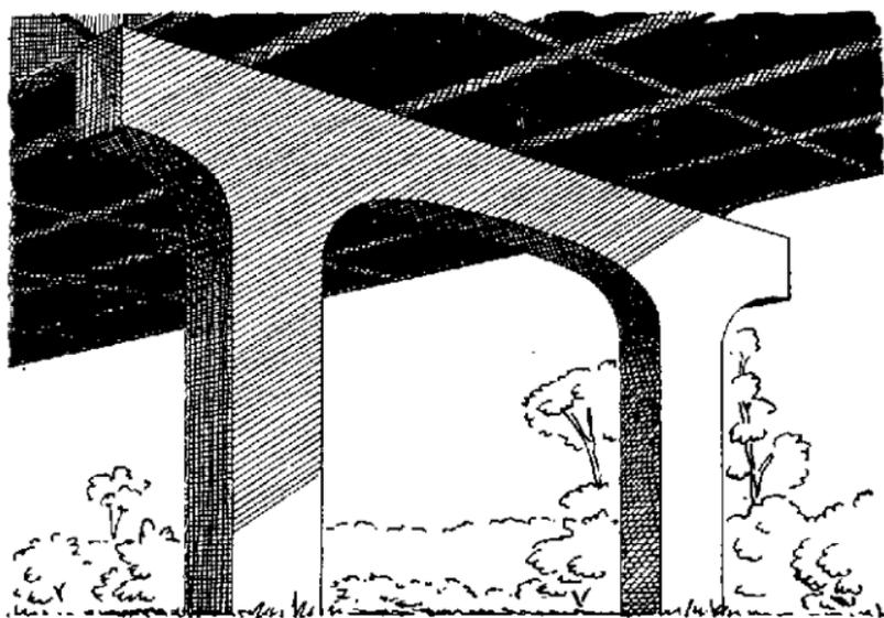
*Figure 102. Typical open type concrete pier.*
