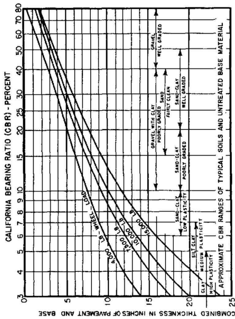
Figure 57. Load-bearing capacity of roads with flexible pavements.
