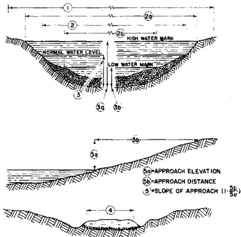
Figure 14. Standard dimensional data for fords.
