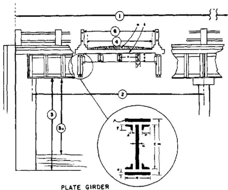
*Figure 77. Standard dimension data for plate girder bridges.*
