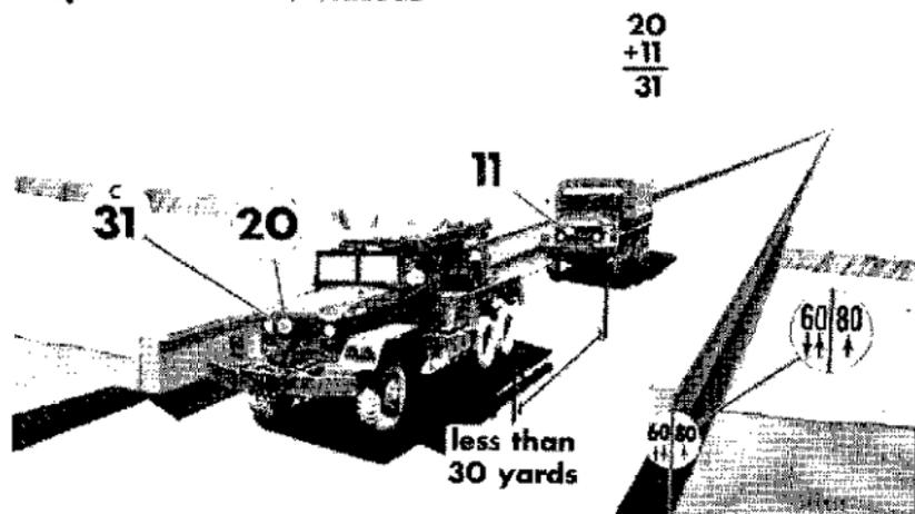
*Figure 27. Nonstandard combination of vehicles.*
