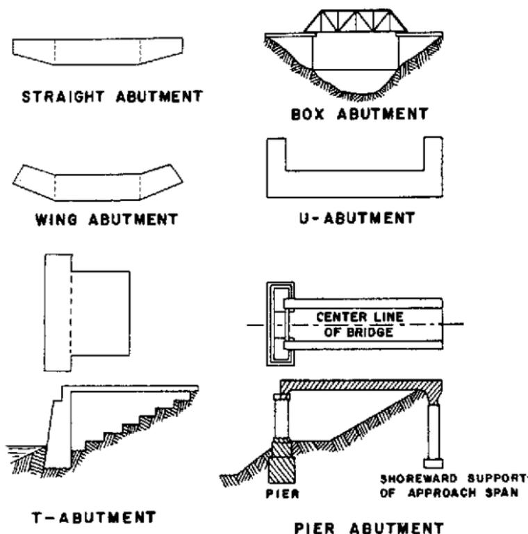
Figure 104. Common types of abutments.
