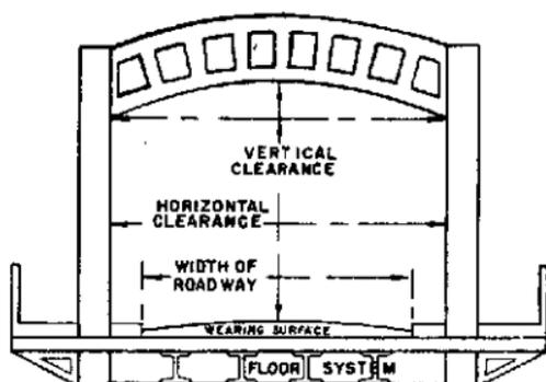
① MEASURING WIDTH OF ROADWAY AND CLEARANCES
