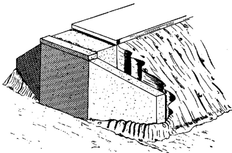
*Figure 108. Typical wing type abutment.*
