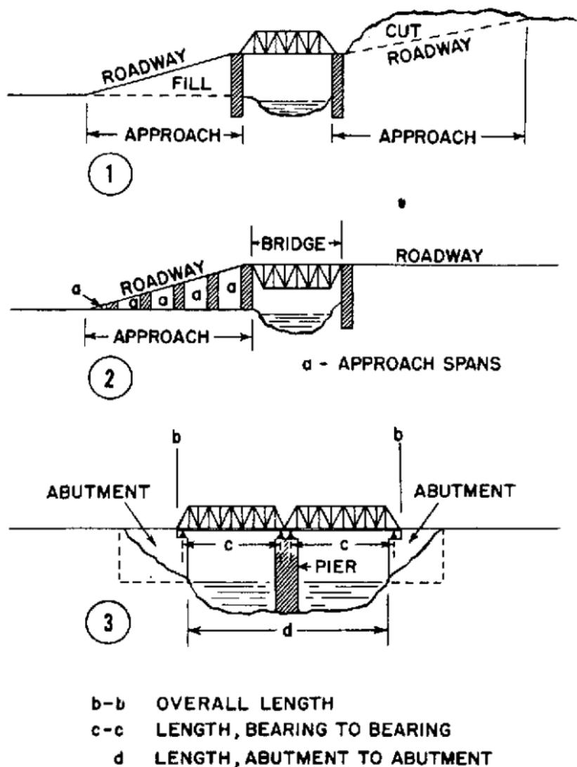
*Figure 7. Typical bridge approaches, abutments, and piers.*
