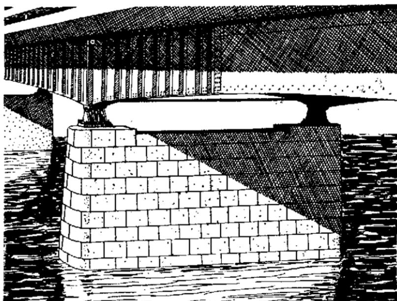
*Figure 100. Typical masonry pier.*
