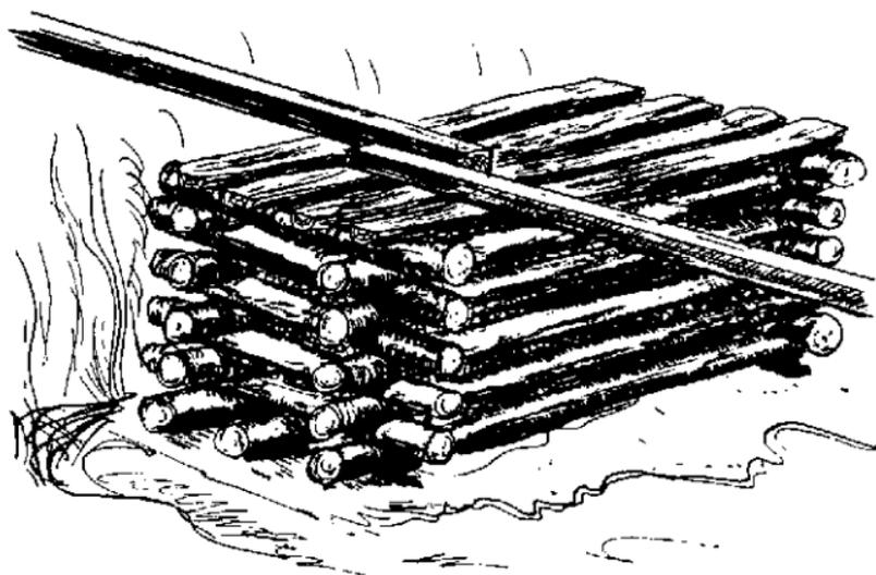
*Figure 99. Typical crib pier.*
