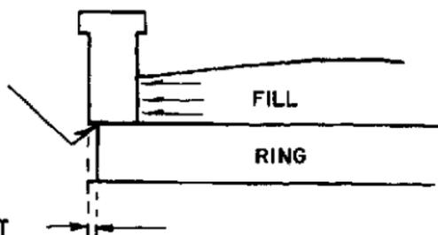
Figure 115. Cracks between arch ring and parapet wall.
