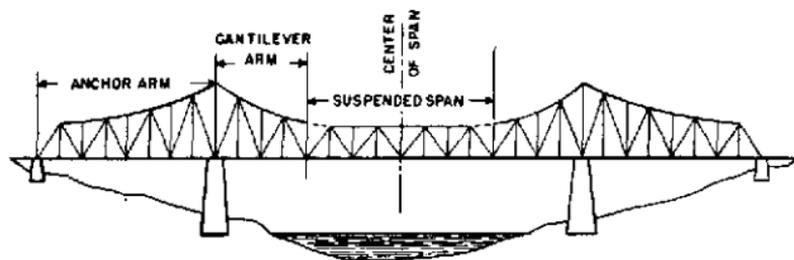
Figure 59. Typical cantilever bridge.
