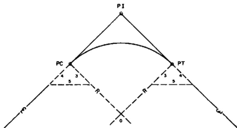
Figure 4. Curve radius by locating center of circle.
