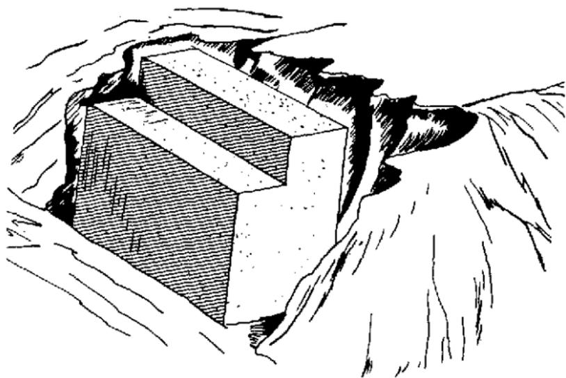
*Figure 105. Typical straight abutment.*
