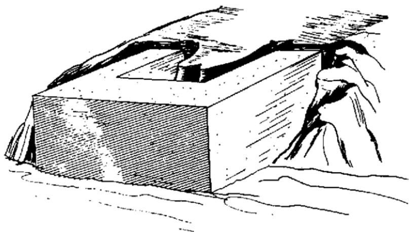
*Figure 107. Typical U-type abutment.*
