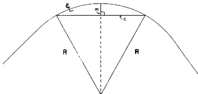
Figure 5. Measuring a curve using formula
