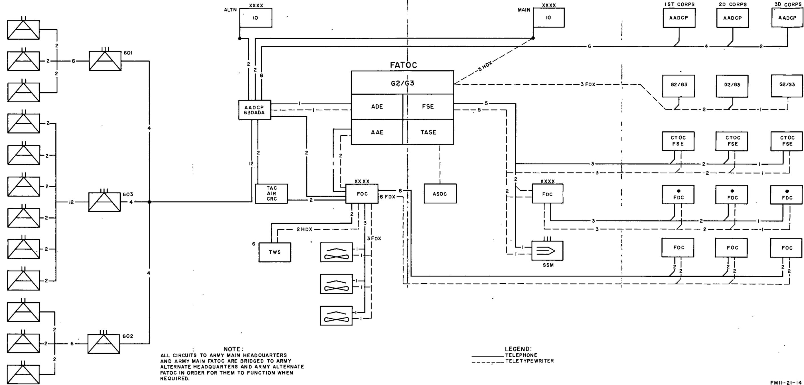
Figure 17. Type army sole-user telephone and teletypewriter traffic diagram.
