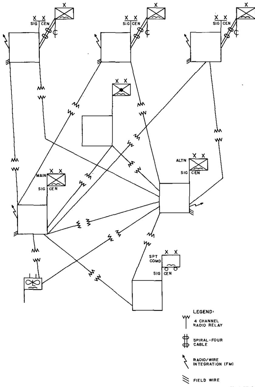
Figure 8. Type Airborne Division Multichannel Communication Network.
