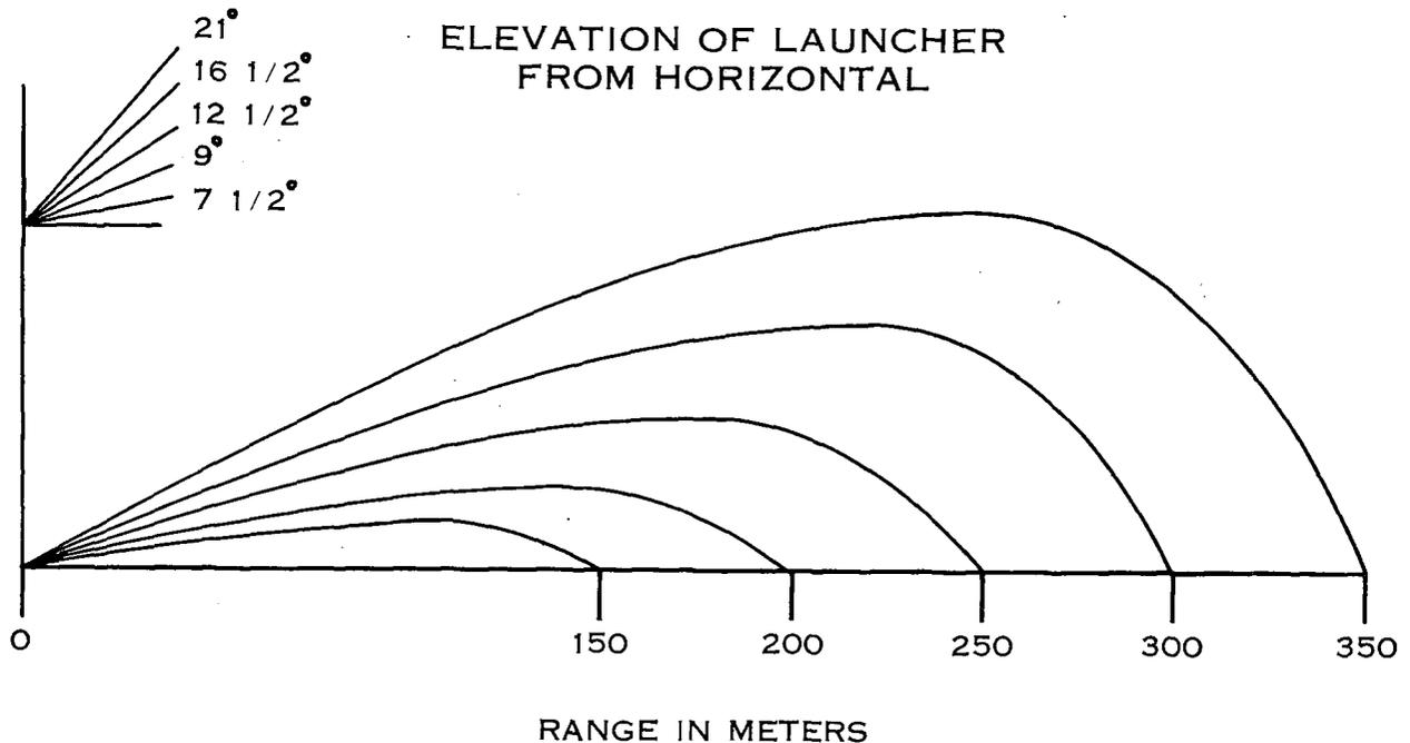
Figure 5. Trajectory of 40-mm grenade launcher ammunition.
