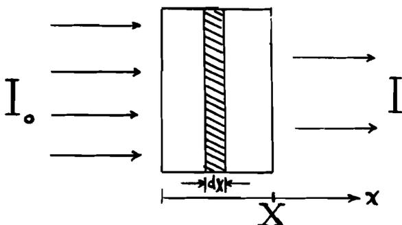
Fig. 4-4 Particles entering a slab of material.
