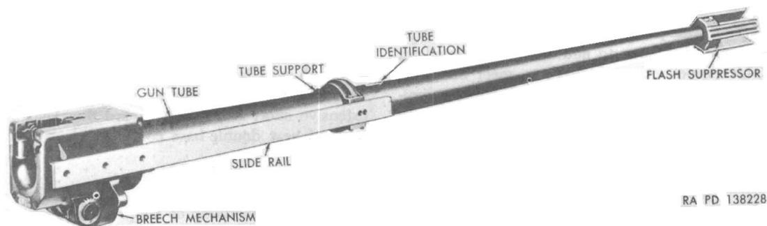
Fig. 3-15 Flash suppressor on 75-mm gun tube.
