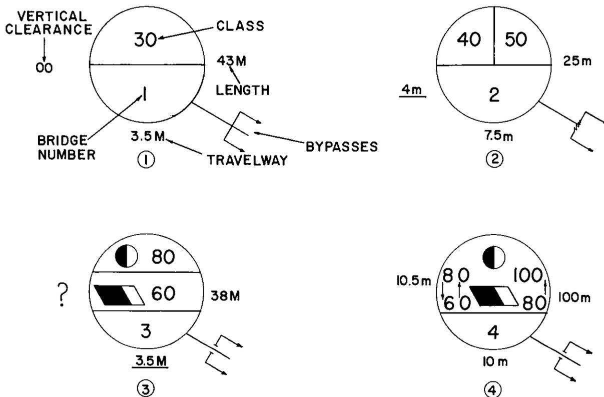
Figure 185. Examples of the full bridge symbol for use on a map or overlay.
