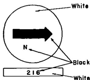
Figure 84. Example of alternate lateral route signs.
