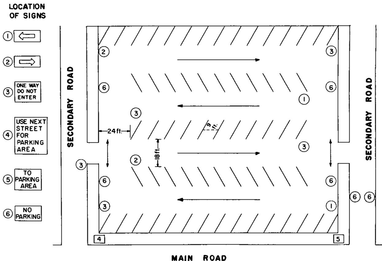
Figure 36. Example of a temporary parking facility with a turnover using alternating one-way aisles.
