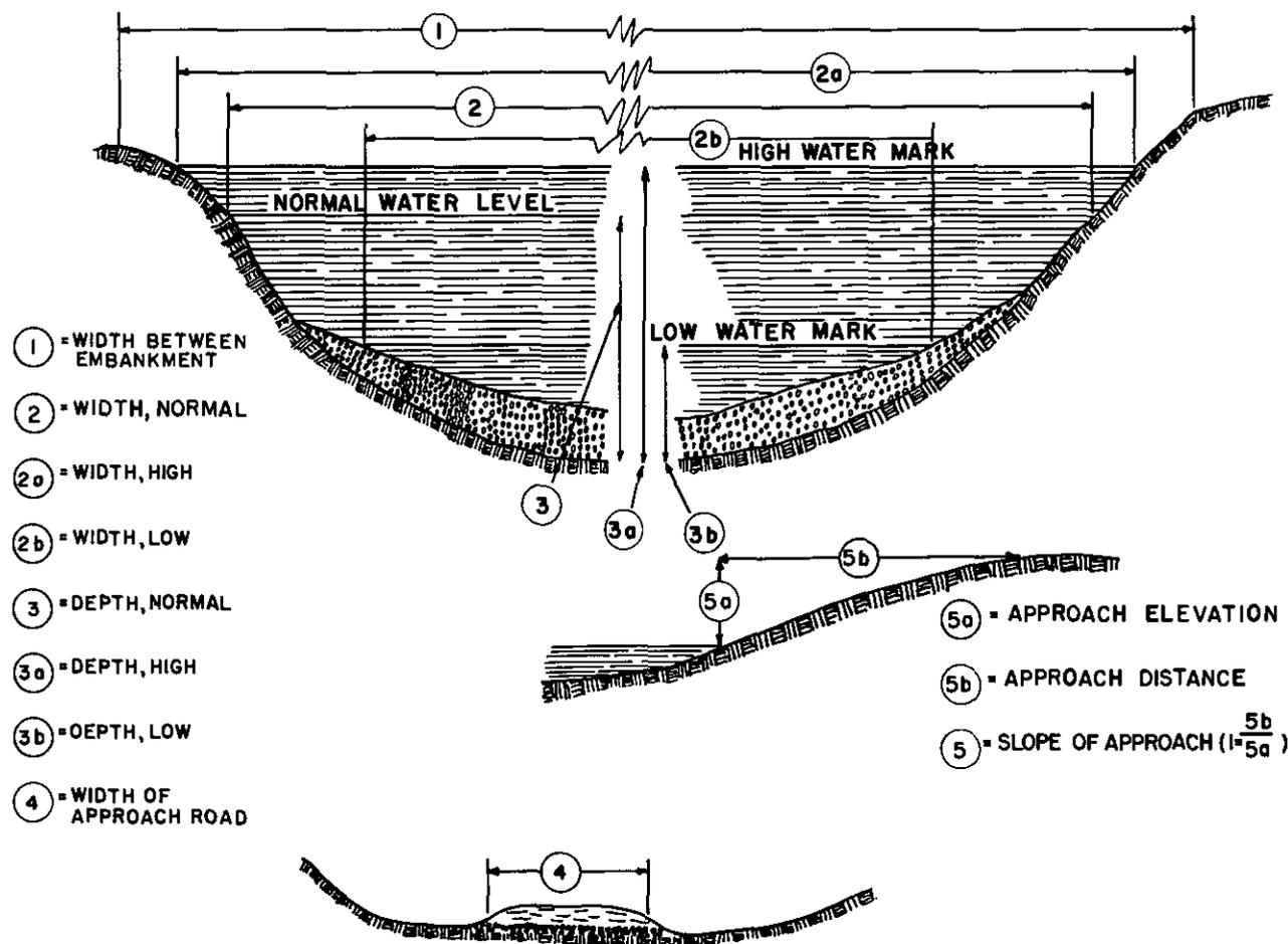
Figure 133. Standard dimensional data for fords.
