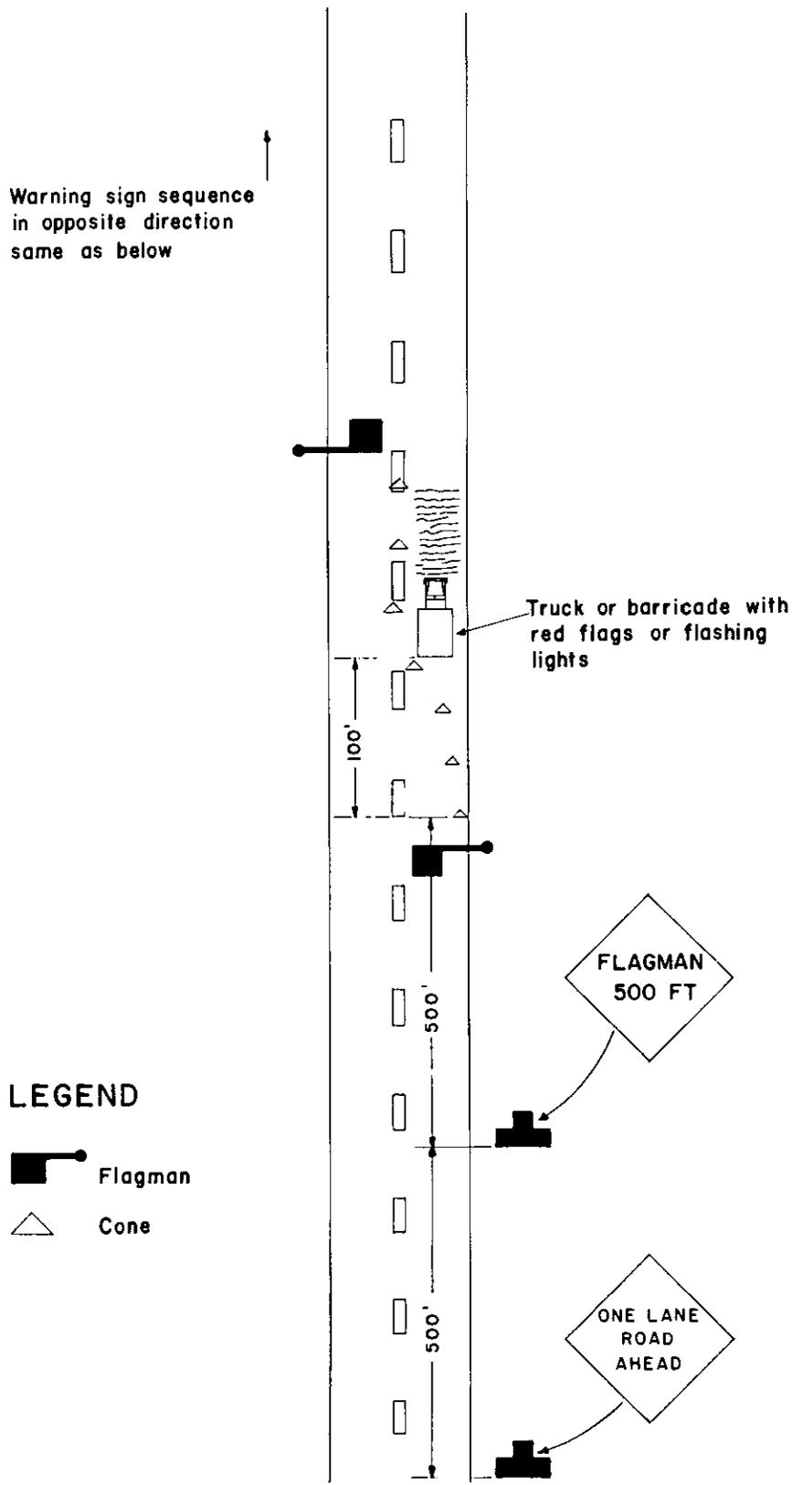
Figure 41. Example of one lane closed road using a flagman.
