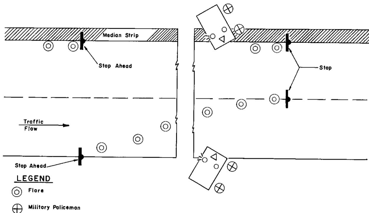
Figure 49. Example of a multilane road roadblock.
