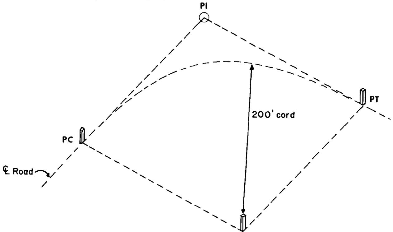
Figure 120. A curve staked by using a cord.
