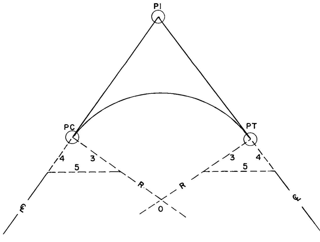
Figure 121. Curve radius by locating center of circle.
