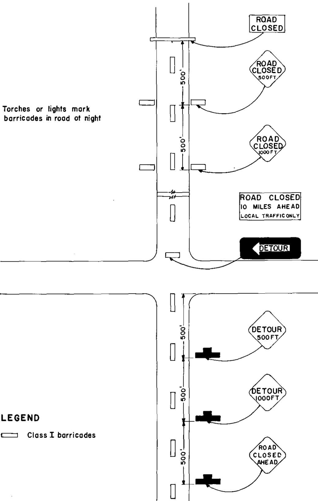
Figure 40. Example of signing for a closed road.
