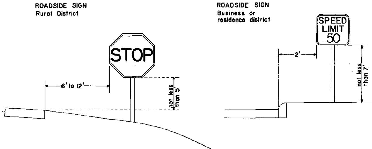
Figure 38. Examples of erection of temporary signs.
