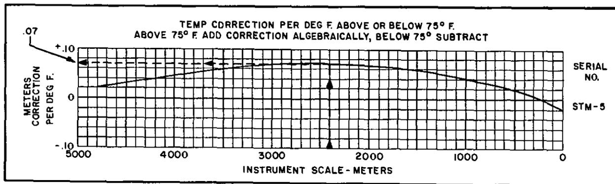
Figure 93. Instrument temperature correction chart.
