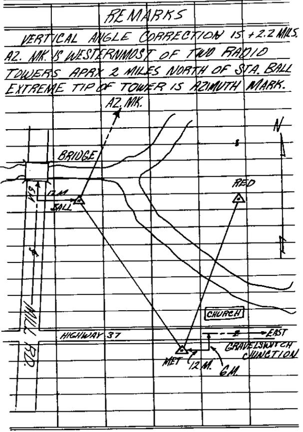
Figure 67. Recorder's notes for aiming circle triangulation.
