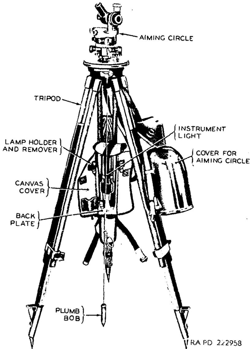
Figure 29. Aiming circle with accessory equipment.
