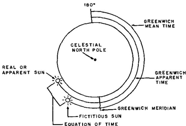
Figure 114. Apparent solar time.
