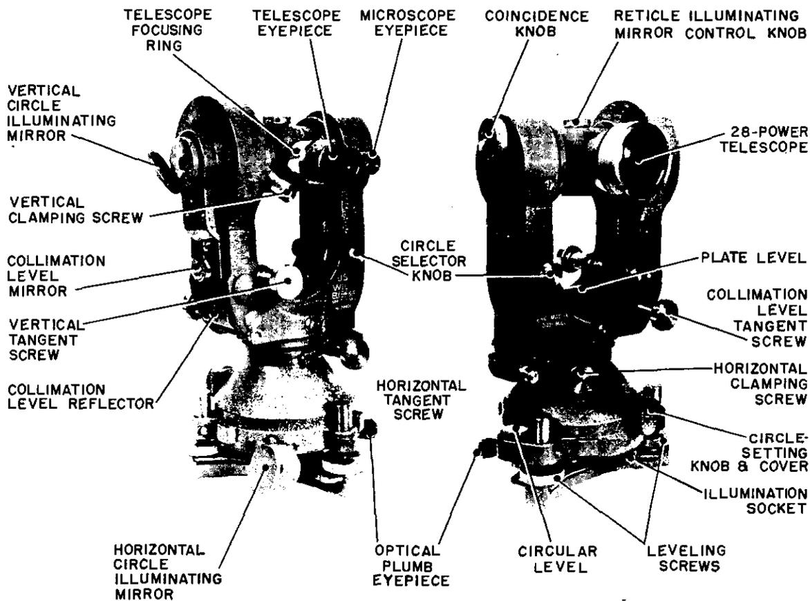
Figure 38. The T2 theodolite.
