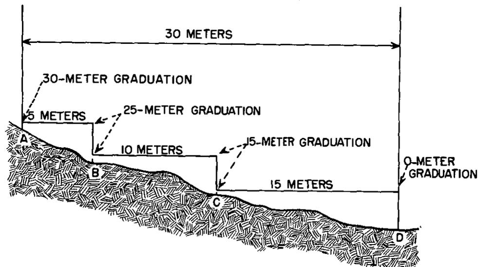
Figure 12. Breaking tape.
