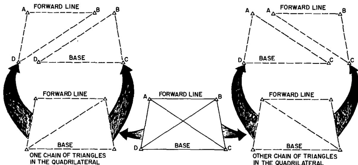
Figure 77. A quadrilateral separated into two single chains of two triangles each.
