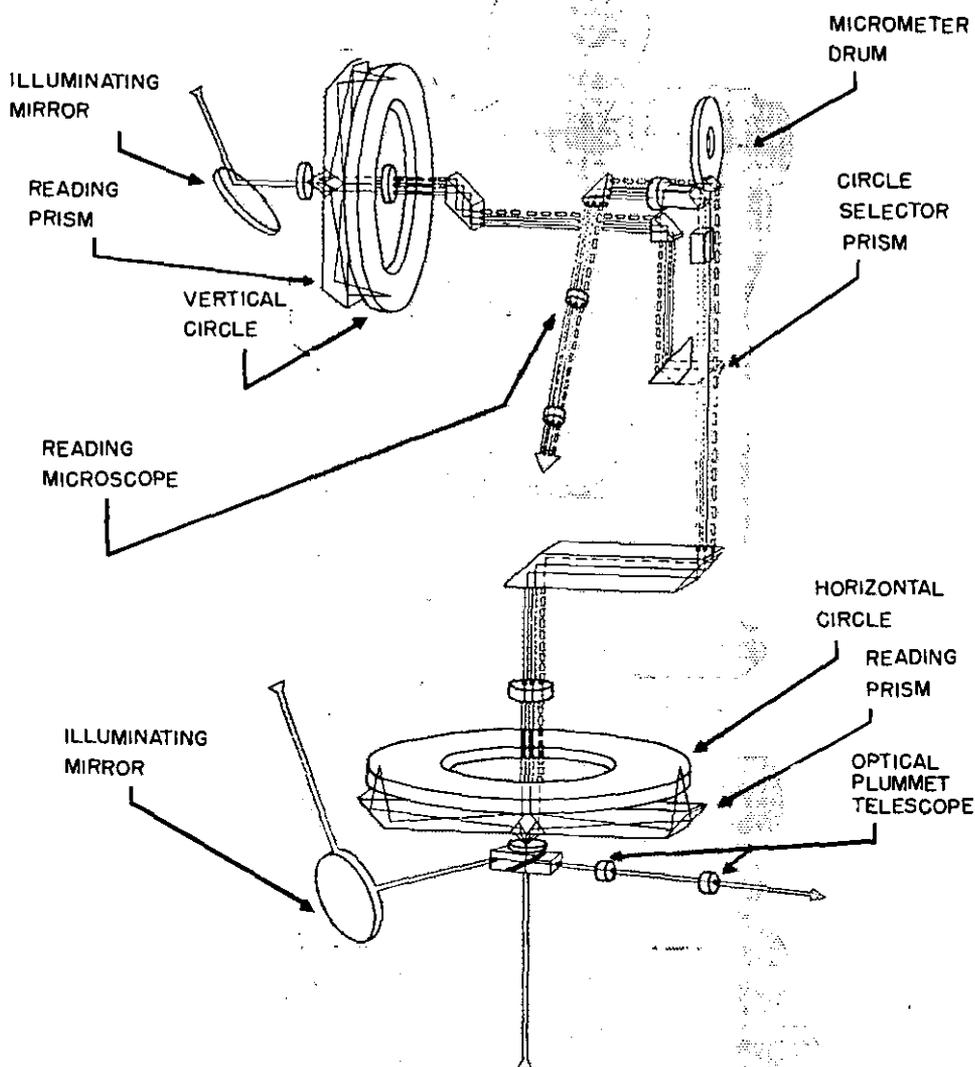
Figure 39. Circle-reading optical system of the T2 theodolite.
