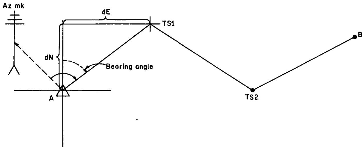
Figure 52. Requirements for  $dE$  and  $dN$ .
