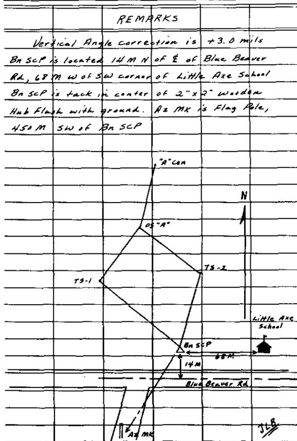
Figure 47. Recorder's notes for 1:500 (aiming circle) traverse.
