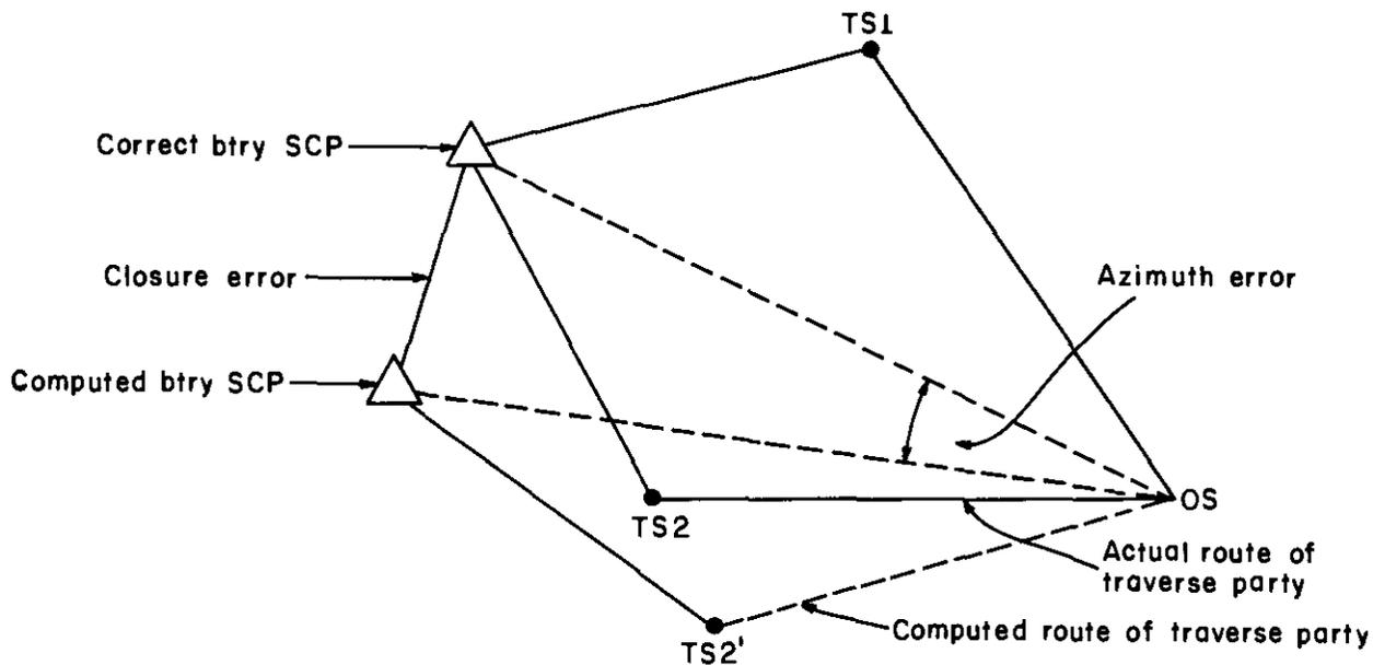
Figure 63. Azimuth error.
