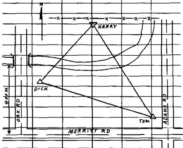
Figure 68. Recorder's notes for fifth-order, T16 theodolite, triangulation.
