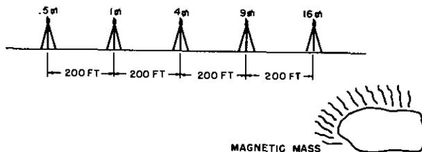
Figure 104. Detecting hidden magnetic disturbance.
