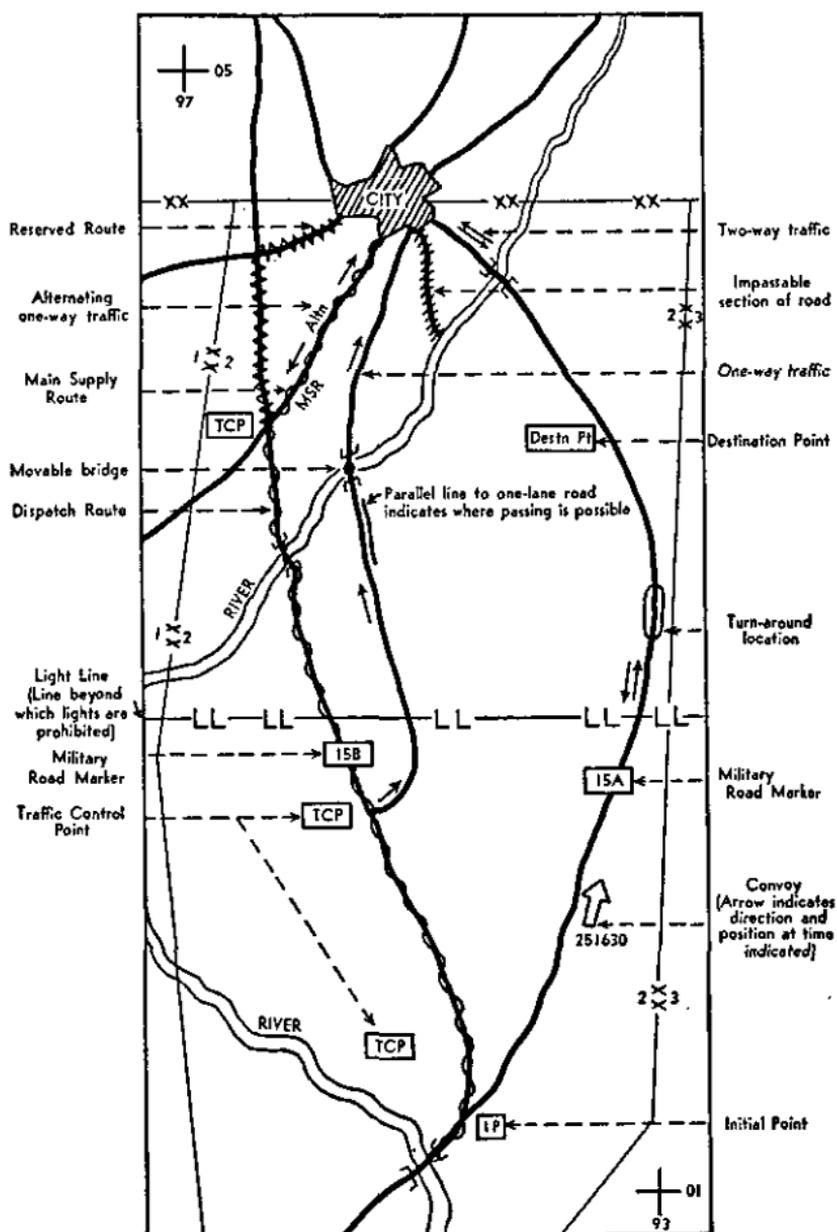
Figure 18. Traffic circulation overlay.
