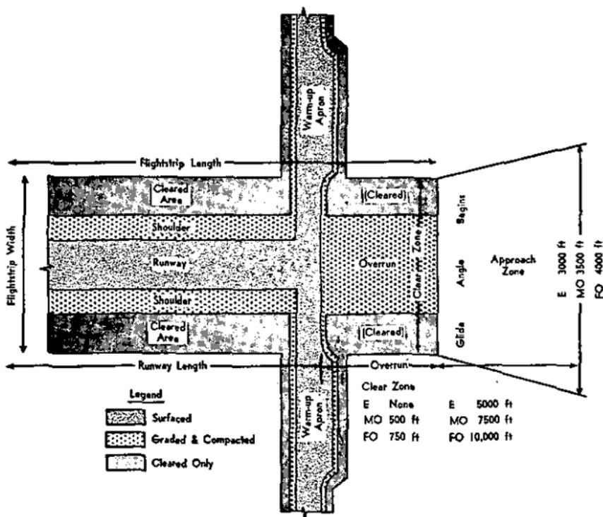
Figure 21. Elements of a flightway.
