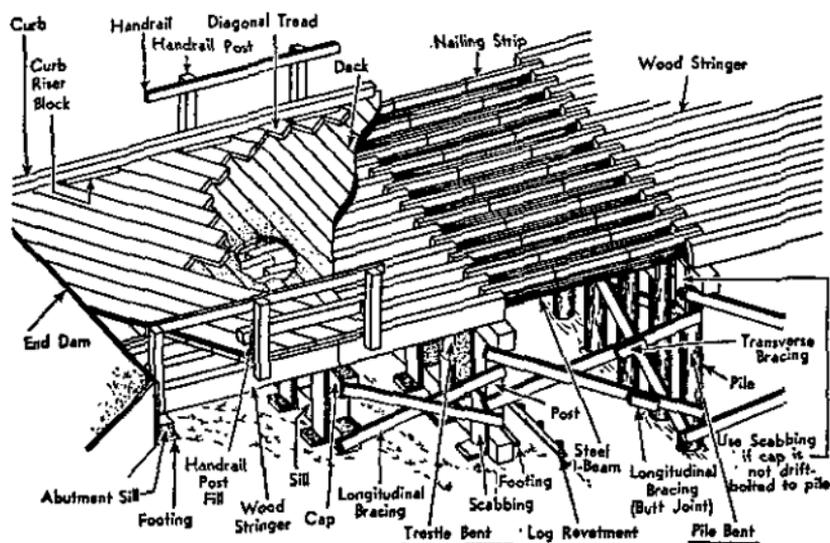
Figure 20. Elements of a timber trestle bridge.
