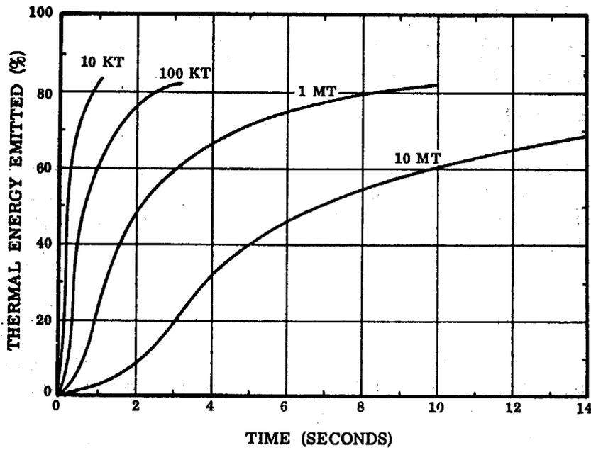
Figure 7.95. Percentage of thermal energy emitted as a function of time for air bursts of various yields.
