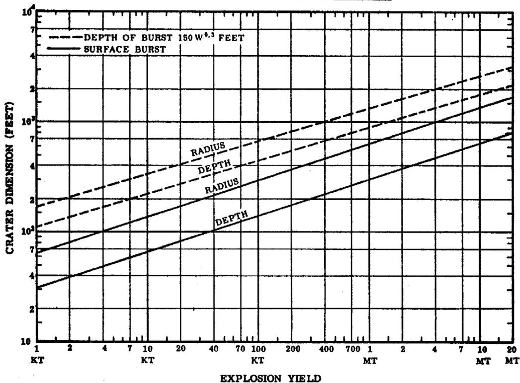
Figure 6.48. Apparent crater dimensions for bursts at the surface and at a depth of 150 W<sup>0.3</sup> feet in dry soil.
