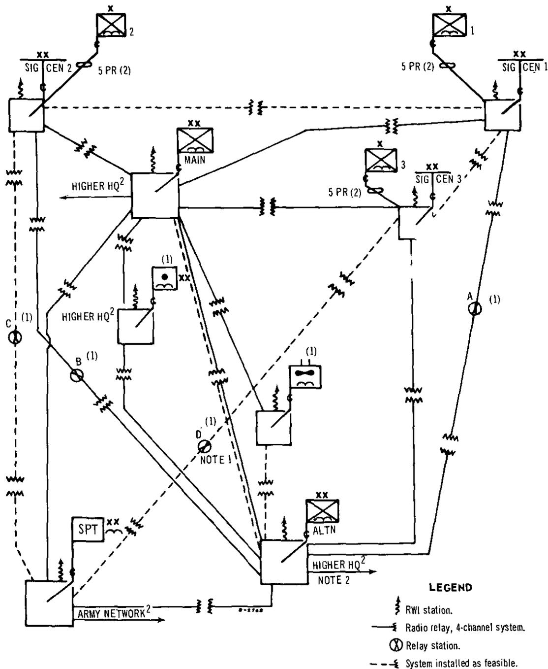
Figure 4-10. Type multichannel networks, airborne division.
