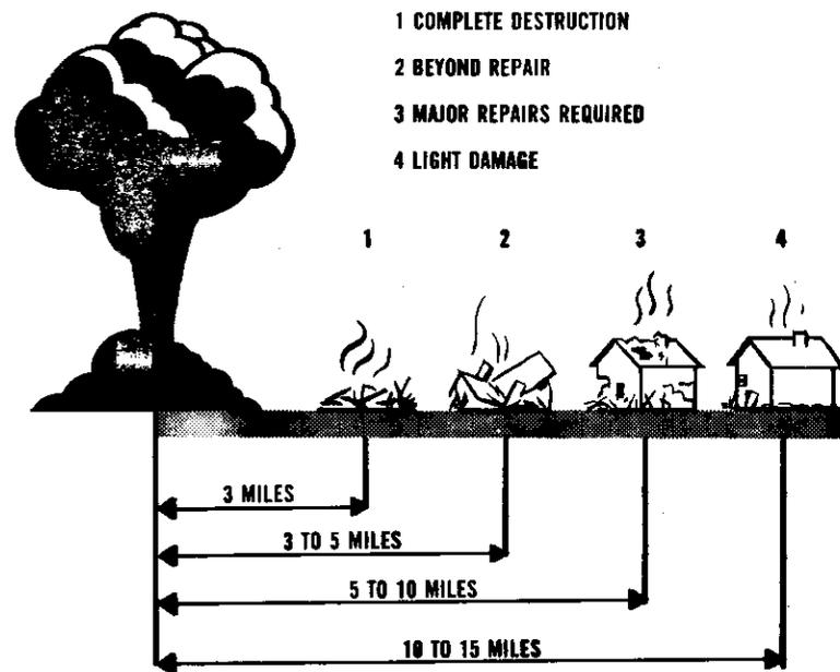
The kinds of damage that the blast can do to buildings are:
