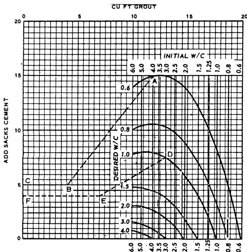
Figure 6. Portland-cement grout thickening chart
