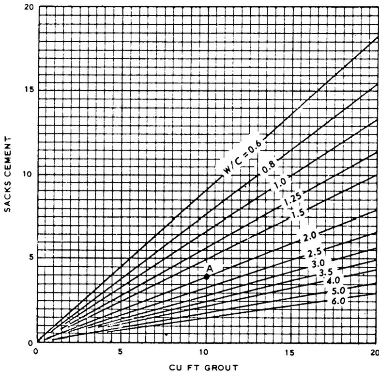
Figure 5. Cement content of portland-cement grout mixes
