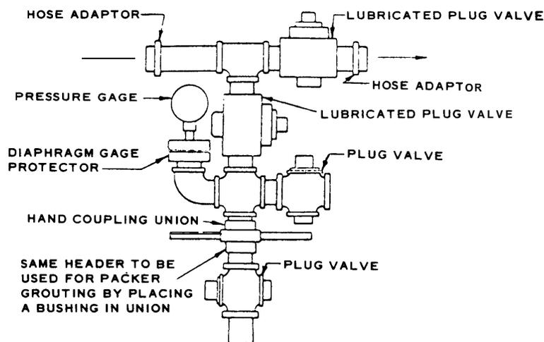
NOTE: ALL PIPE AND FITTINGS ARE 1-1/2" SIZE. PLUG VALVES TO BE USED THROUGHOUT FOR PRESSURES ABOVE 250 PSI. GROUT HOSE TO BE 1-1/2" WITH SCREW-TYPE COUPLINGS.
