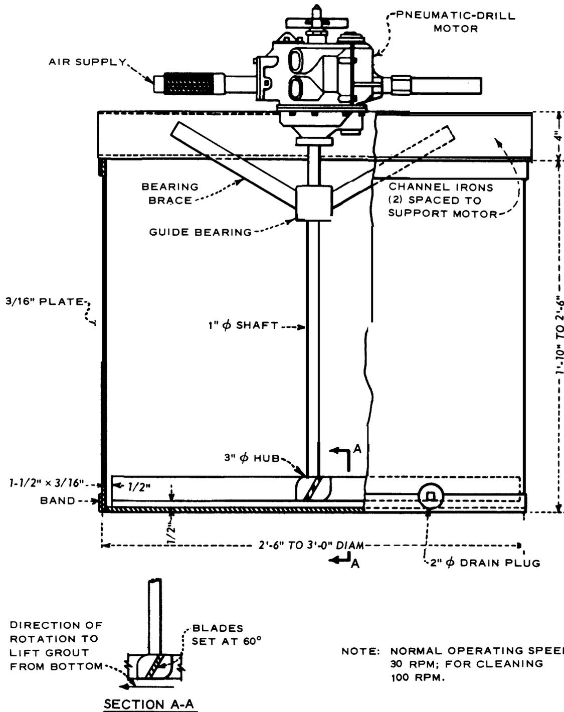
Figure 12. Grout agitator
