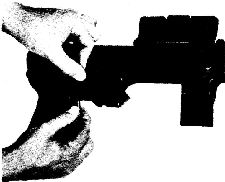
*Figure 16. Replace the trigger and sear group in the receiver, with the trigger pin holes in the trigger and receiver aligned. Replace the trigger pin. The front arm of the trigger pin goes through the holes in the receiver and does not go through any other parts.*
