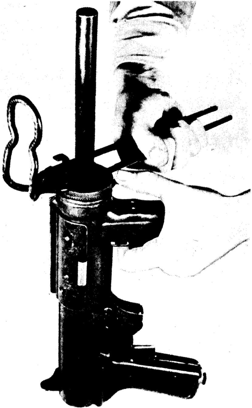
*Figure 10. Using MSA1 stock as a wrench.*
