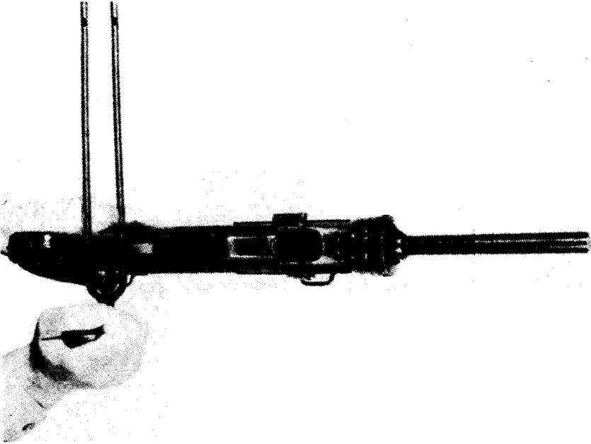
*Figure 18. Use of the stock in replacing the trigger guard.*
