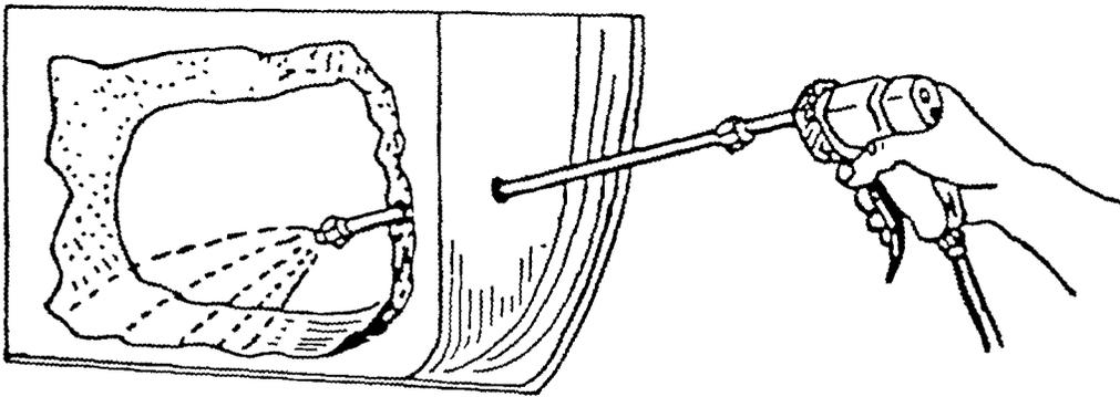
FIGURE 5 Spraying inside of door.
