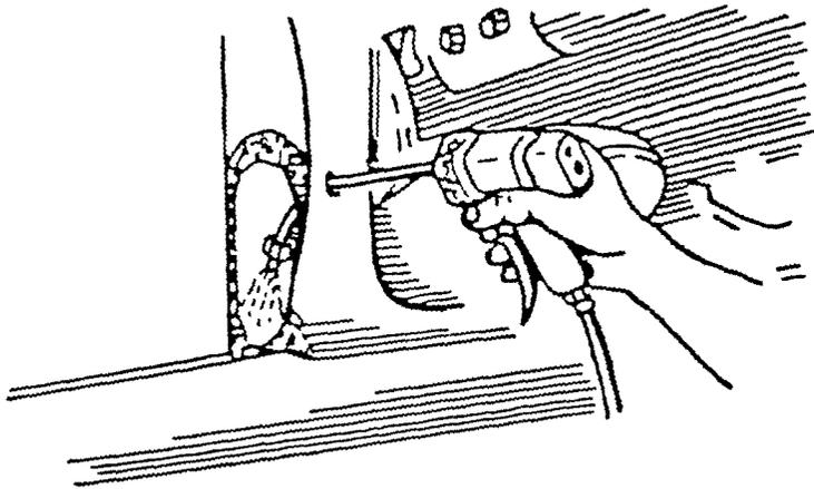
FIGURE 4 Spraying inside of center door post
