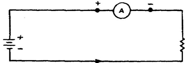
**B. AMMETER CONNECTED IN SERIES**
