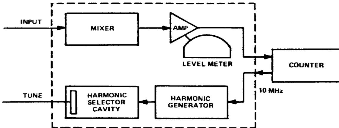
Figure 3-10. Electronic counter heterodyne method, block diagram
