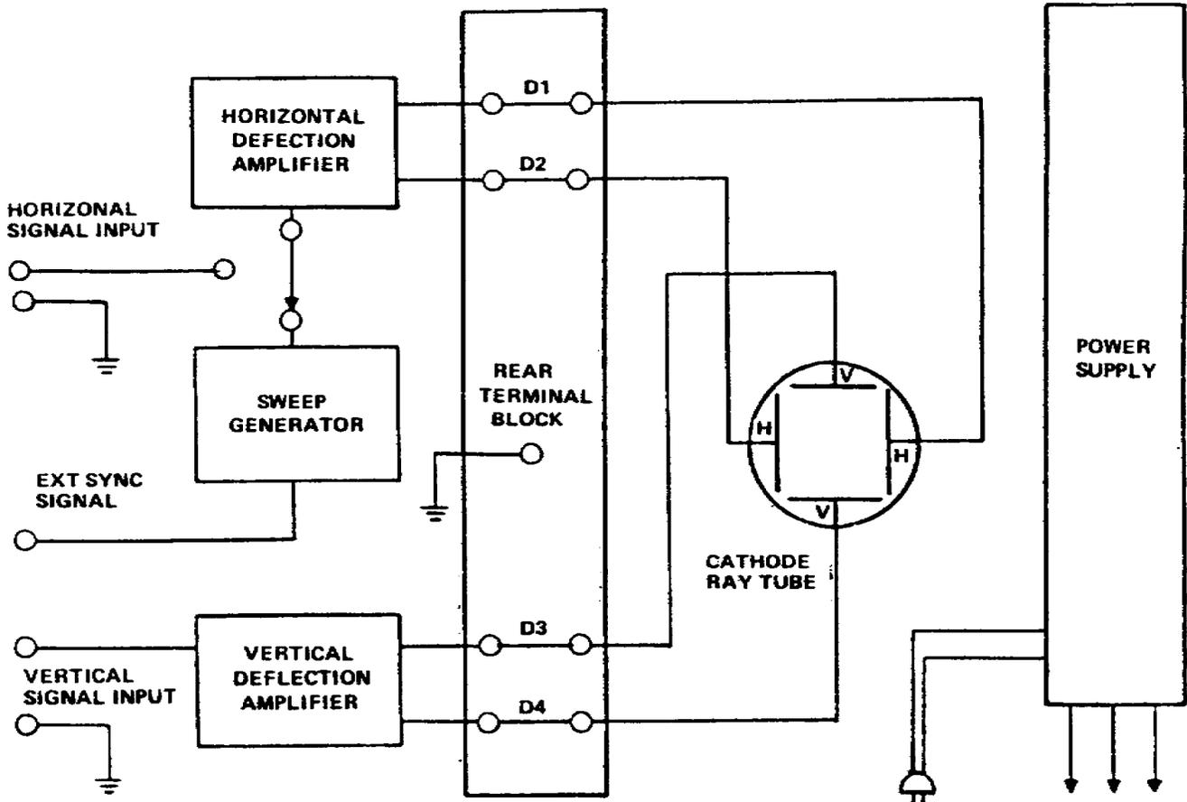
Figure 2-2. Block diagram of a typical cathode-ray oscilloscope
