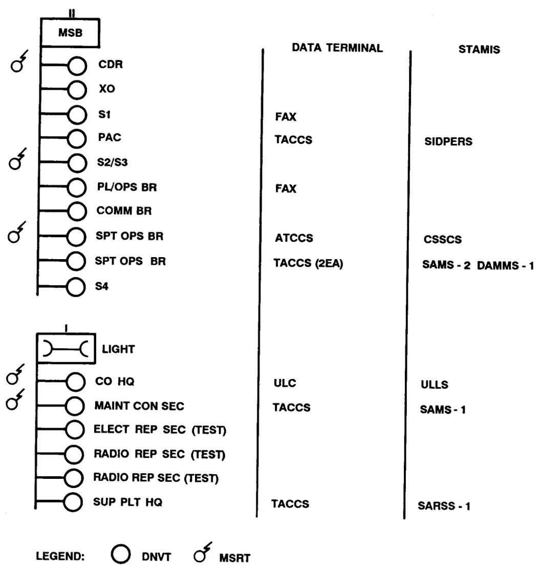
Figure 3-16 MSB Subscriber Terminal Assignments (Fixed and Mobile)
