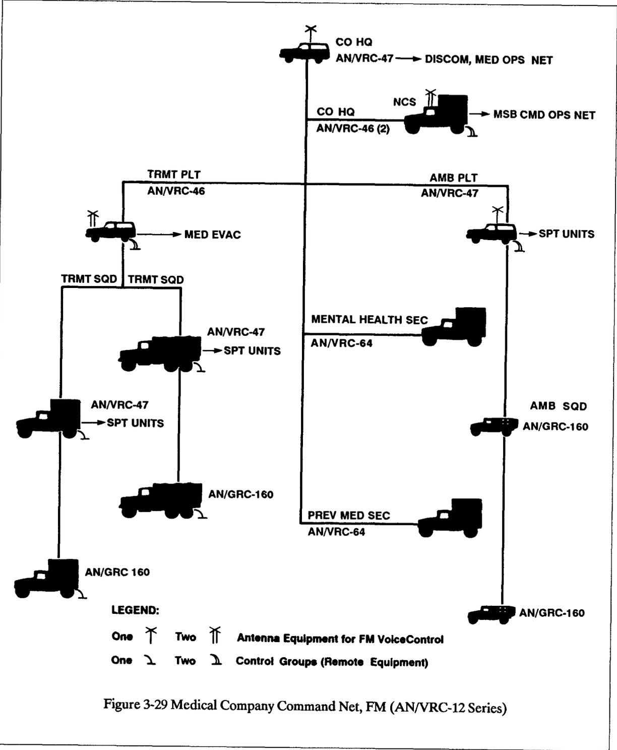
Figure 3-29 Medical Company Command Net, FM (AN/VRC-12 Series)
