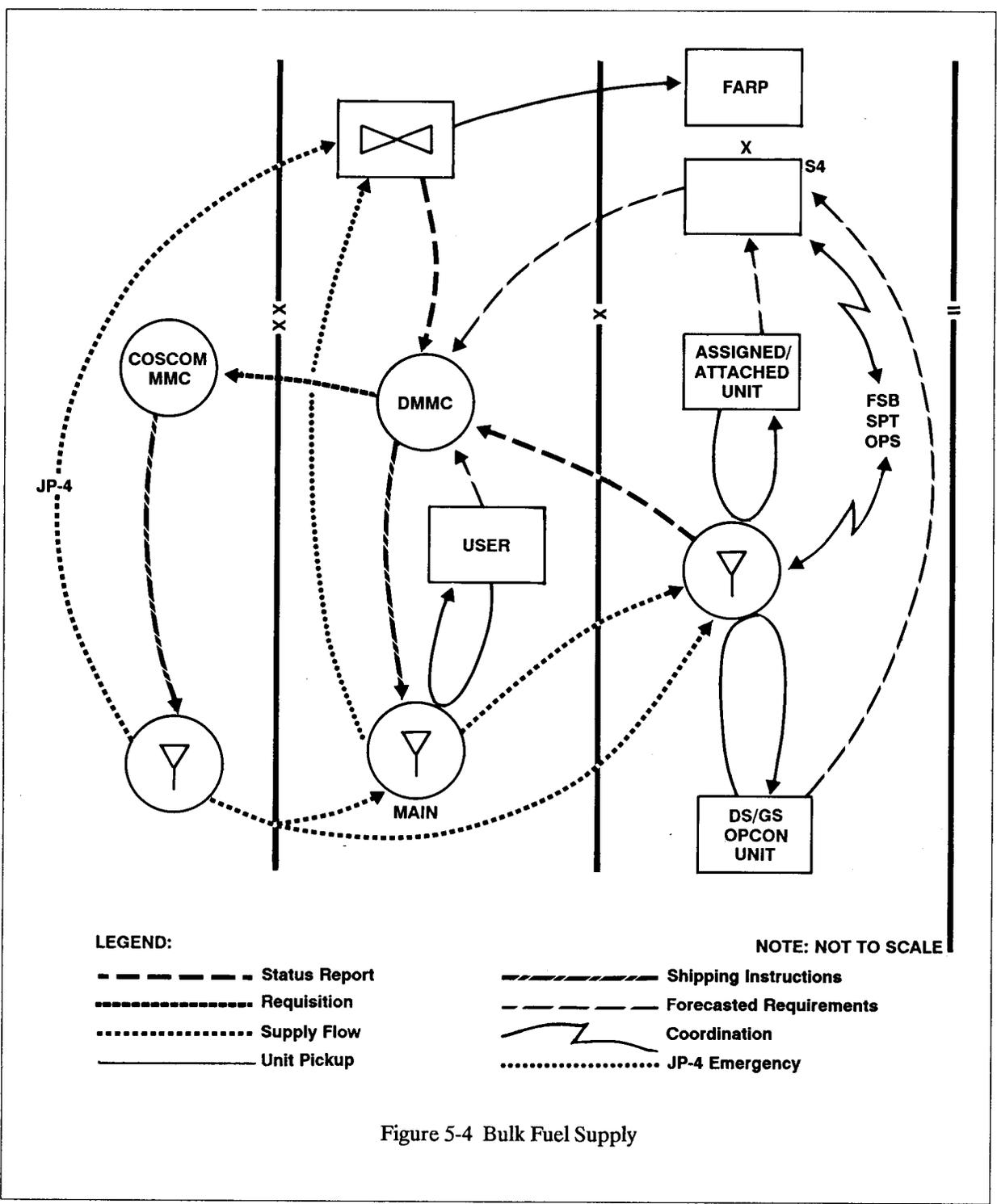
Figure 5-4 Bulk Fuel Supply
