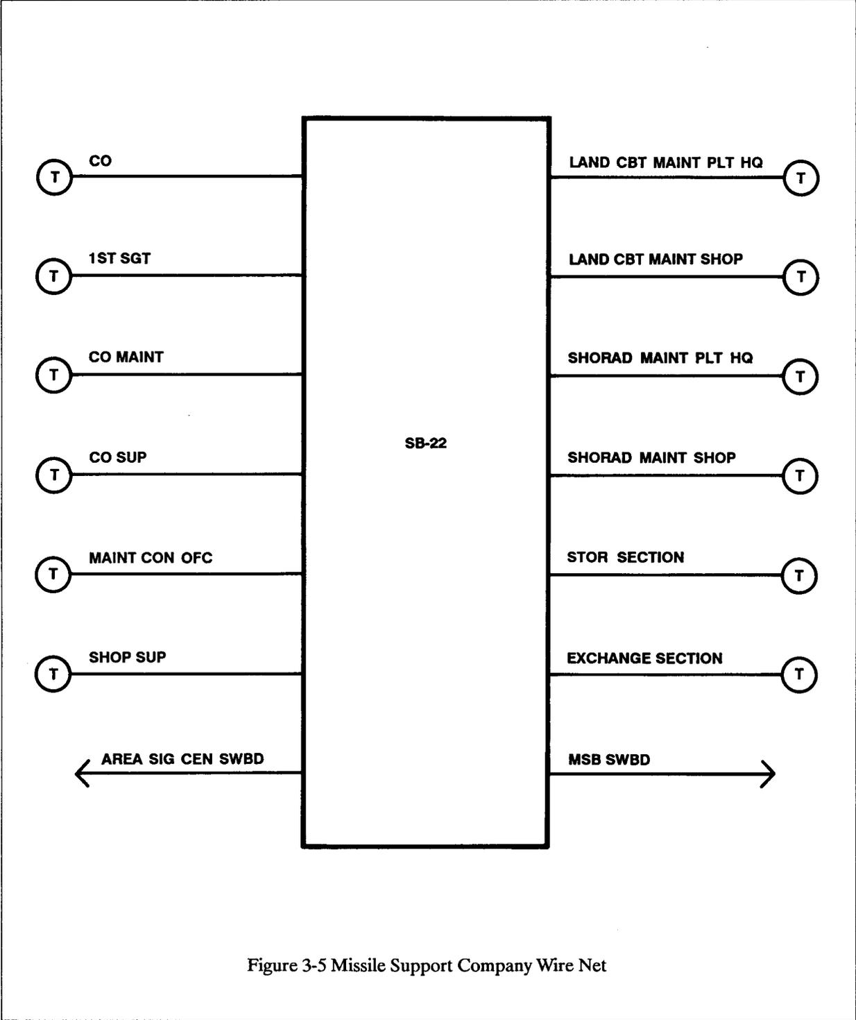
Figure 3-5 Missile Support Company Wire Net
