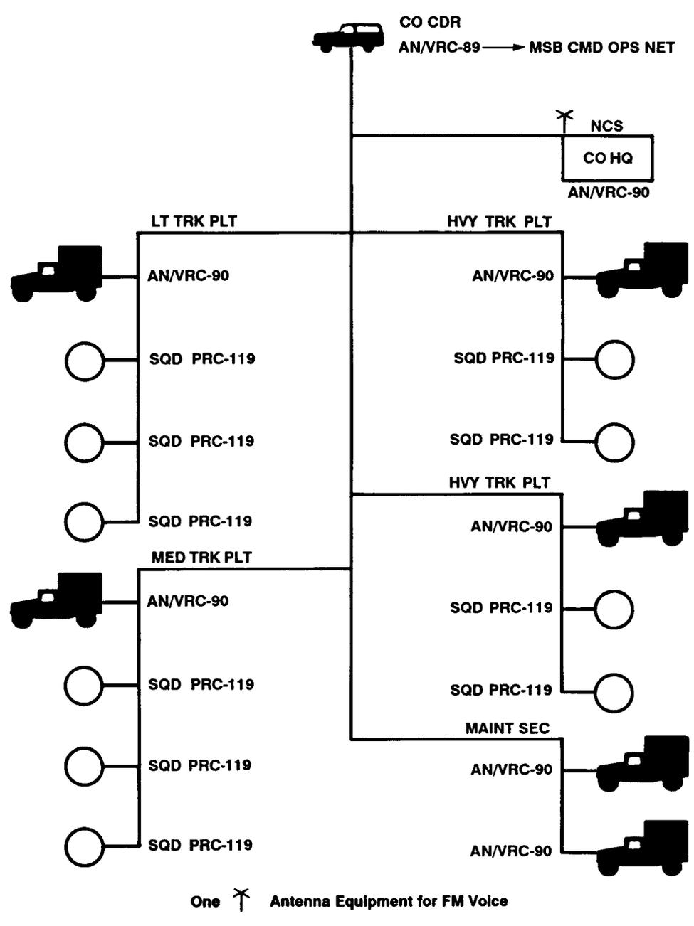
Figure 3-34 Transportation Motor Transport Company Command Net, FM (SINGARS)
