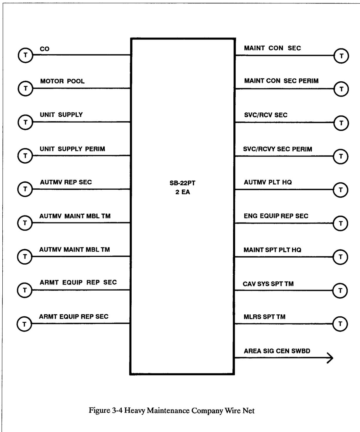
Figure 3-4 Heavy Maintenance Company Wire Net
