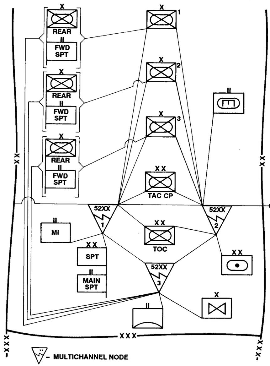
Figure 3-1 Sample Armored/Mechanized Infantry Division Multichannel Diagram
