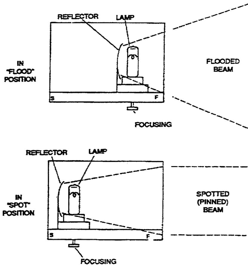
FIGURE 2-4. VARIABLE-FOCUS INSTRUMENT
