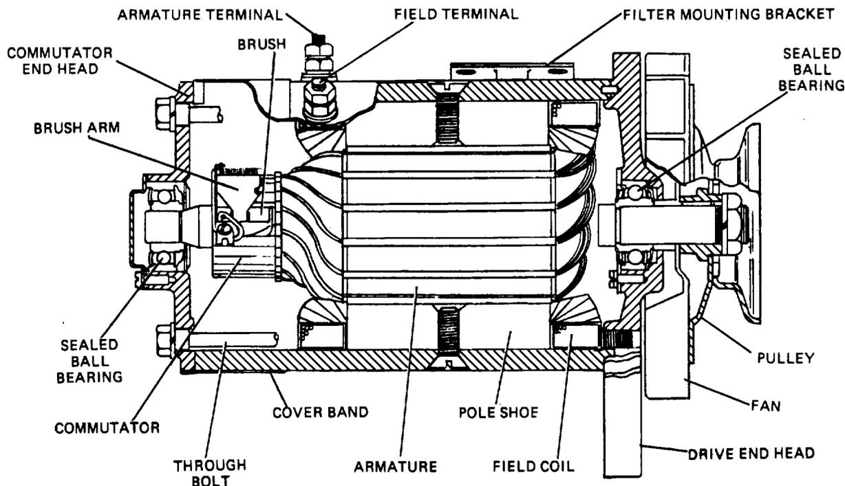
Figure 13-5. Shunt-Wound Generator.
