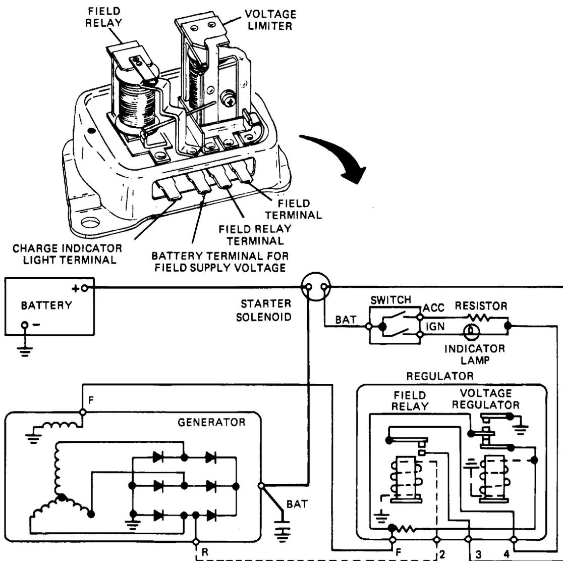
Figure 13-39. Field Relay and Warning Light Circuit.
