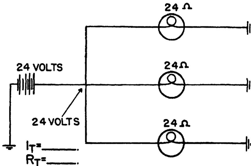
Figure 1-7. Parallel Circuits.
