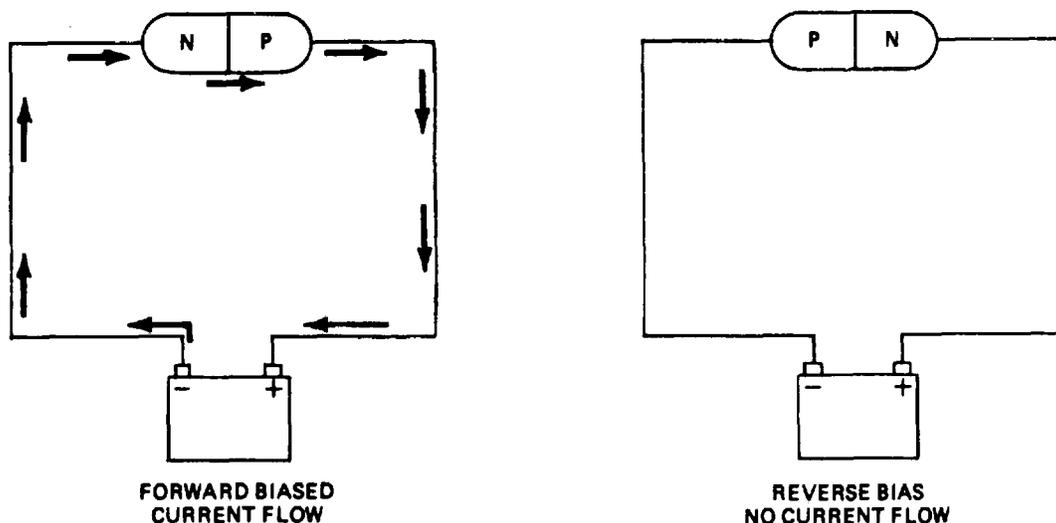
Figure 11-8. Diode Operation.
