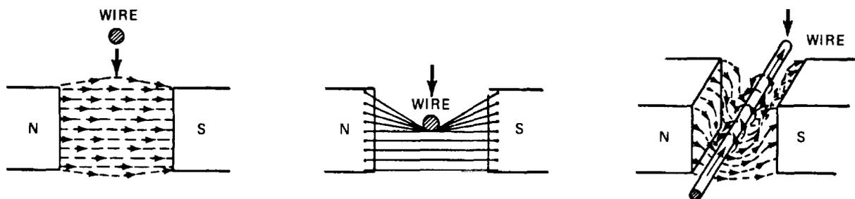
Figure 11-22. Electromagnetic Induction.
