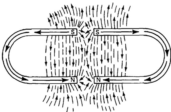
Figure 11-18. Electromagnetism.
