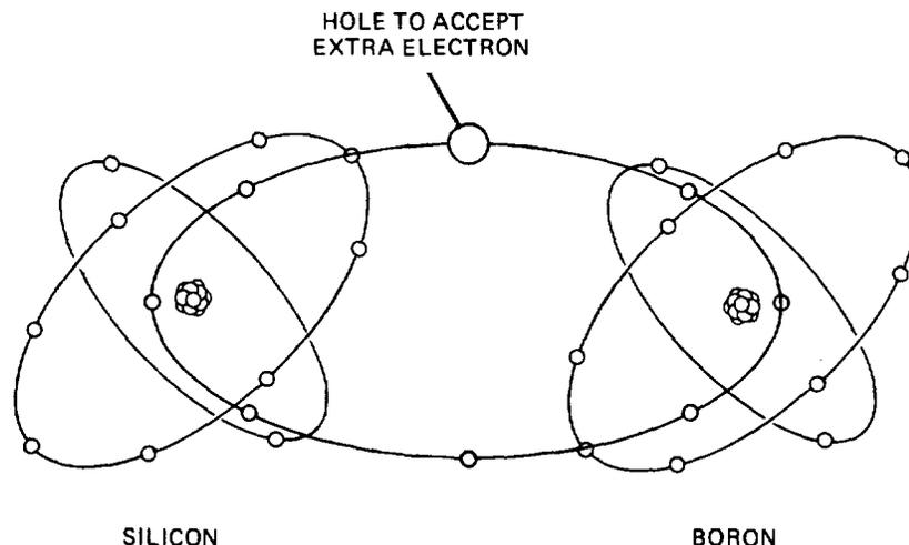
Figure 11-6. Boron-Doped Silicon.
