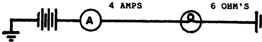
Figure 1-3. Determine Voltage.
