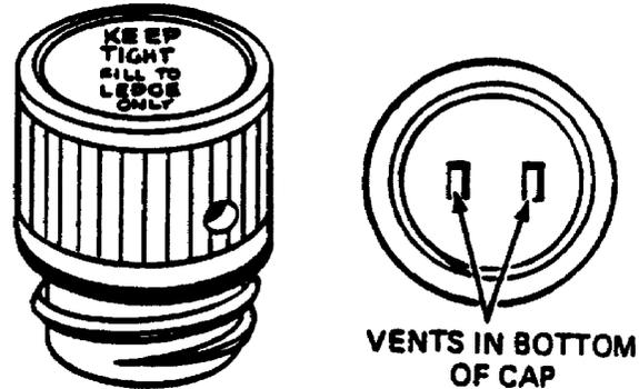
Figure 2-2. Vent Cap (Plug).
