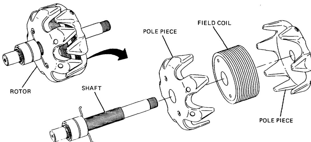
Figure 13-25. Rotor Construction.
