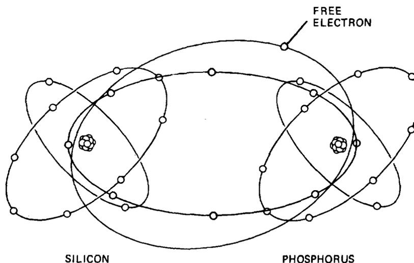
Figure 11-5. Phosphorus-Doped Silicon.
