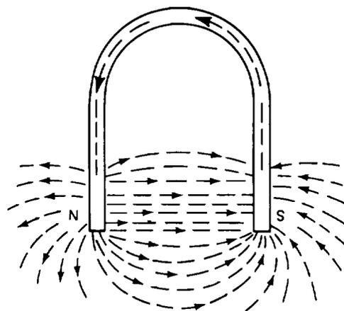
Figure 11-15. (3) The lines of force repel each other along their entire length and try to push each other apart.
