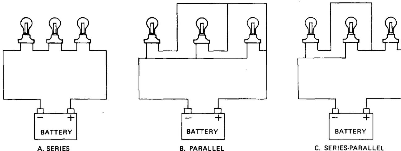
Figure 11-14. Circuit Configurations.
