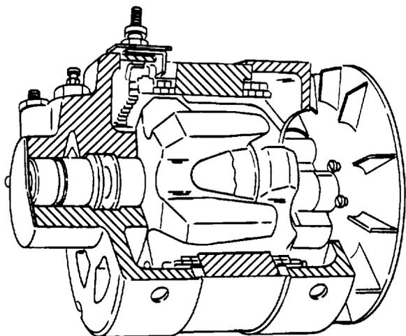
Figure 13-29. Rotor-to-Stator Relationship.
