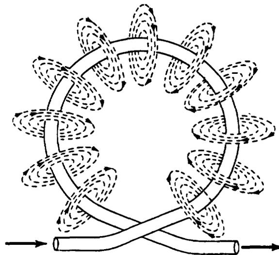
Figure 11-19. Electromagnetism in a Wire Loop.
