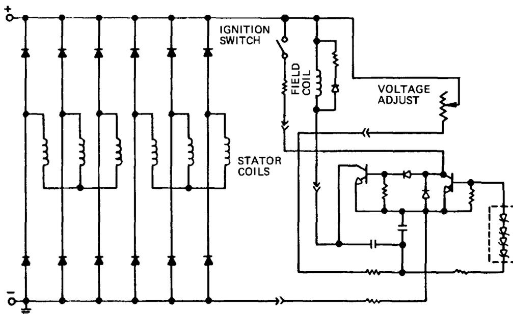
Figure 13-31. Inductor Alternator
