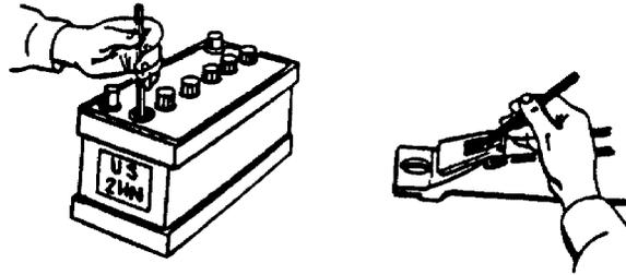
Figure 2-6. Electrolyte Sample.
