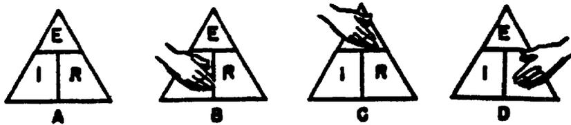
E = Volts, I = Current in Amperes, R = Resistance in Ohms
