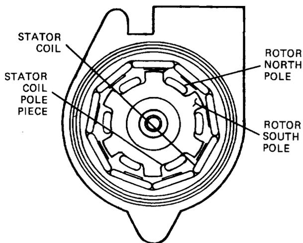
Figure 13-27. Rotor-to-Stator Relationship.
