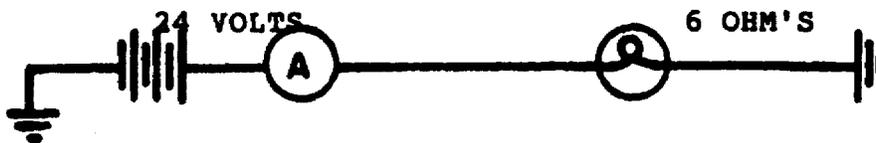
Figure 1-4. Determine Current.
