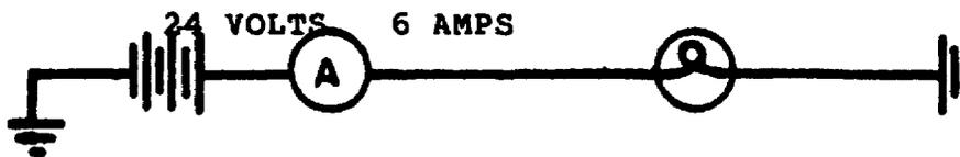
Figure 1-5. Determine Resistance.
