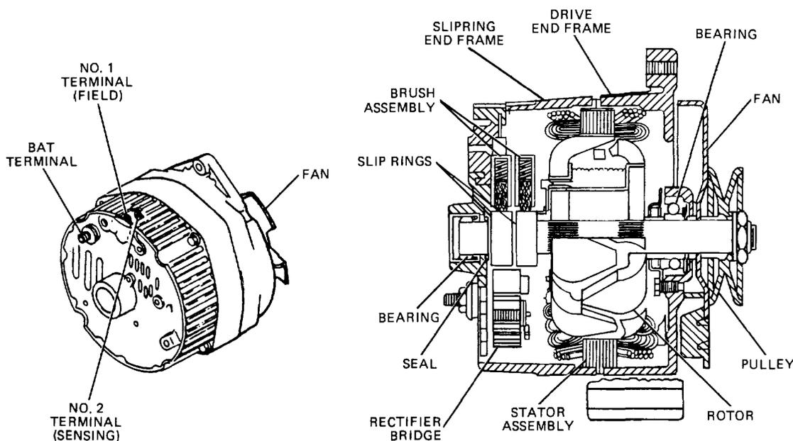
Figure 13-21. Typical Alternator.
