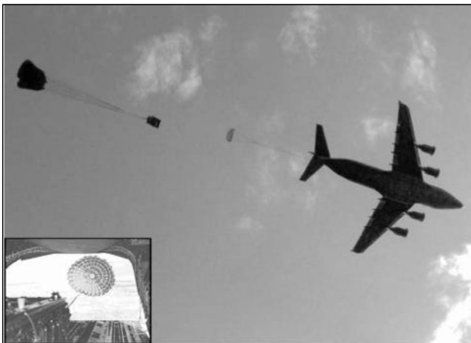
**Figure 2.2. Aerial Extraction Method of Aerial Delivery**
