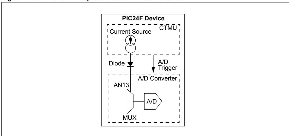
At 25°C, the forward voltage of the temperature diode is 0.83V. The rate of change between the forward voltage of the diode and its temperature is 1.87 mV per degree Celsius. The formula shown in Equation 11-7 can be used to calculate the forward voltage.
