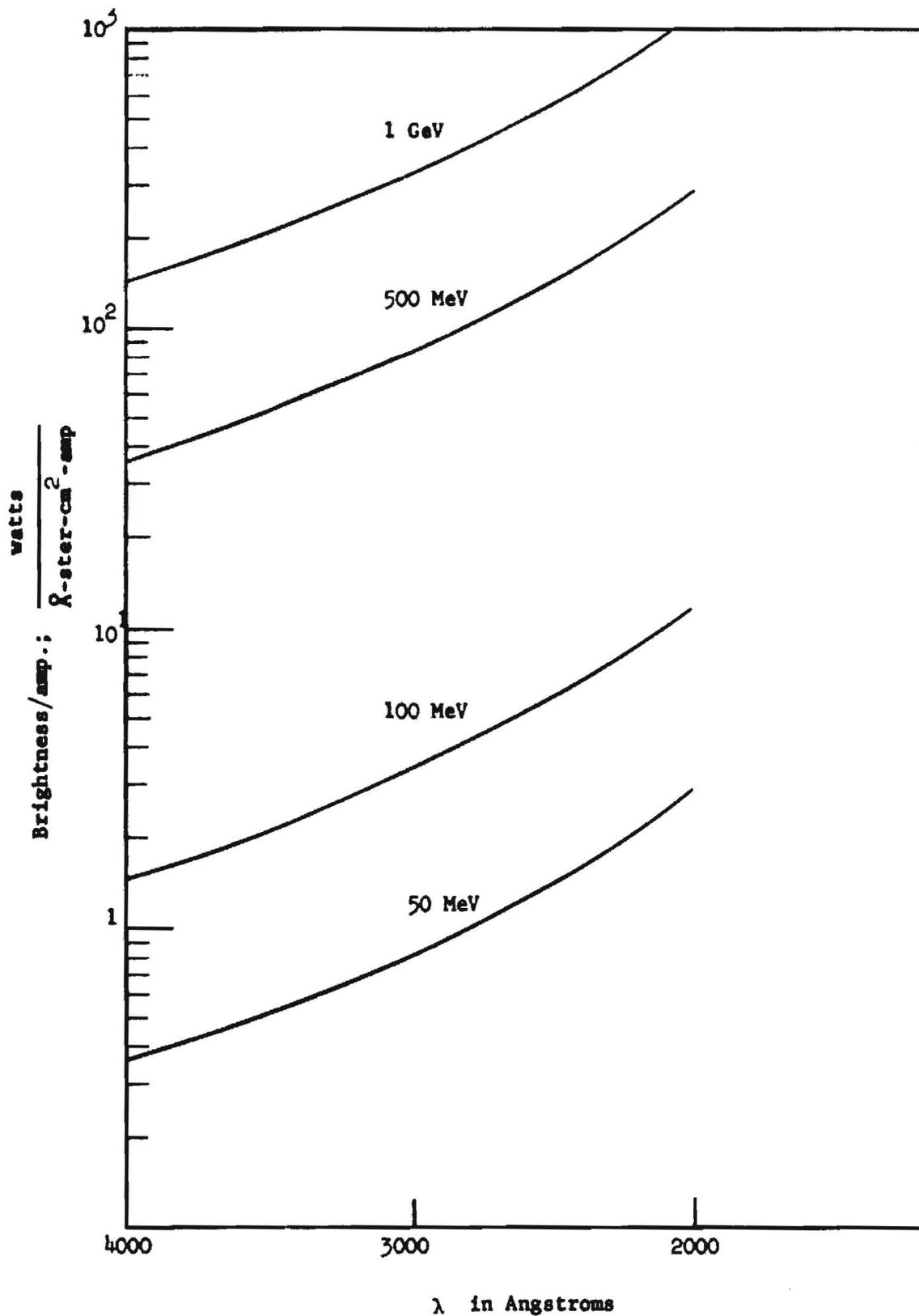
Fig. 4--Brightness per ampere vs wavelength from quartz at various electron beam energies for path lengths,  $L \gg L_{\min}$  where
