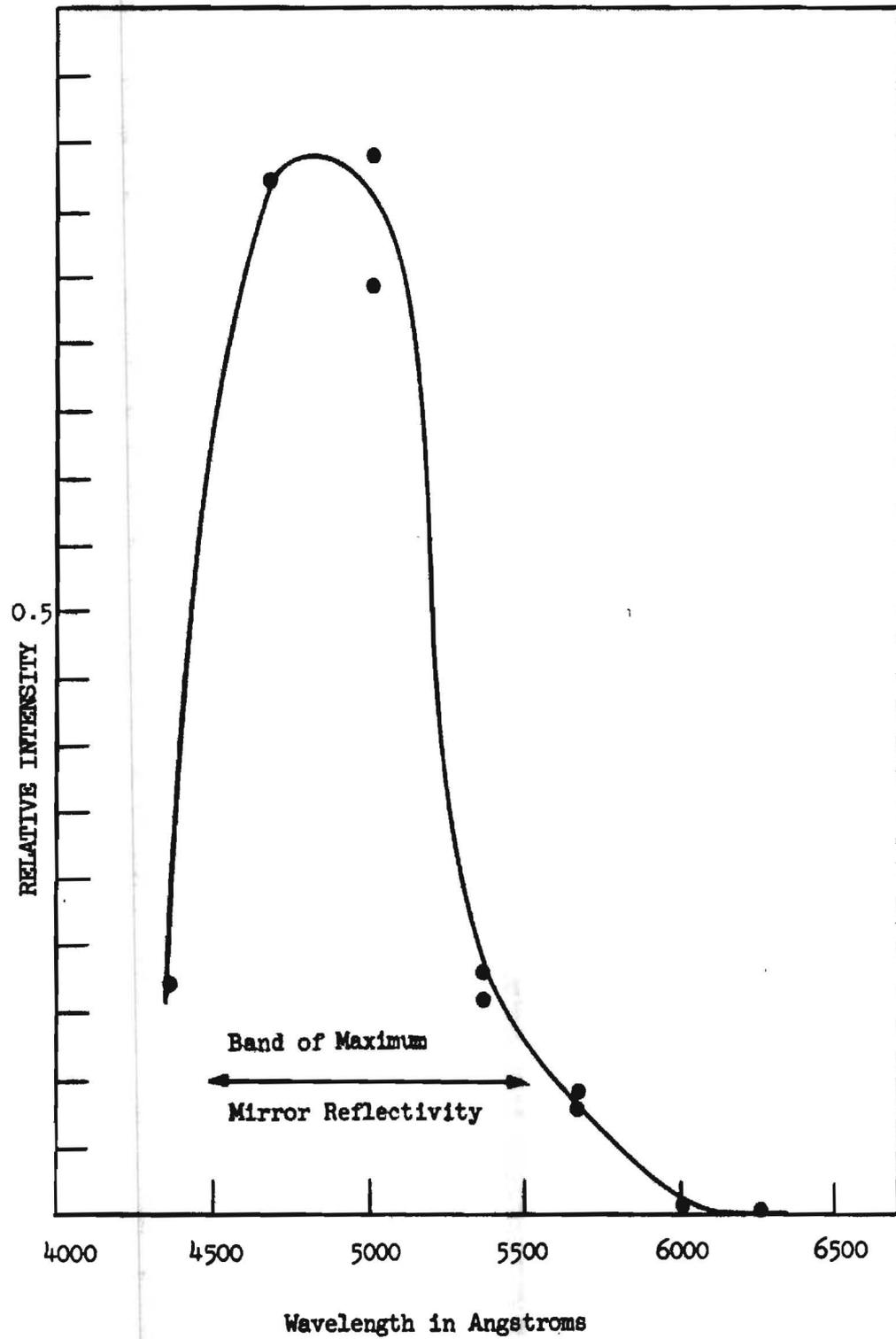
FIG. 16--Spectral distribution of Cerenkov light from quartz coated with dielectric mirrors.
