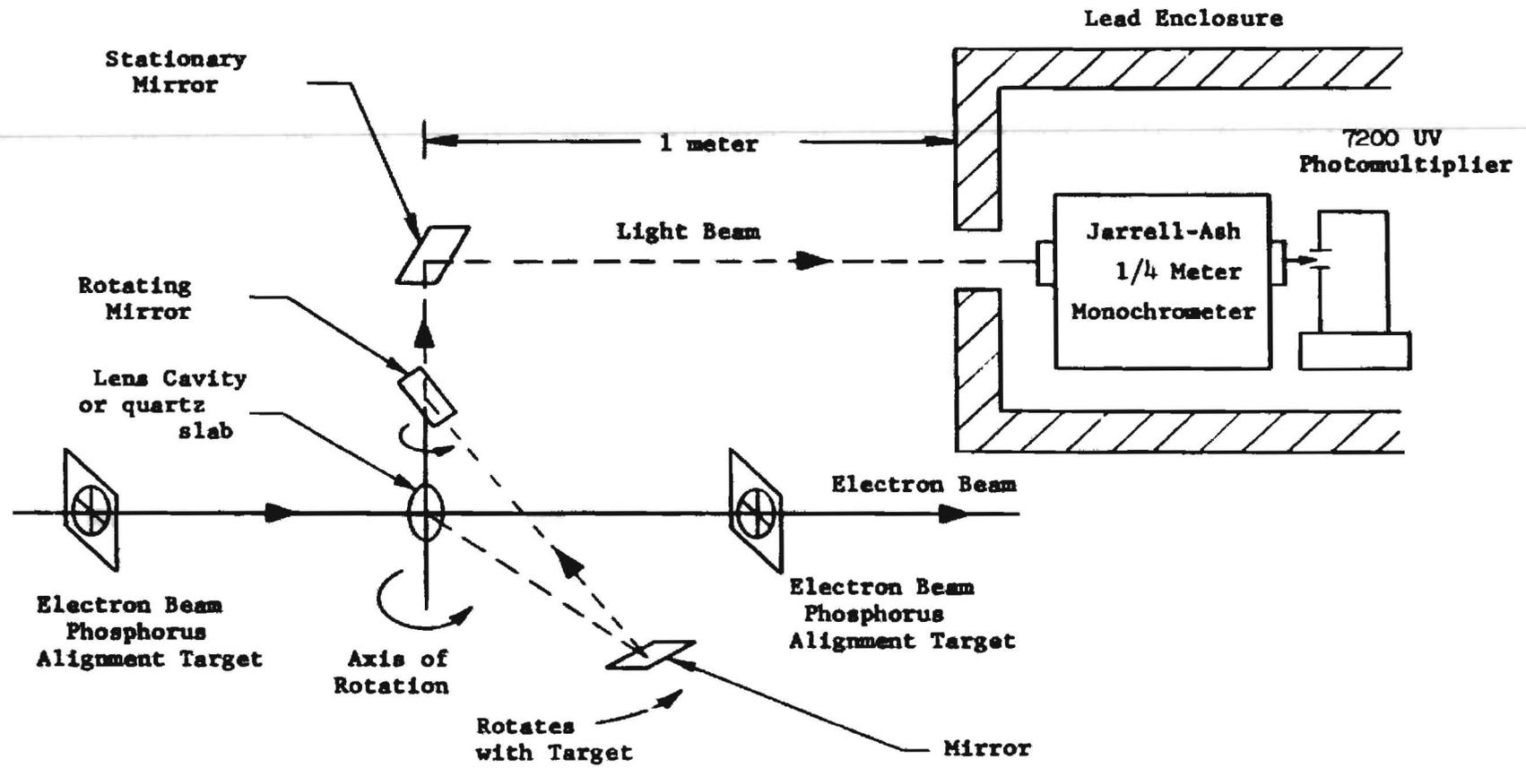
Fig. 9--Experimental setup for the brightness measurement of the spontaneous and stimulated Cerenkov effects.
