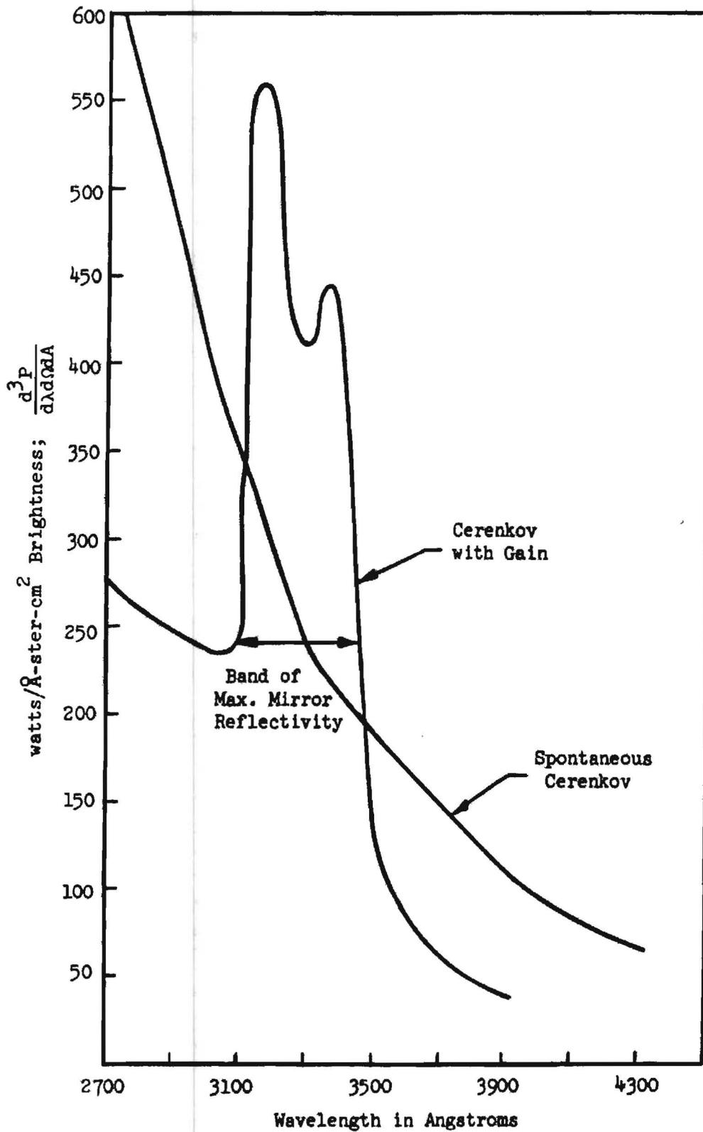
FIG. 17--Spectral distribution of Cerenkov light from quartz coated with dielectric mirrors whose band of maximum reflectivity is at 3250 Å .
