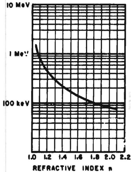
Fig. 2--Minimum threshold electron energy for Cerenkov Radiation to occur.
