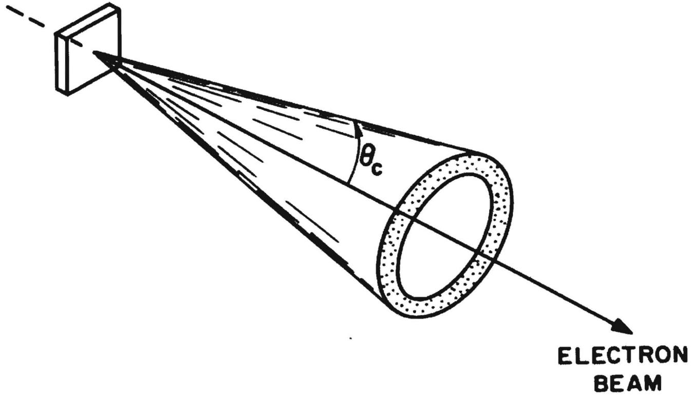
FIG. 1--Generation of Cerenkov light cone at angle  $\theta_c$ .
