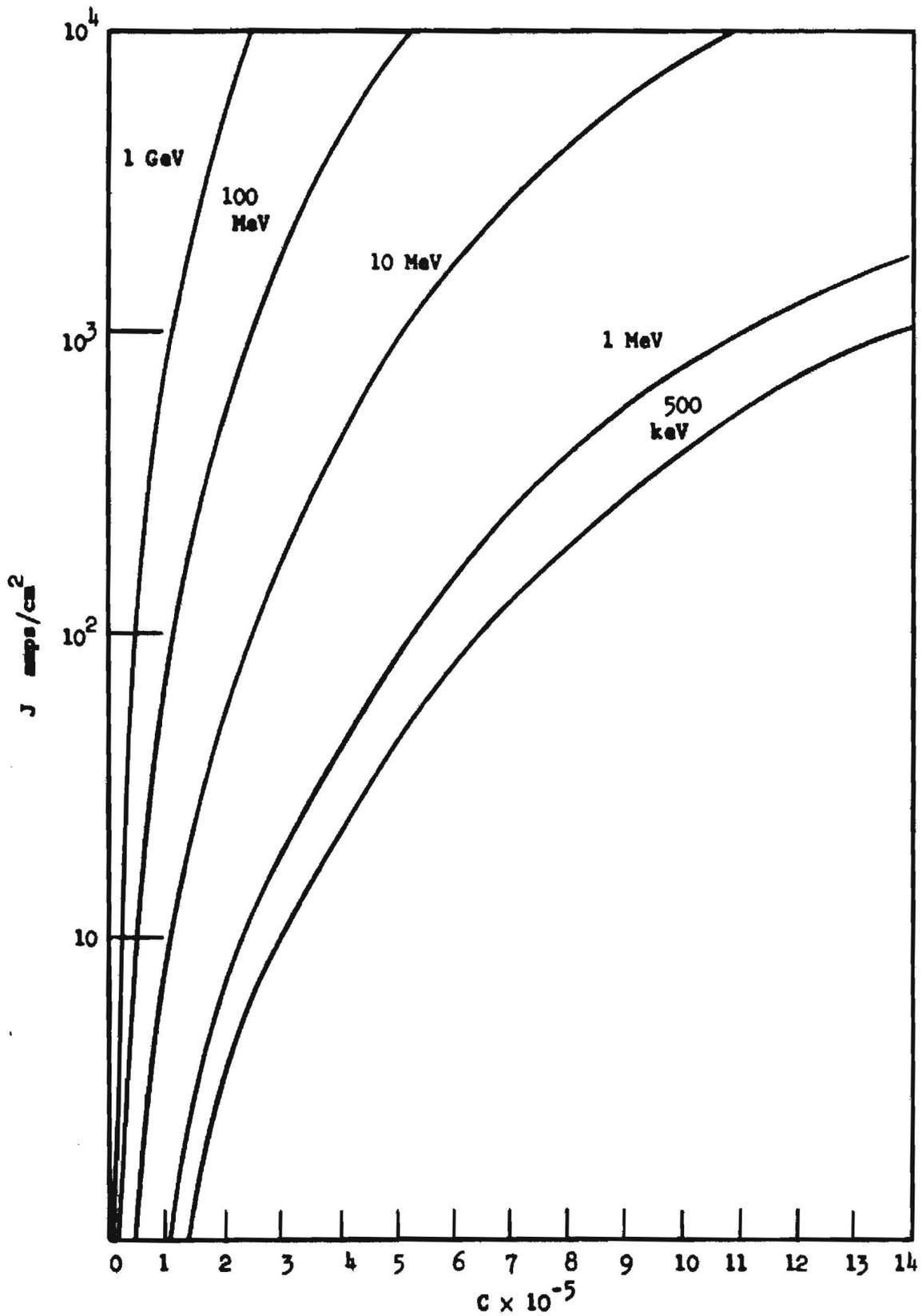
Fig. 6--The gain constant  $C$  versus current density for various electron beam energies ( $\lambda = 3000 \text{ \AA}$ ).
