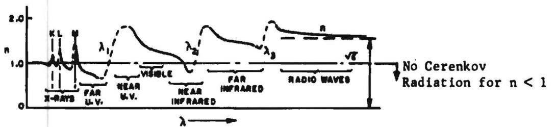
Fig. 3--The dispersion curve of a typical transparent medium over the whole electromagnetic spectrum. (After Jenkins and White, 1937).
