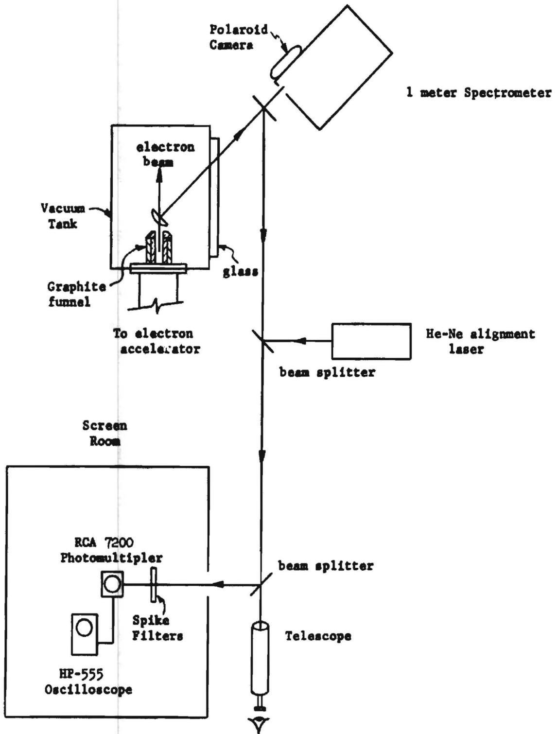
Fig. 15--Experimental setup using low energy, high current electron accelerator at Physics International, San Leandro, California.
