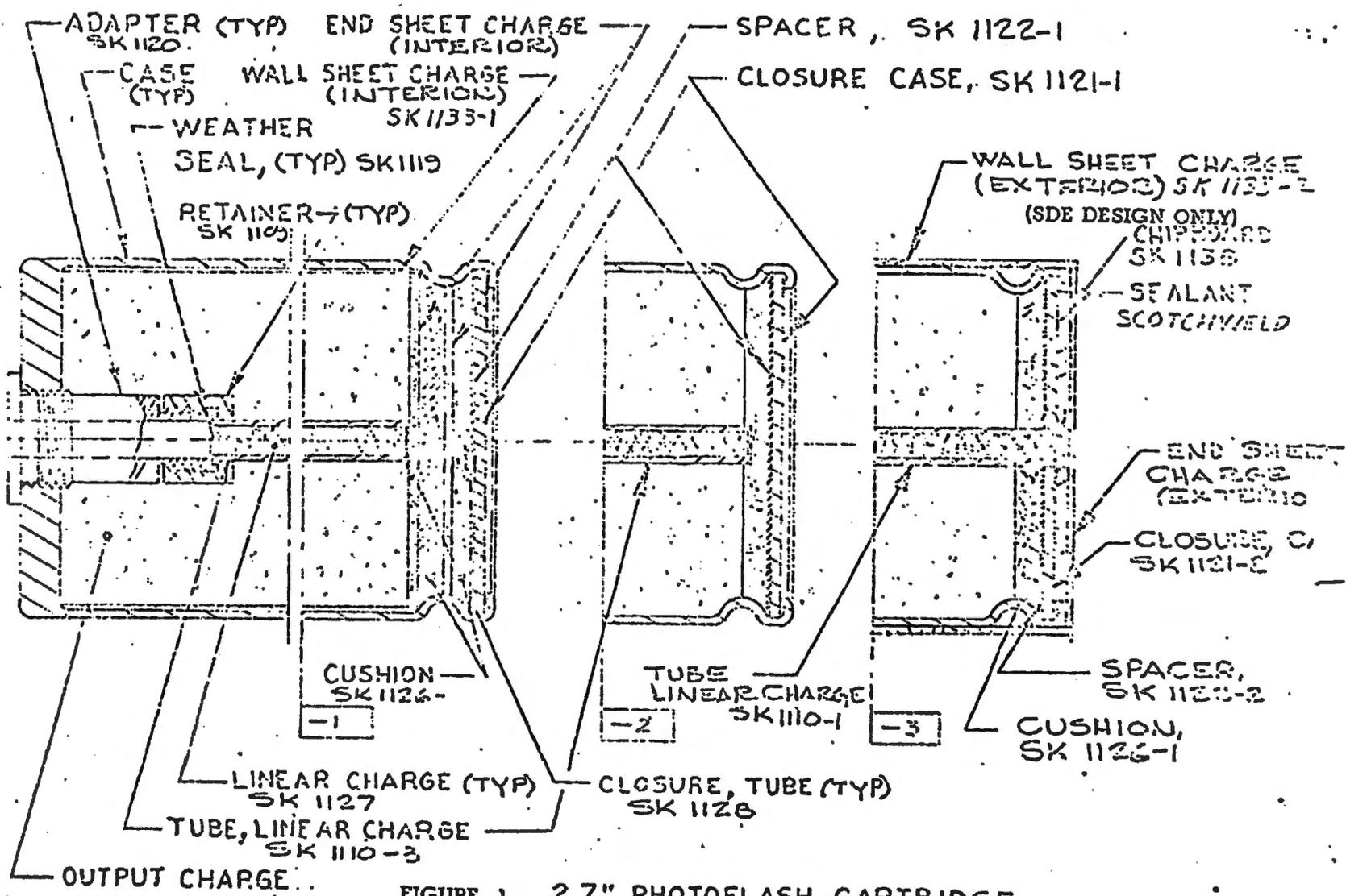
FIGURE 1. 2.7" PHOTOFLASH CARTRIDGE
