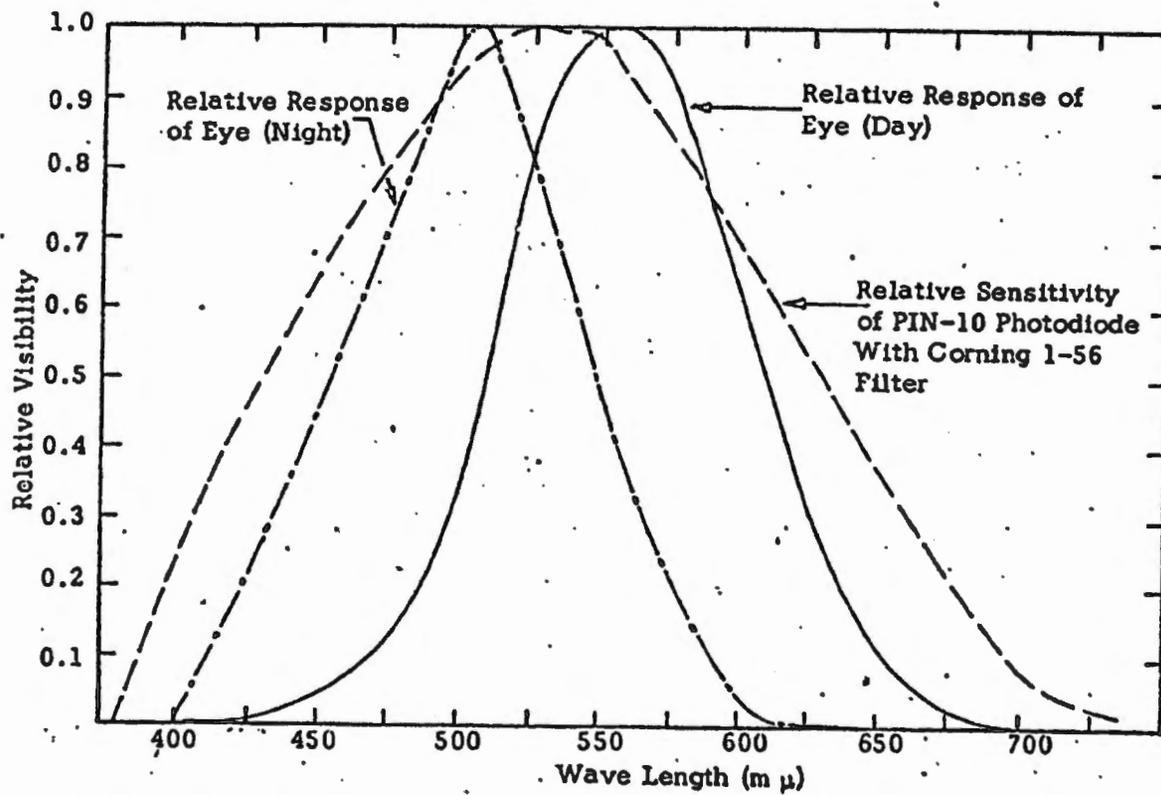
Figure 4. Comparison of Eye and Photodetector Sensitivity Curve.
