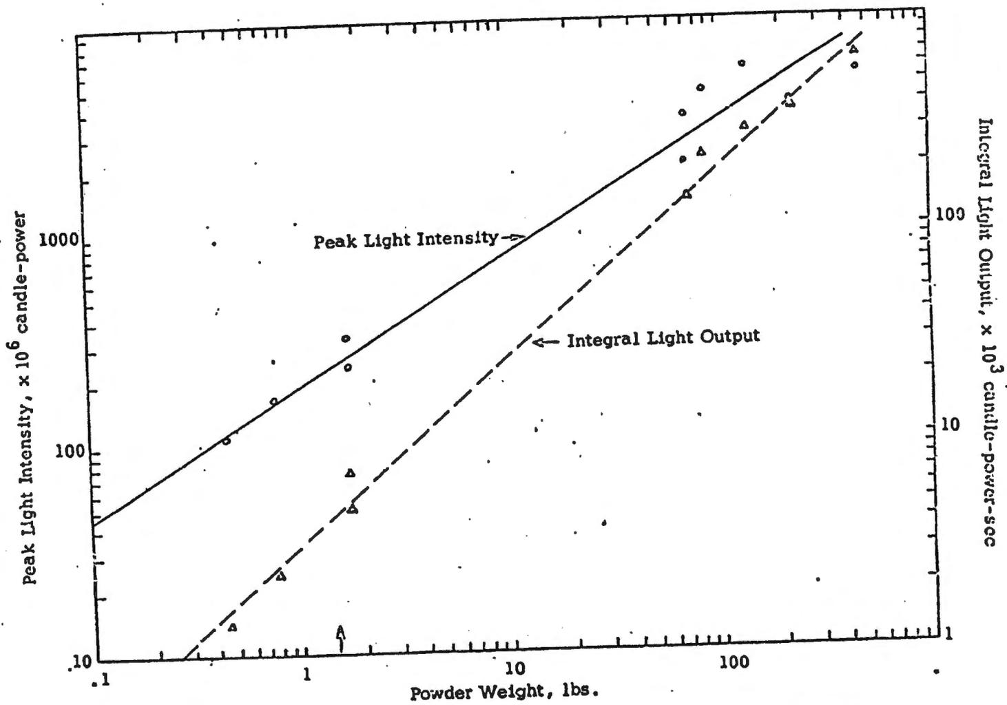
Figure 9. Peak Intensities Produced by Type III Photoflash Mixtures as a Function of Charge Weight<sup>2</sup>.
