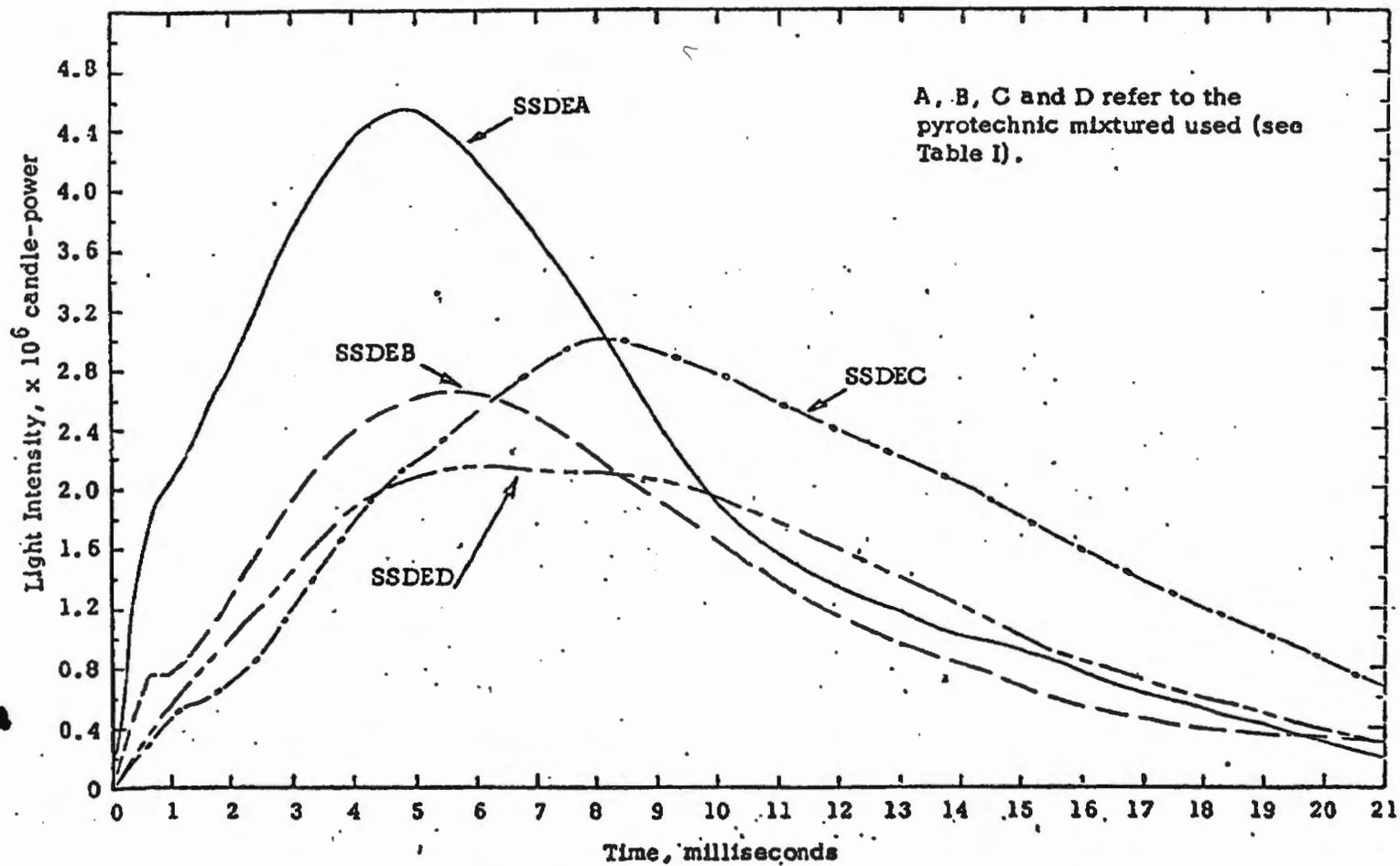
Figure 8. Light Output From Series SSDE Photoflash Units
