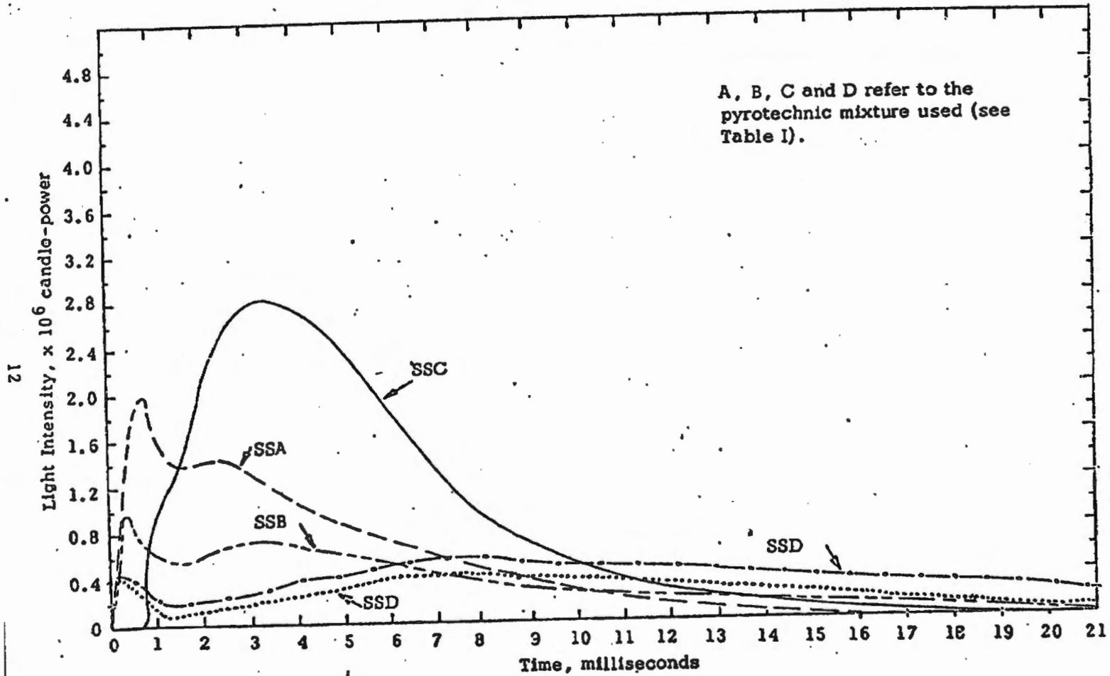
Figure 7. Light Output From Series SS Photoflash Units
