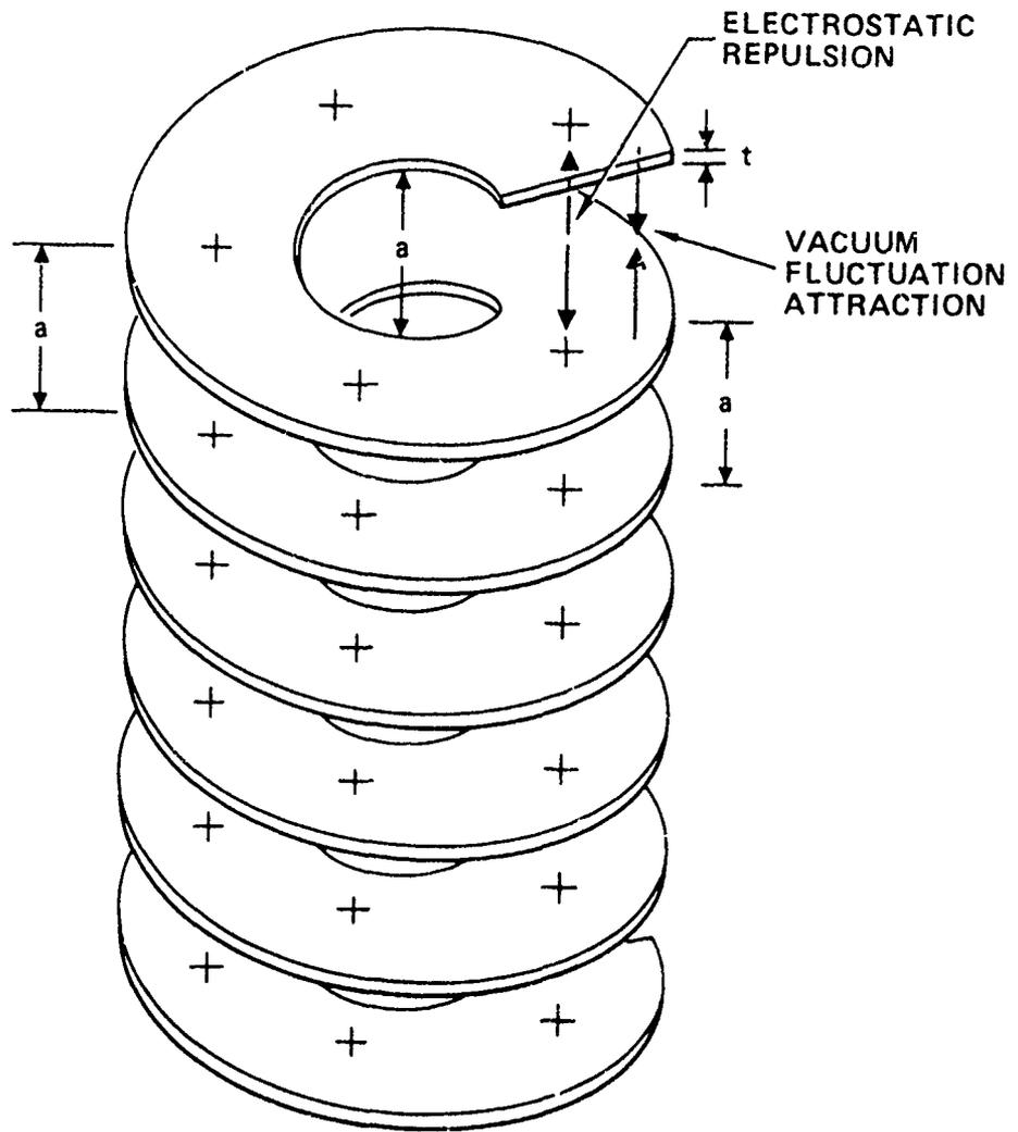
Figure 2 - Spiral design for a vacuum fluctuation battery.
