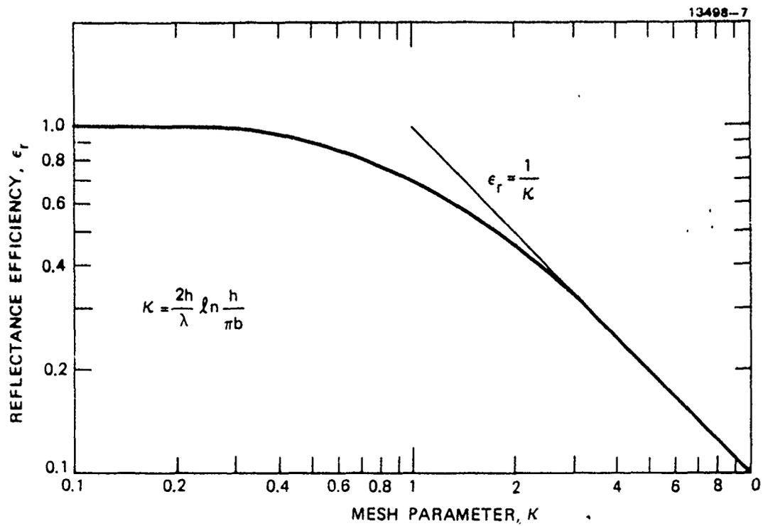
Figure 2. Mesh reflectance vs. wire size and spacing
