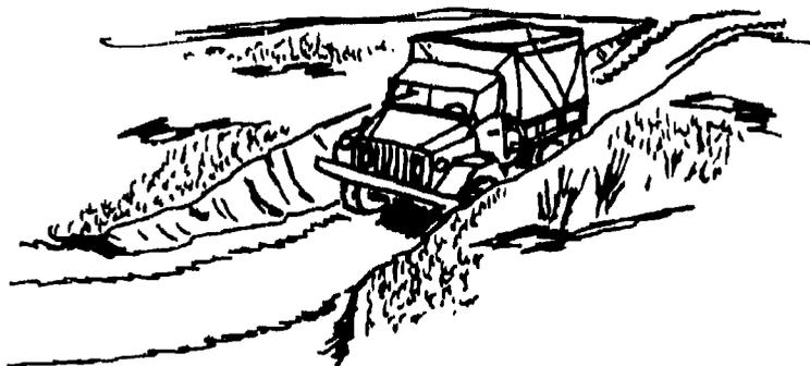
FIGURE 22. PROTECTION OF VEHICLES IN SLOT TRENCHES.
