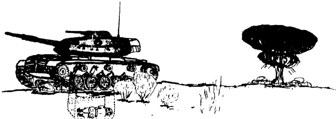
FIGURE 7. USING TRACKED VEHICLES AS EXPEDIENT OVERHEAD COVER.
