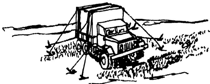
FIGURE 21. ANCHOR AND TIE DOWN VEHICLE AND CARGO.
