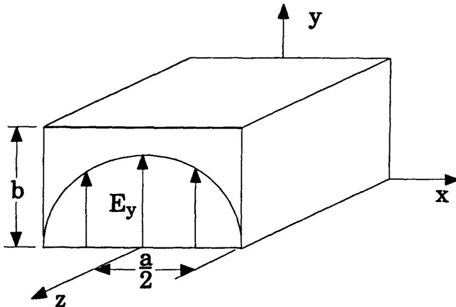
Figure 1a. Coordinate convention for a rectangular waveguide.
