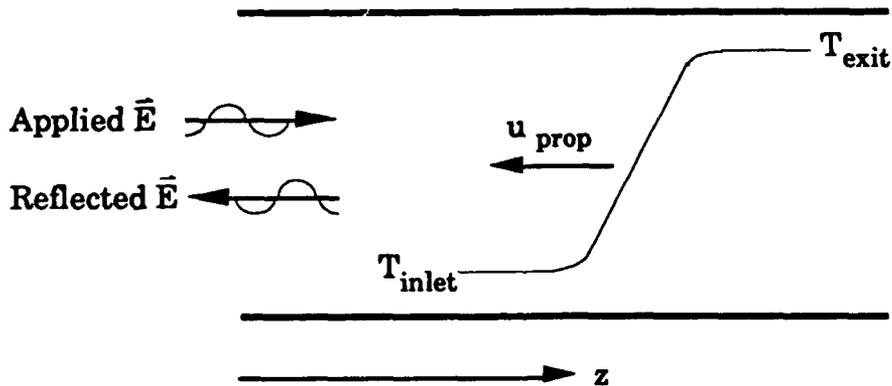
**Figure 2. Schematic of plasma propagation in a rectangular waveguide.**
