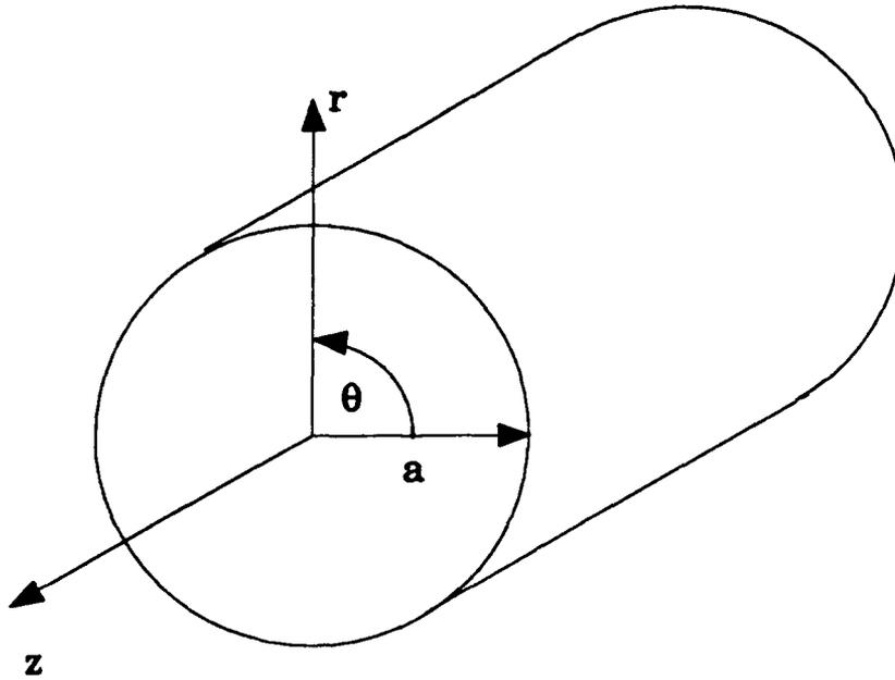
**Figure 1b. Coordinate convention for a cylindrical waveguide.**
