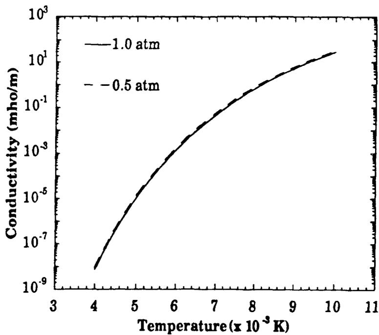
Figure A5. Electrical conductivity values for helium at .5 and 1 atmosphere pressure.
