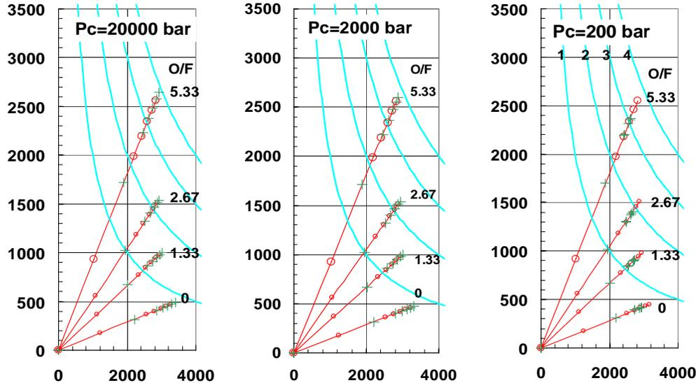
**FIGURE 2.** Coupling coefficient (ordinate, N/MW) vs Isp (abscissa, m/s) for various formulations of Delrin with AN: O/F = 5.33, 2.67, 1.33, 0, and addition of 7 MJ/kg of laser energy at constant pressure (200000, 2000, 200 bar), followed by expansion with expansion ratios of  $\epsilon = 1, 4, 8, 16, 32, 64$ , using NASA CEA code, chemical equilibrium code. Hyperbolic constant apparent efficiency lines (constant apparent  $\alpha\beta$ ) are shown at 100%, 200%, 300%, and 400 %.
