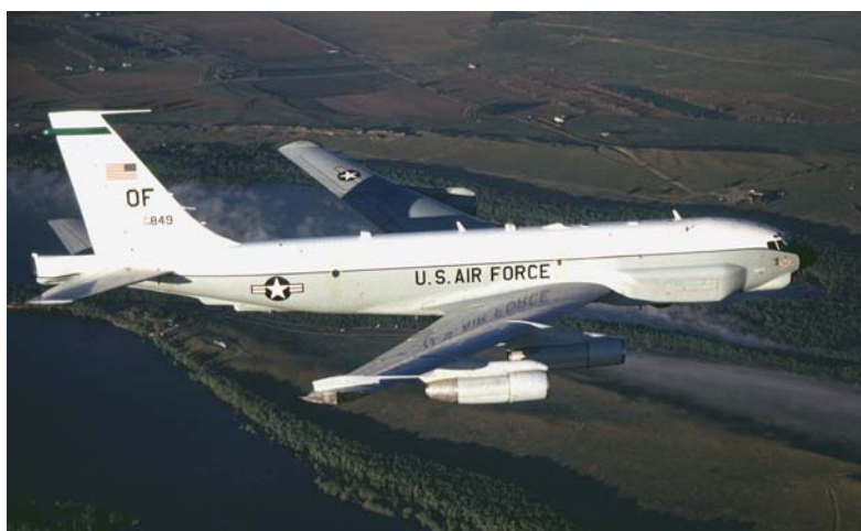
Modified RC-135U advanced ELINT airborne collection platform
