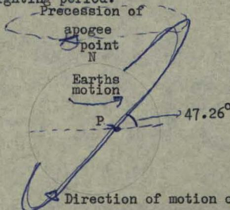
The sketch shows the satellite and Earth (not to scale). If the Earth were stationary the satellite would always cross the equator at point P, but due to the Earth's motion of 361° per day from West to East, then after one orbit has elapsed the point P will have moved eastward by  $361^\circ \times \frac{115.15}{24 \times 60} = 28.87^\circ$ .
