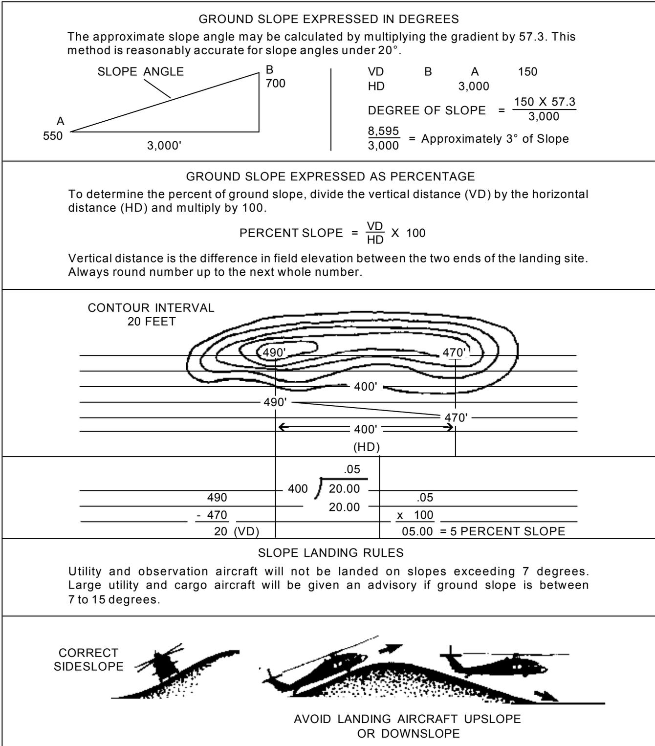
Figure 2-3. Determining ground slope
