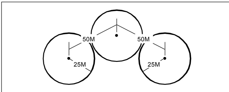
Figure 2-2. Size 3 aircraft landing zone for V-formation
