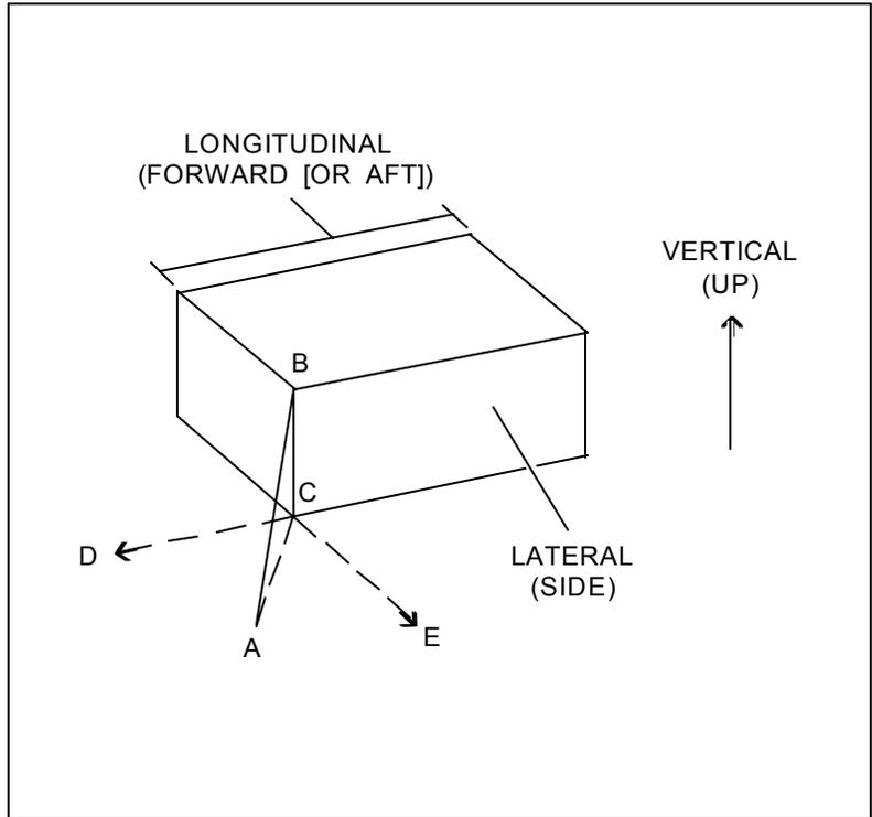
Figure 2-26. Longitudinal angle of tie-down
