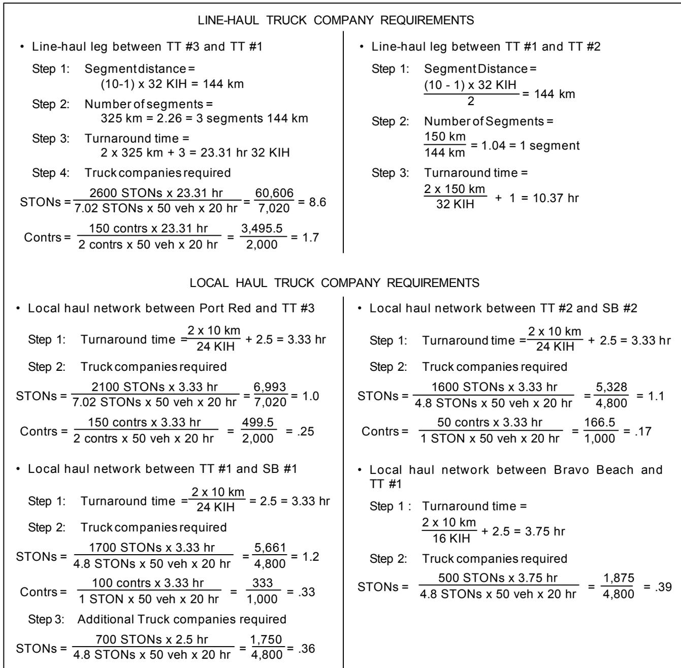
Figure 3-10. Line-haul and local haul truck company requirements
