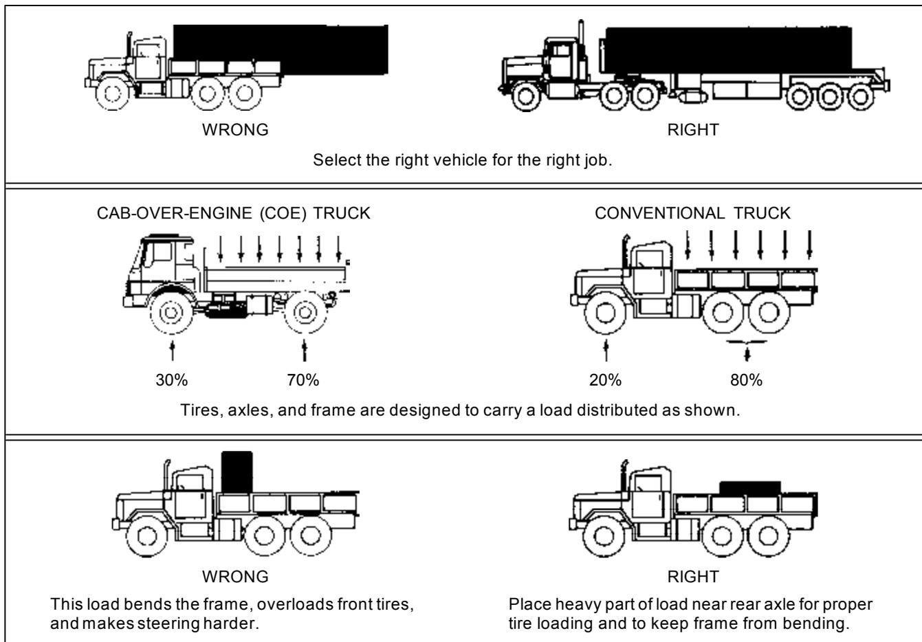
Figure 3-12. Load placement in trucks and semitrailers
