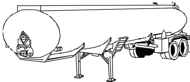
M1062, 4 X 4, 7,500-GALLON, SEMITRAILER, TANK, FUEL
