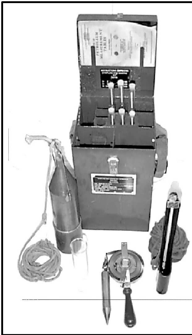
Figure 4-2. Sampling and Gaging test kit
