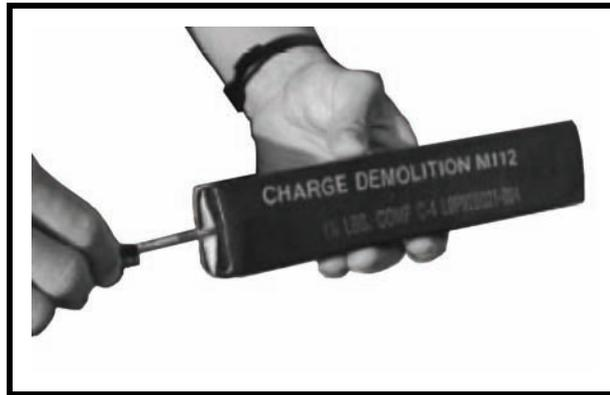
Figure 14-9. Priming of C4 demolition blocks with MDI.
