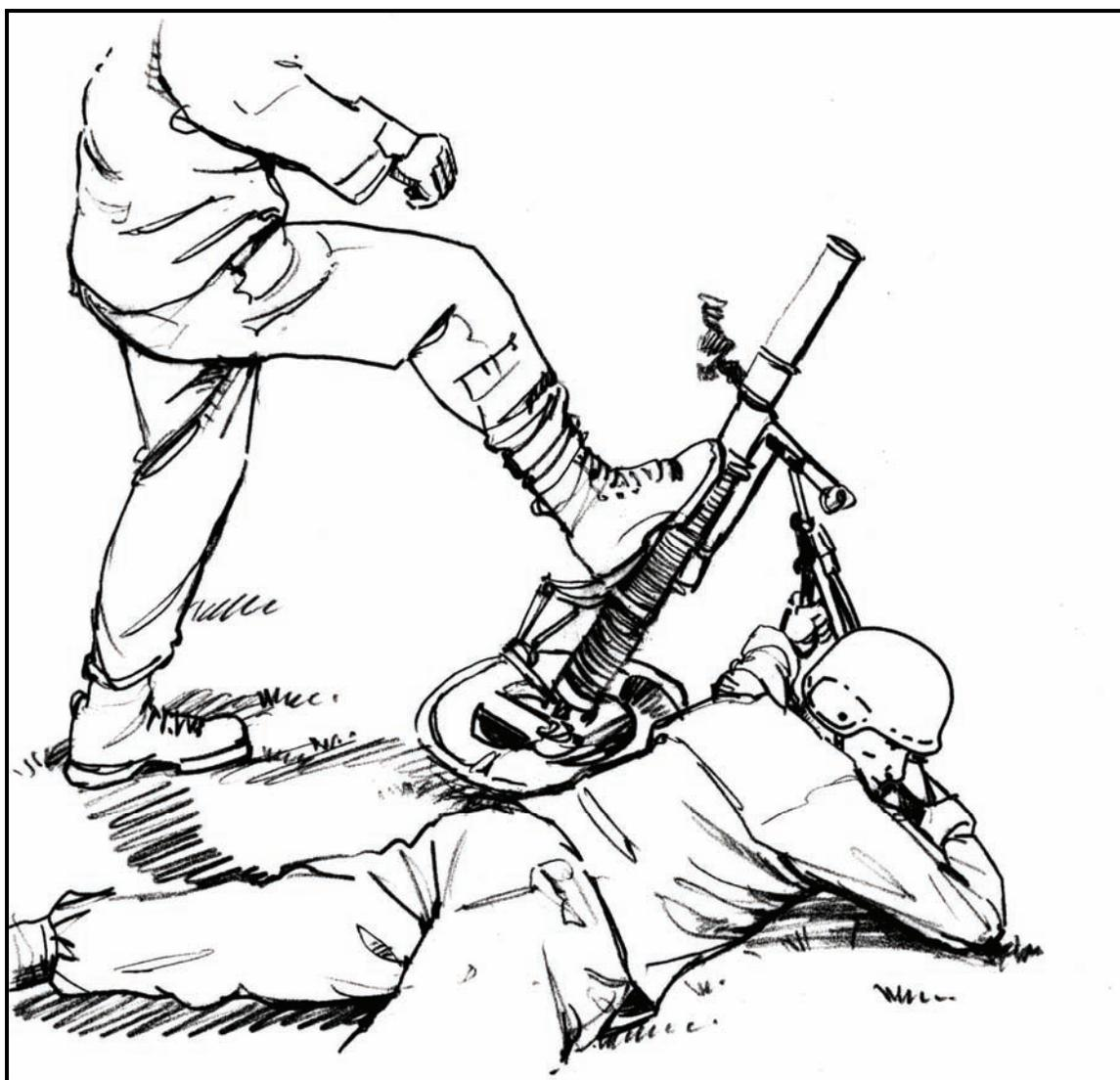
Figure 3-8. Kicking the mortar to clear a misfire.
