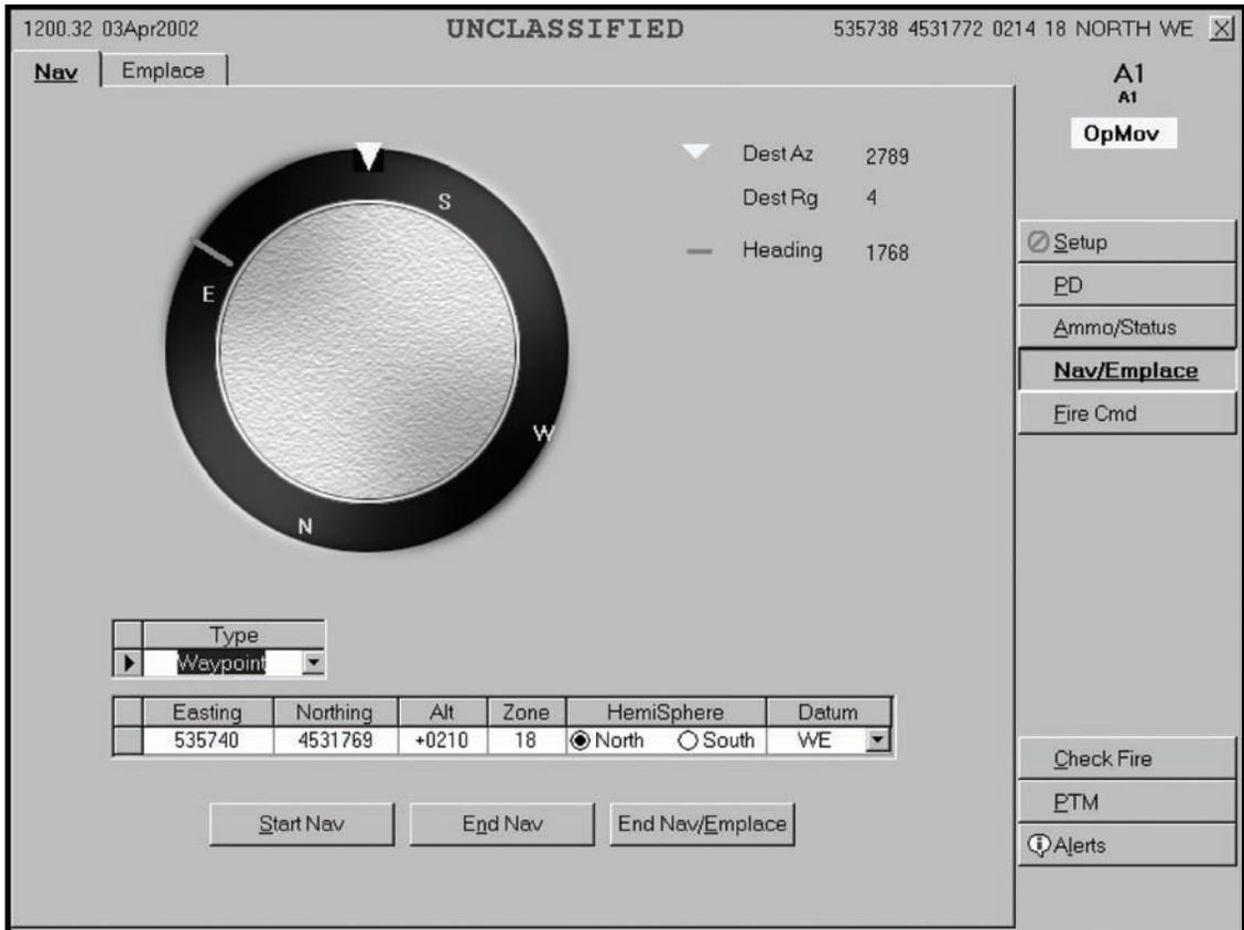
Figure 7-6. “Navigation/Emplacement” screen: destination azimuth, destination range, and heading.
