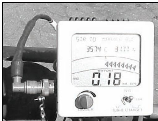
Figure 7-5. Driver's display showing steering directions, distance, and position.
