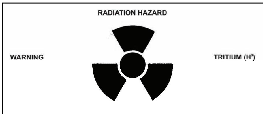
Figure 2-13. Warning label for tritium gas ( $H^3$ ).
