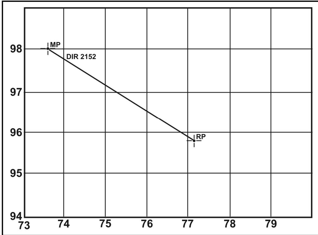
Figure B-5. Determining direction from mortar position to the registration point.
