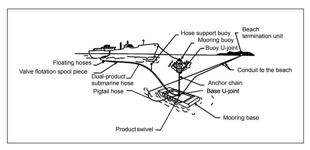
Figure 1-3. OPDS SALMS Sunk to the Bottom and Acting as a Mooring and Discharge Station
