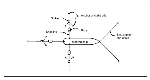
Figure 1-2. Multiple-Point Mooring System
