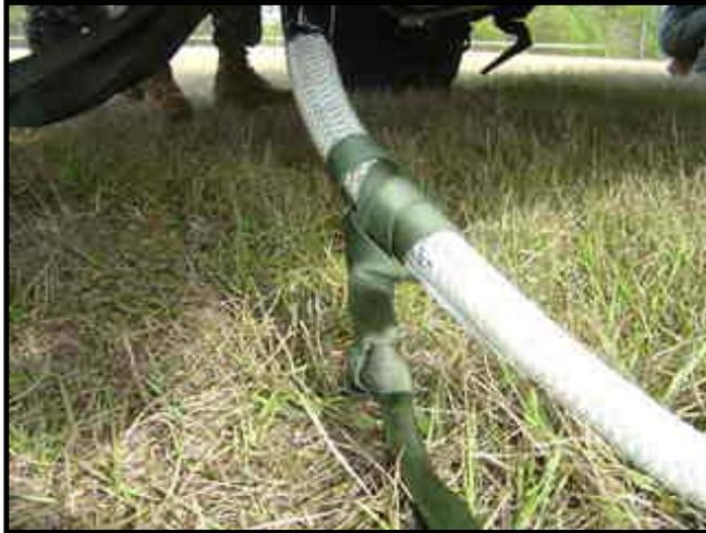
**Figure 5-7. Recovery line with Prusik knot.**
