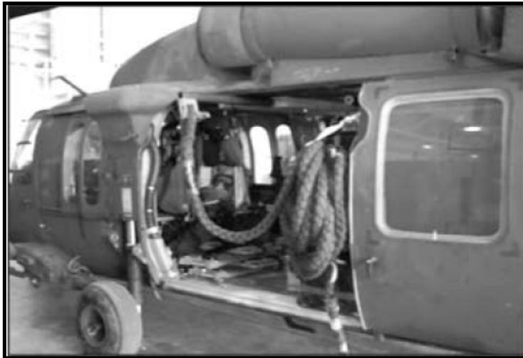
Figure 5-10. UH-60 rigged for fast roping
