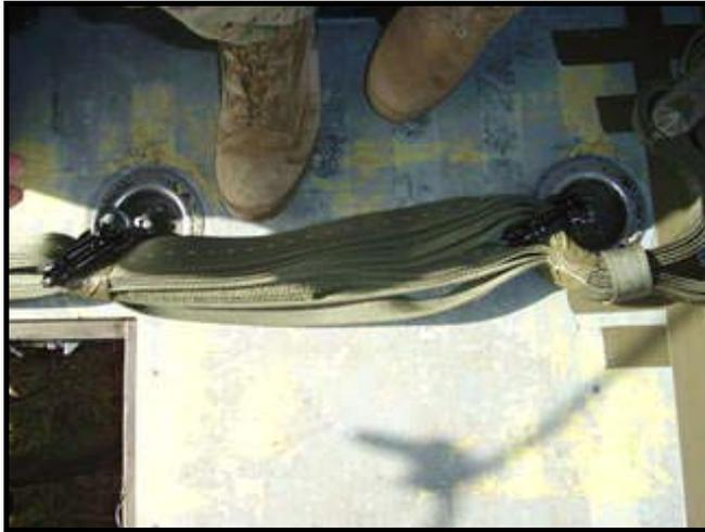
Figure 5-4. Rigging of snap links.
