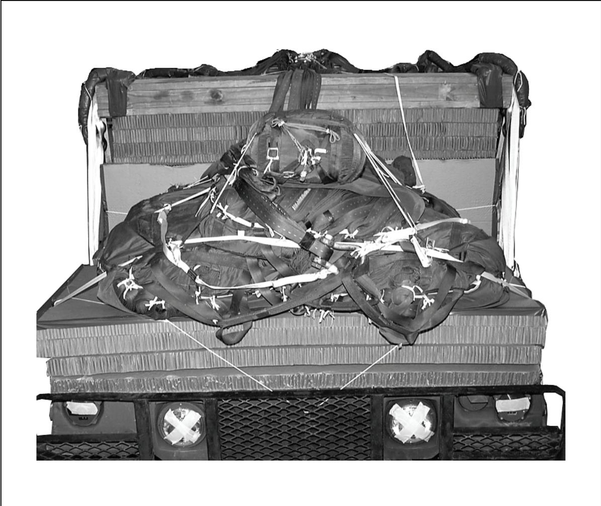
Figure 4-17. Deployment Parachute Installed
