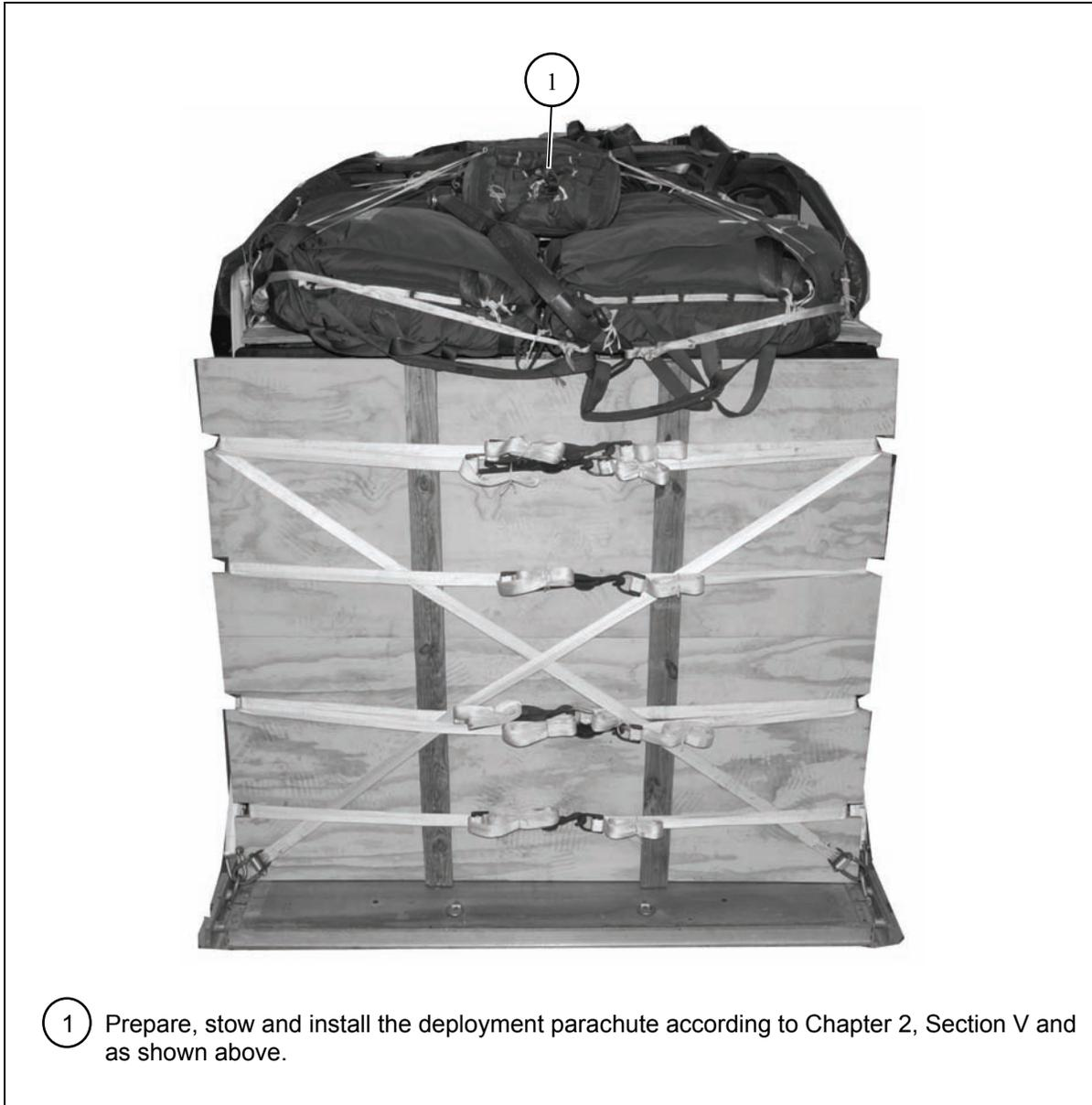
**Figure 8-29. Deployment Parachute Installed**
