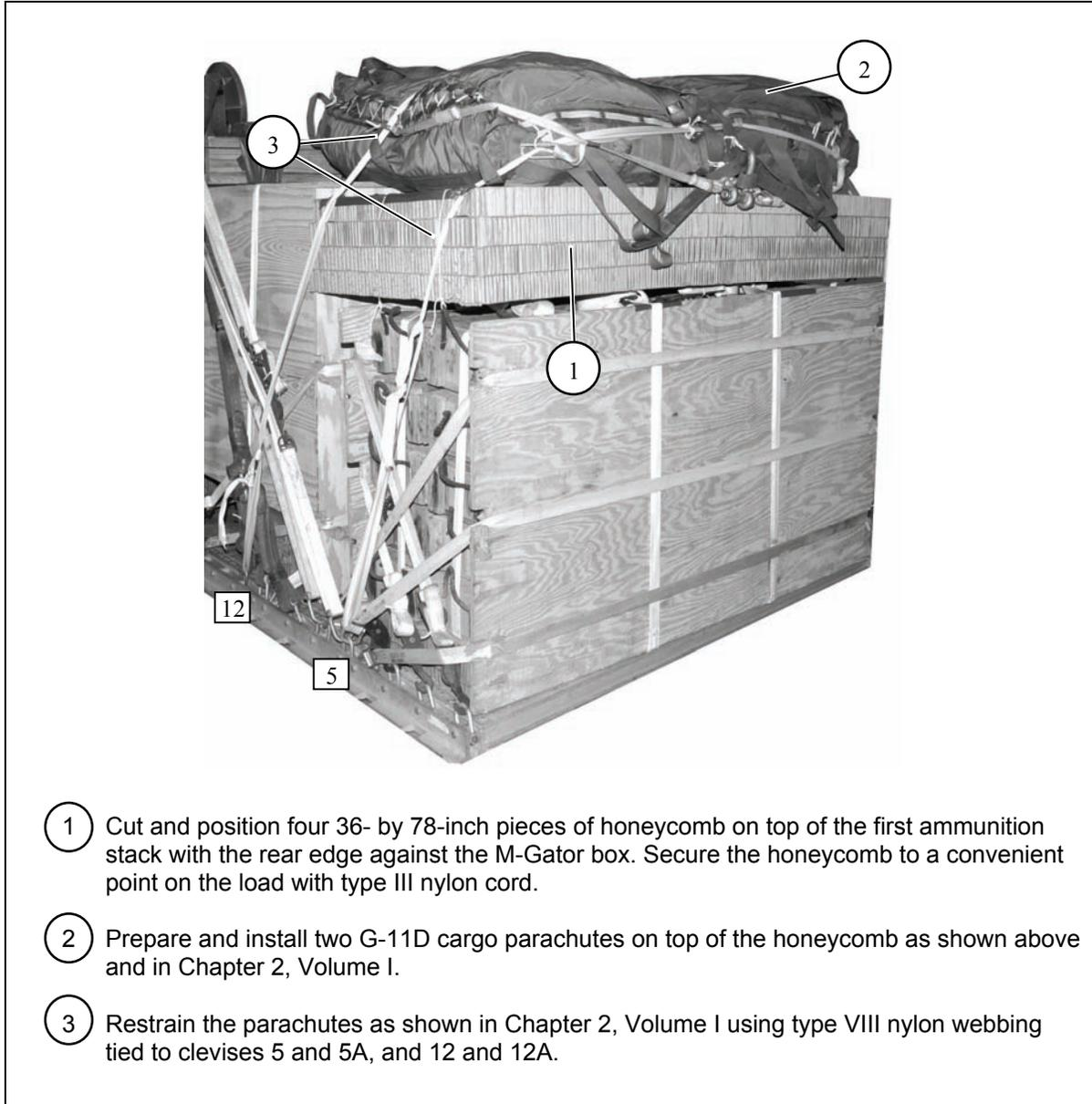
Figure 10-25. Cargo Parachute Stowed
