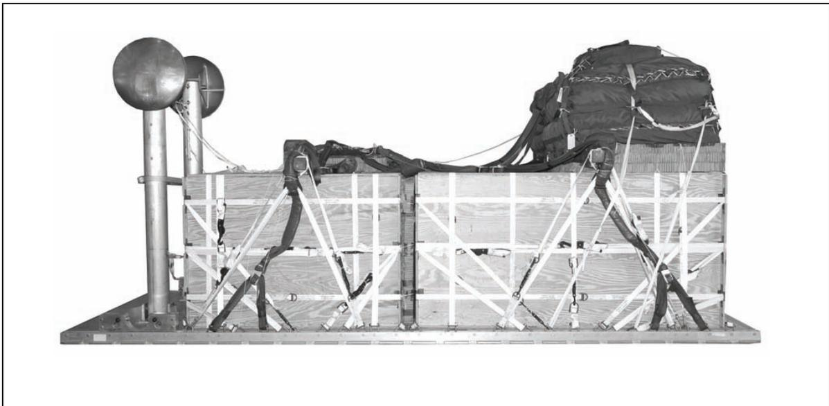
Figure 11-1. Mass Supply Load Rigged on DRAS Platform
