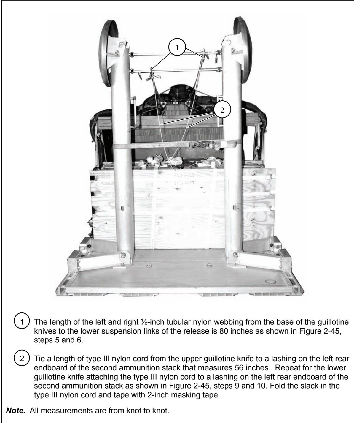
Figure 10-28. Mast Release Knives Installed
