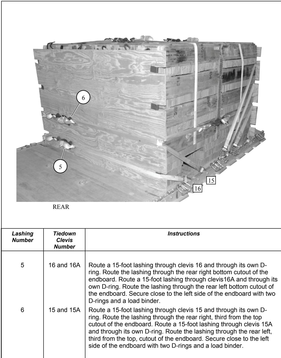
**Figure 9-6. Lashings Installed for First Stack (Continued)**
