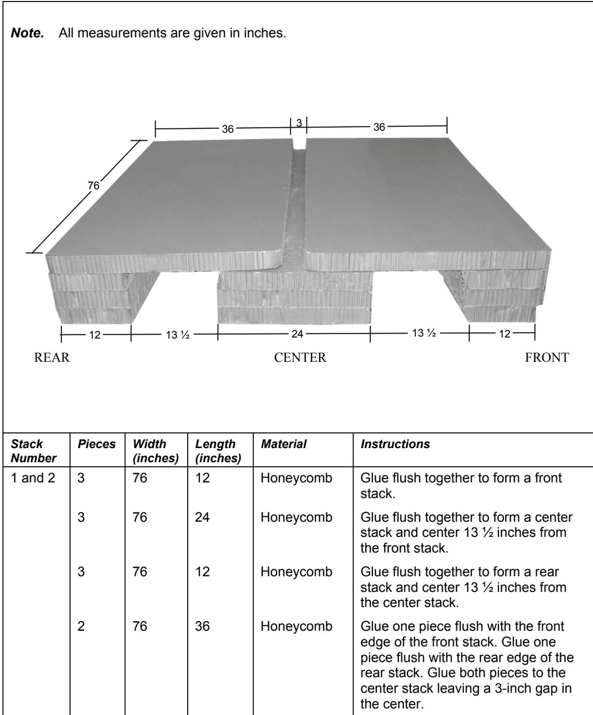
Figure 9-3. Honeycomb Stacks Prepared
