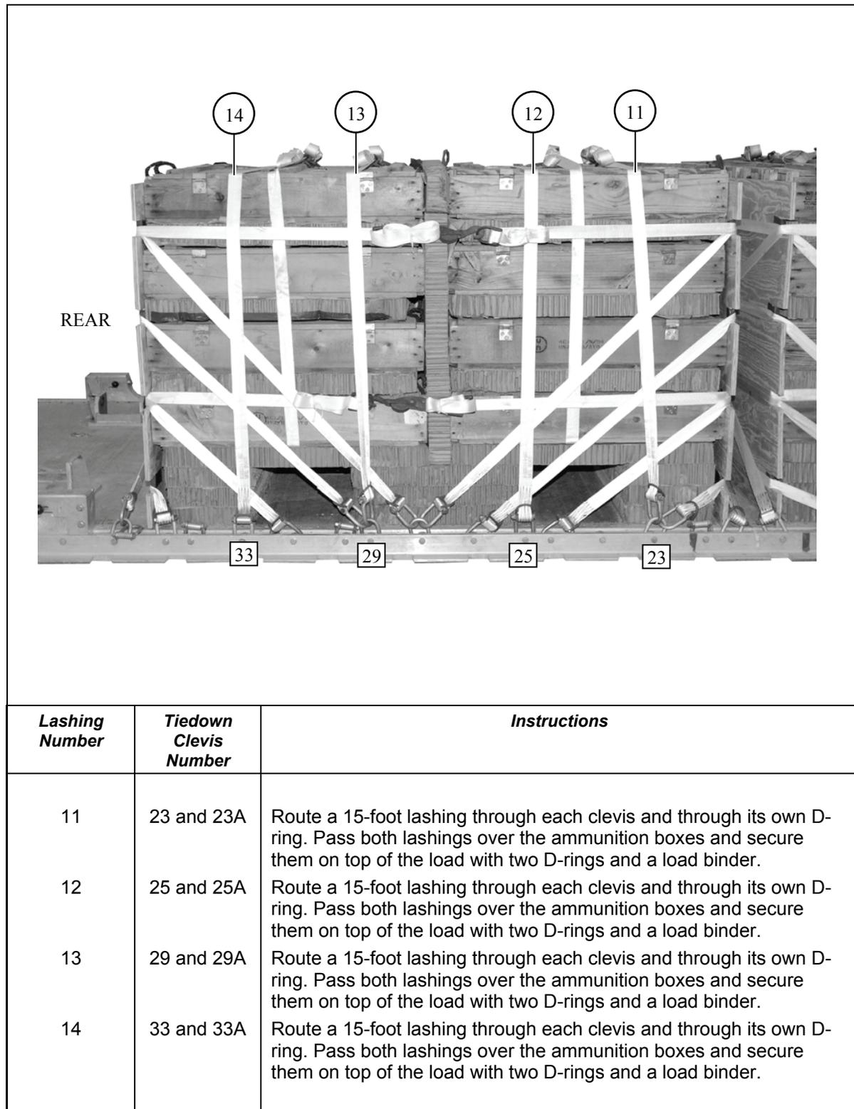
**Figure 9-8. Lashings Installed for Second Stack (Continued)**
