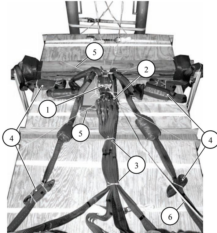
① Cut two 12- by 18-inch pieces of honeycomb and glue together. Tape the edges and position and center the honeycomb to the front of the rear ACS. Secure the honeycomb to a convenient point on the load using type III nylon cord. Center the M-1 release on the honeycomb stack.
