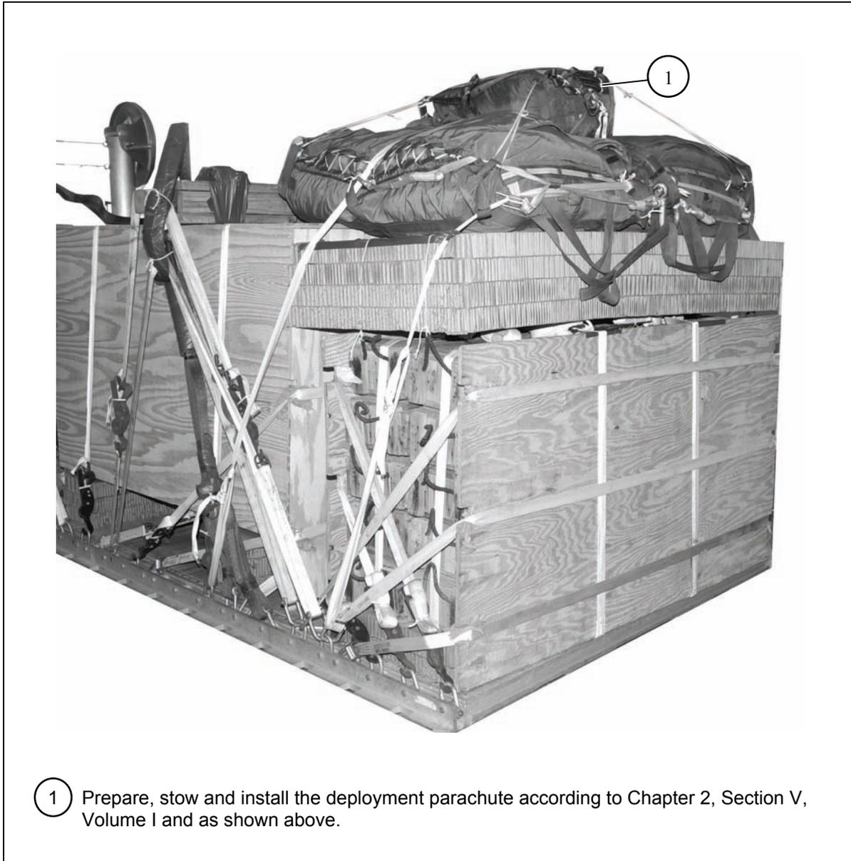
**Figure 10-26. Deployment Parachute Installed**
