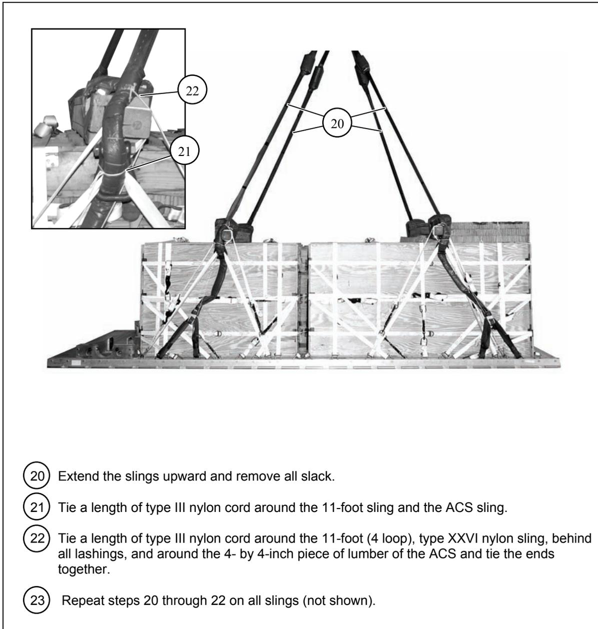
**Figure 11-15. Suspension Slings Installed and Secured (Continued)**
