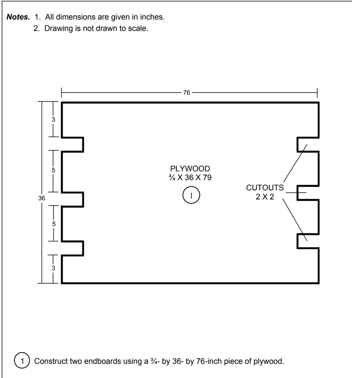
Figure 10-19. Endboards Constructed
