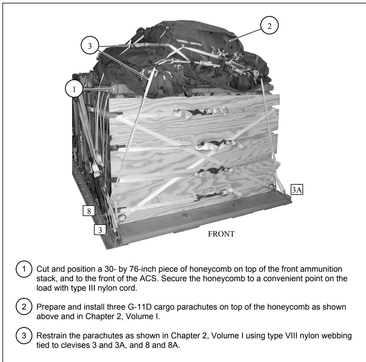
Figure 9-11. Cargo Parachute Stowed
