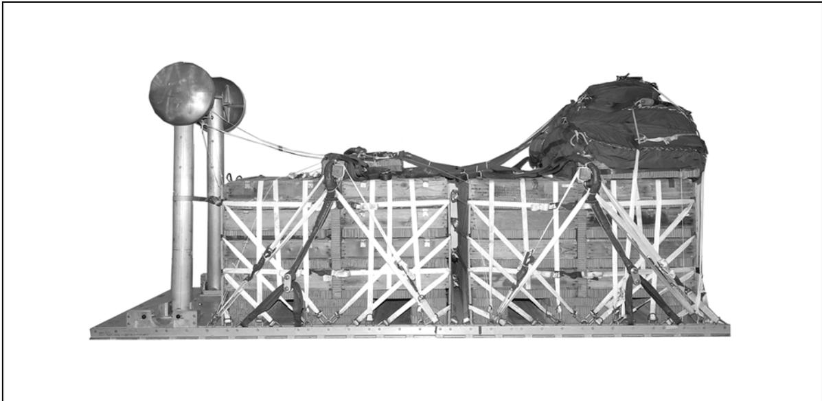
Figure 9-1. 105-mm Ammunition Mass Supply Load Rigged on DRAS Platform
