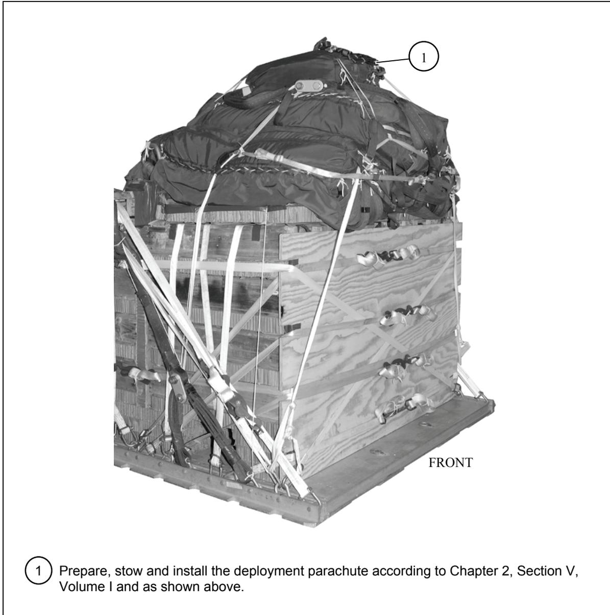
**Figure 9-12. Deployment Parachute Installed**
