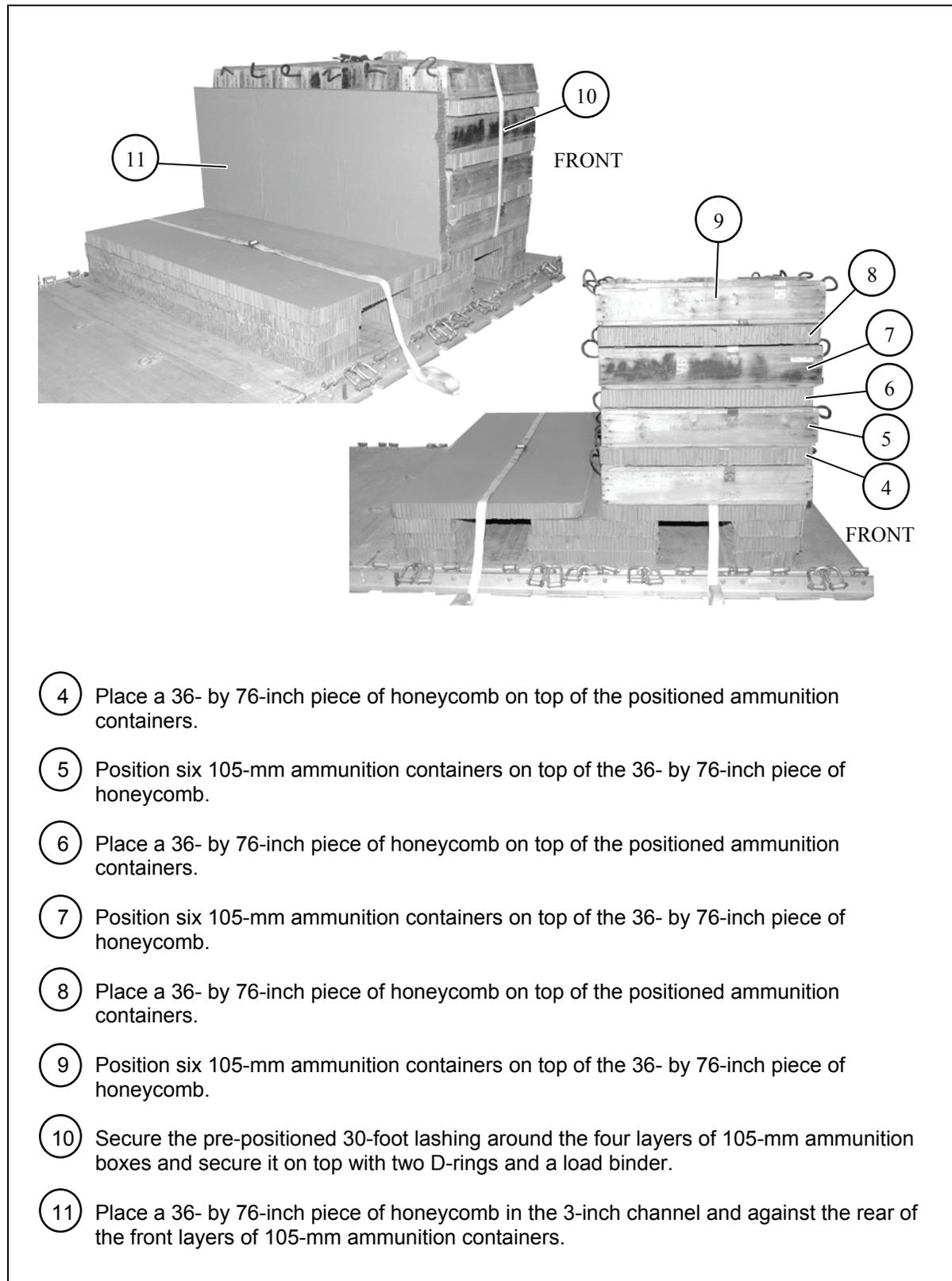
**Figure 9-4. Honeycomb Positioned and Ammunition Secured (Continued)**
