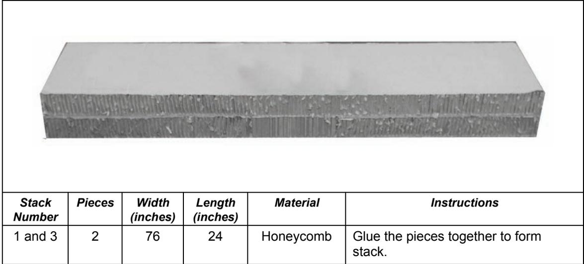
**Figure 10-3. Honeycomb Stacks Prepared**
