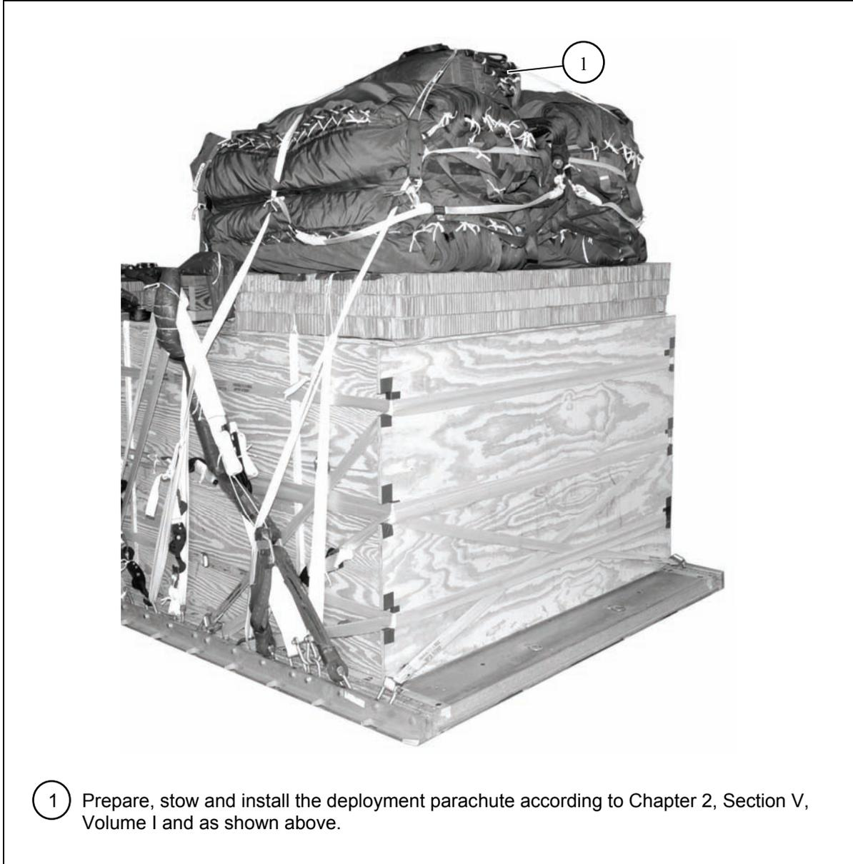
**Figure 11-17. Deployment Parachute Installed**
