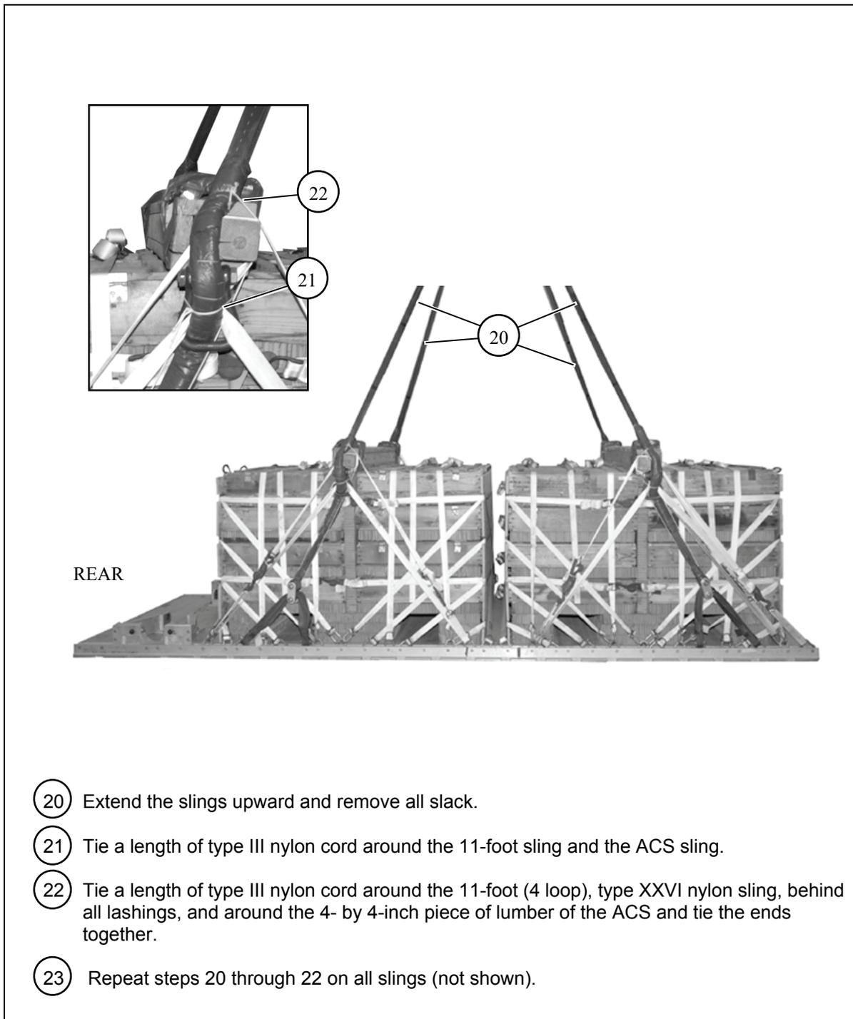
**Figure 9-10. Suspension Slings Installed and Secured (Continued)**
