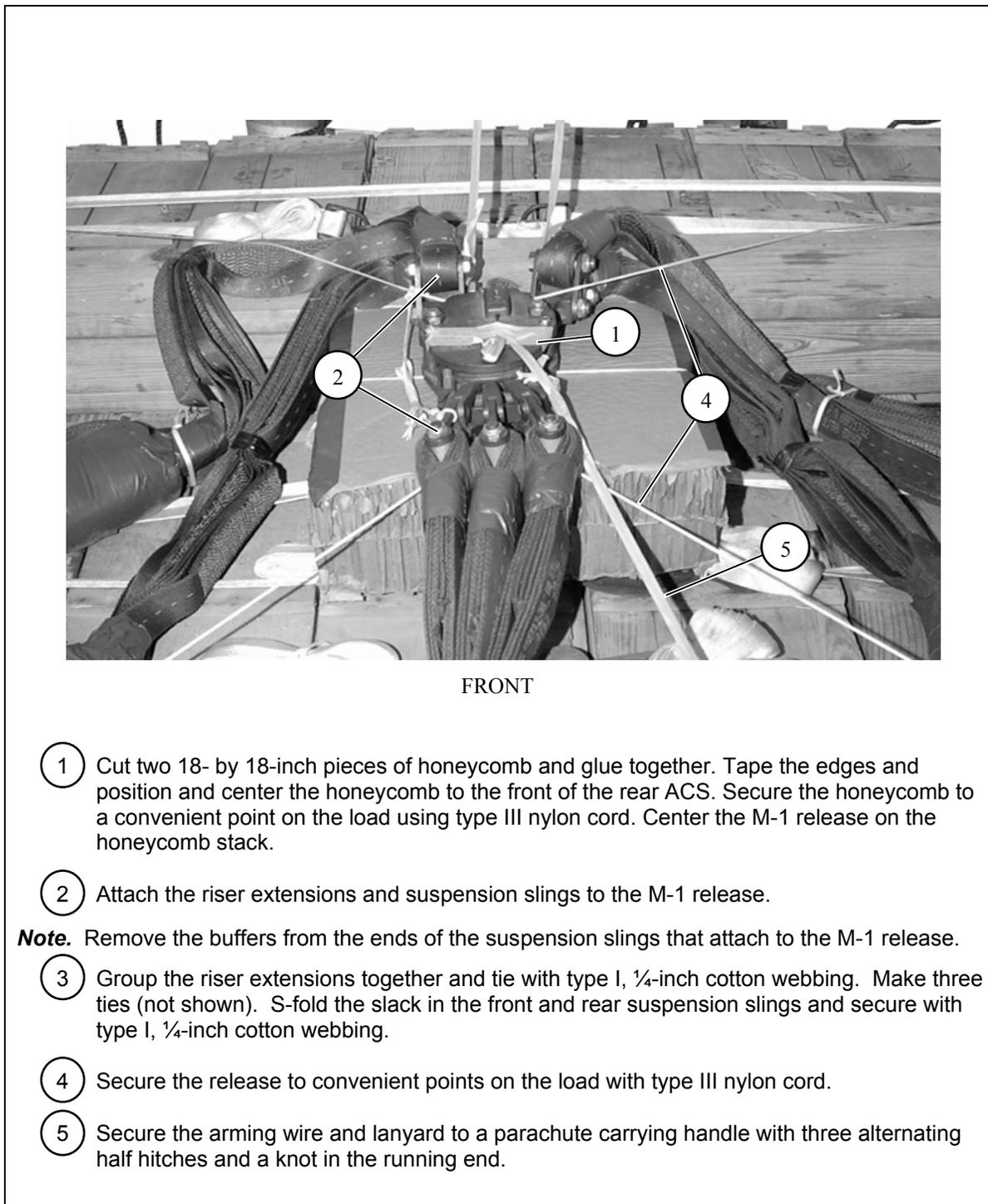
Figure 9-13. M-1 Cargo Parachute Release Installed
