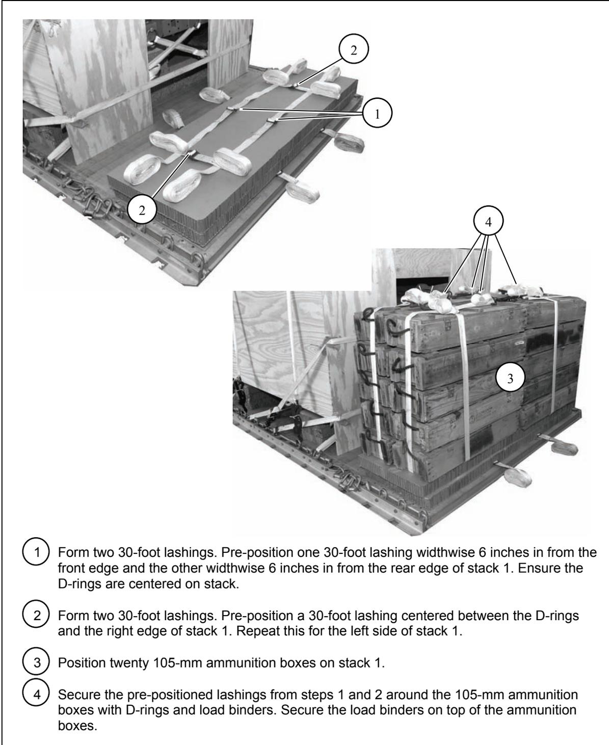
**Figure 10-16. First Ammunition Stack Positioned**
