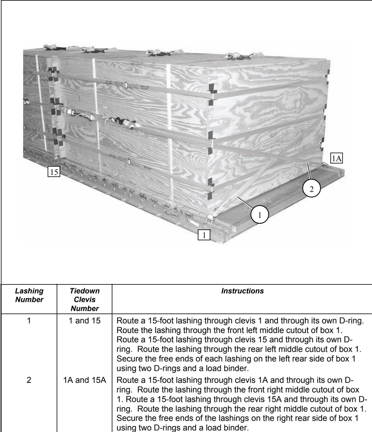
**Figure 11-6. Lashings 1 and 2 Installed**
