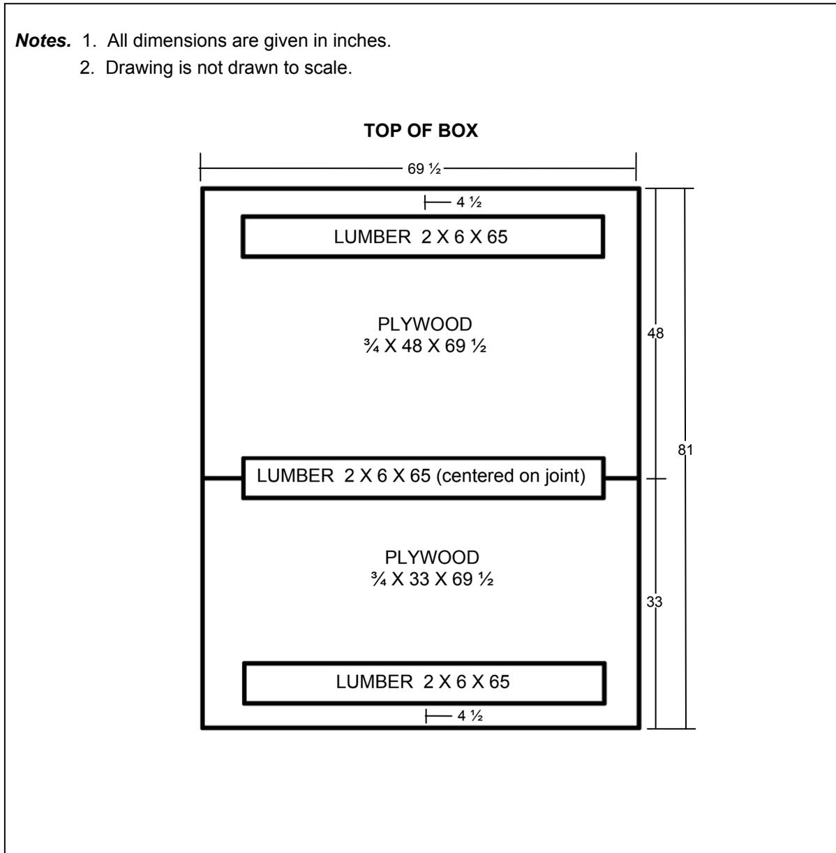
Figure 10-10. M-Gator Box Built
