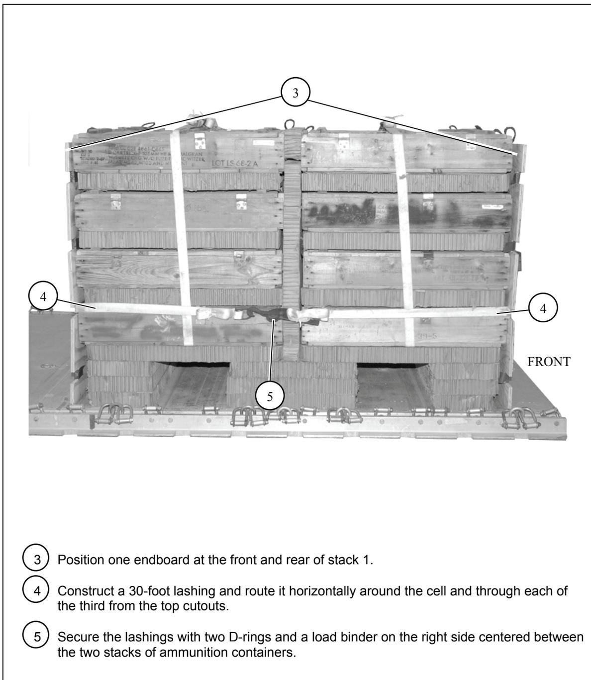
Figure 9-5. Endboards Constructed and Placed (Continued)
