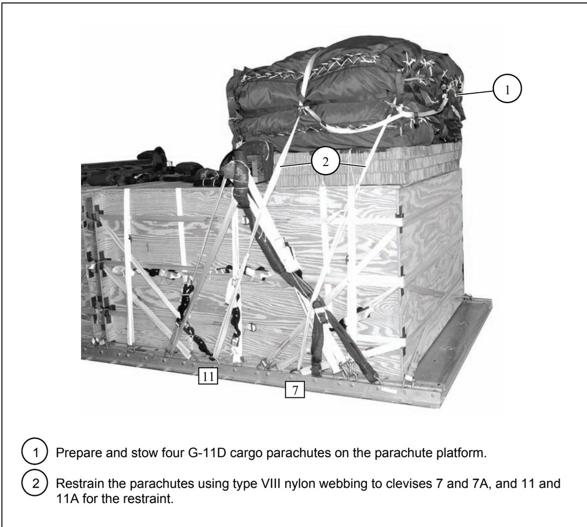
Figure 11-16. Cargo Parachute Stowed
