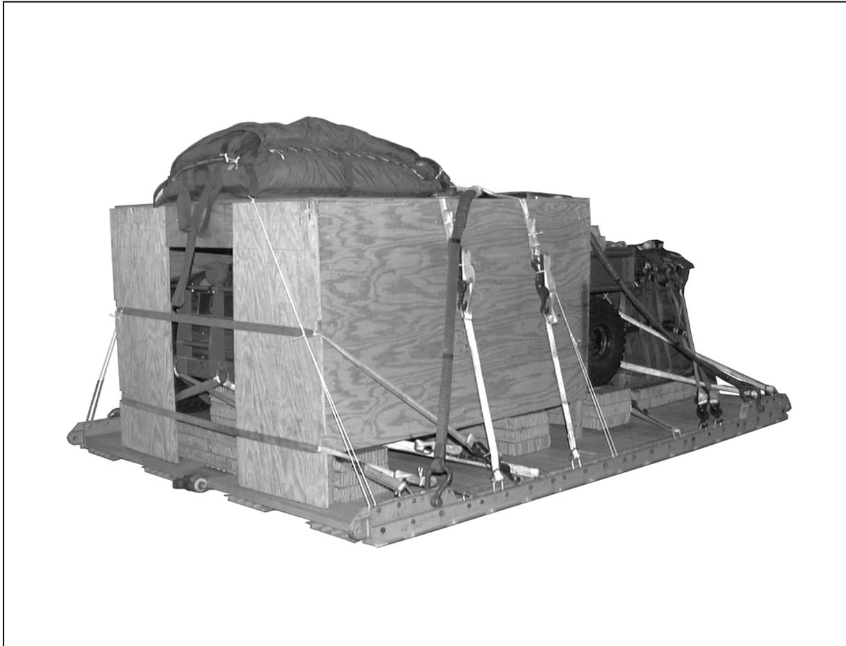
**Figure 3-14. Cargo Parachute Stowed**
