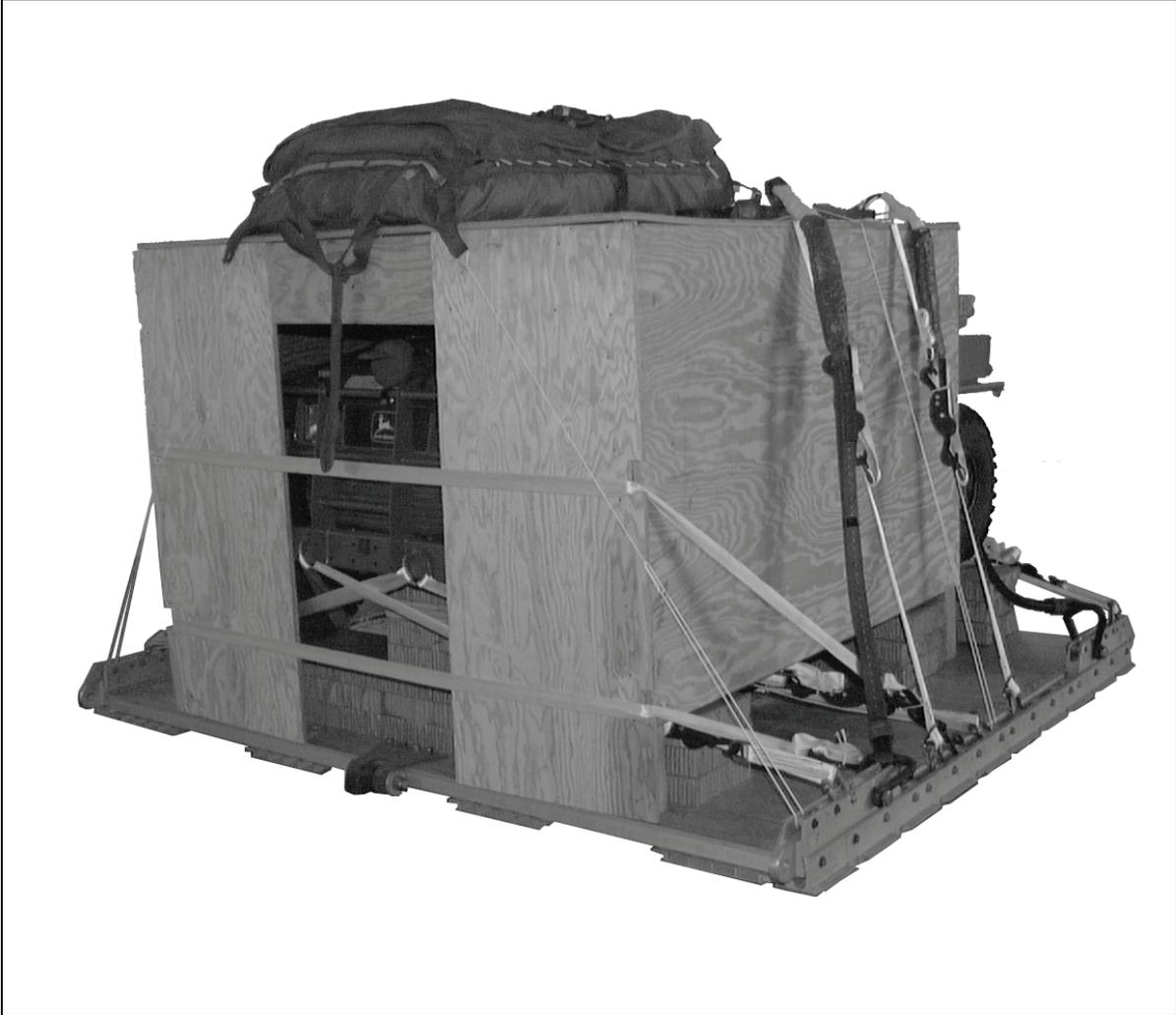
**Figure 1-14. Cargo Parachute Stowed**
