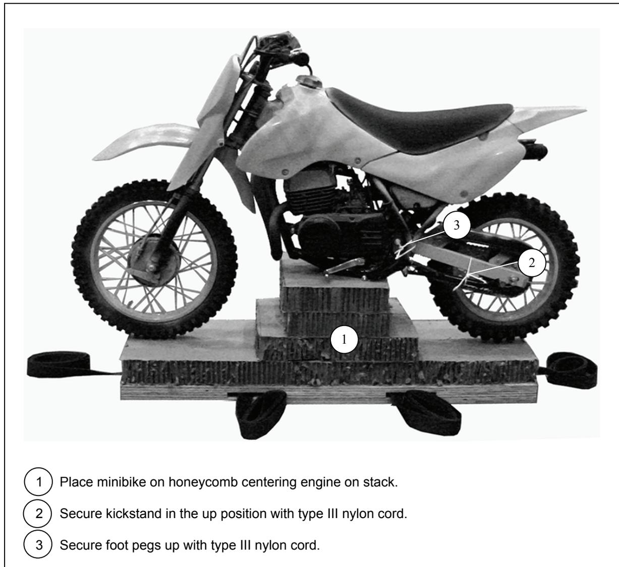
**Figure 5-6. Minibike Positioned on Honeycomb**
