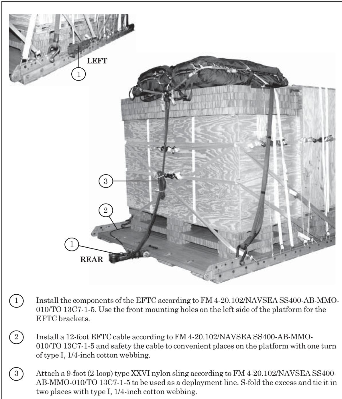
**Figure 2-38. Extraction System Installed**
