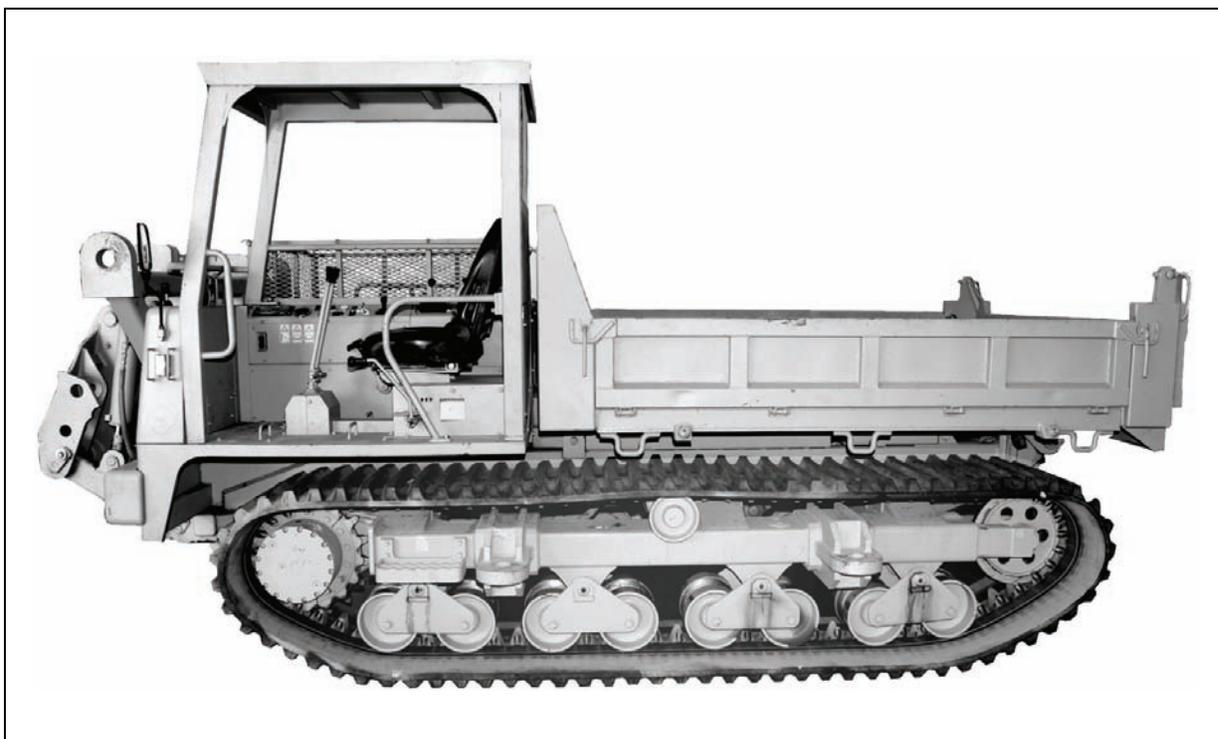
Figure 2-1. IC45-2 IHI Crawler Carrier
