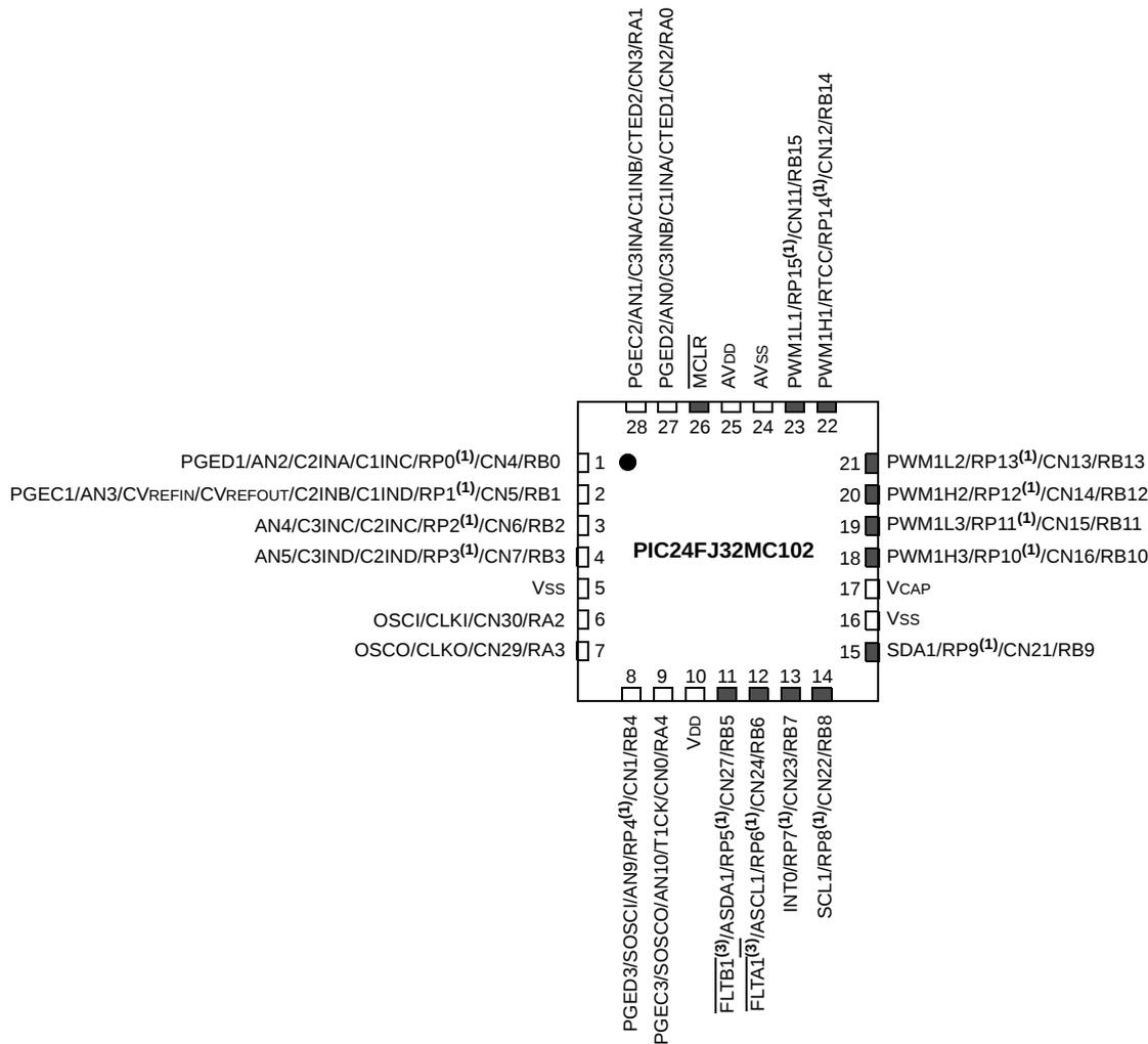
**Note 1:** The RPN pins can be used by any remappable peripheral. See [Table 1](#) for the list of available peripherals.
