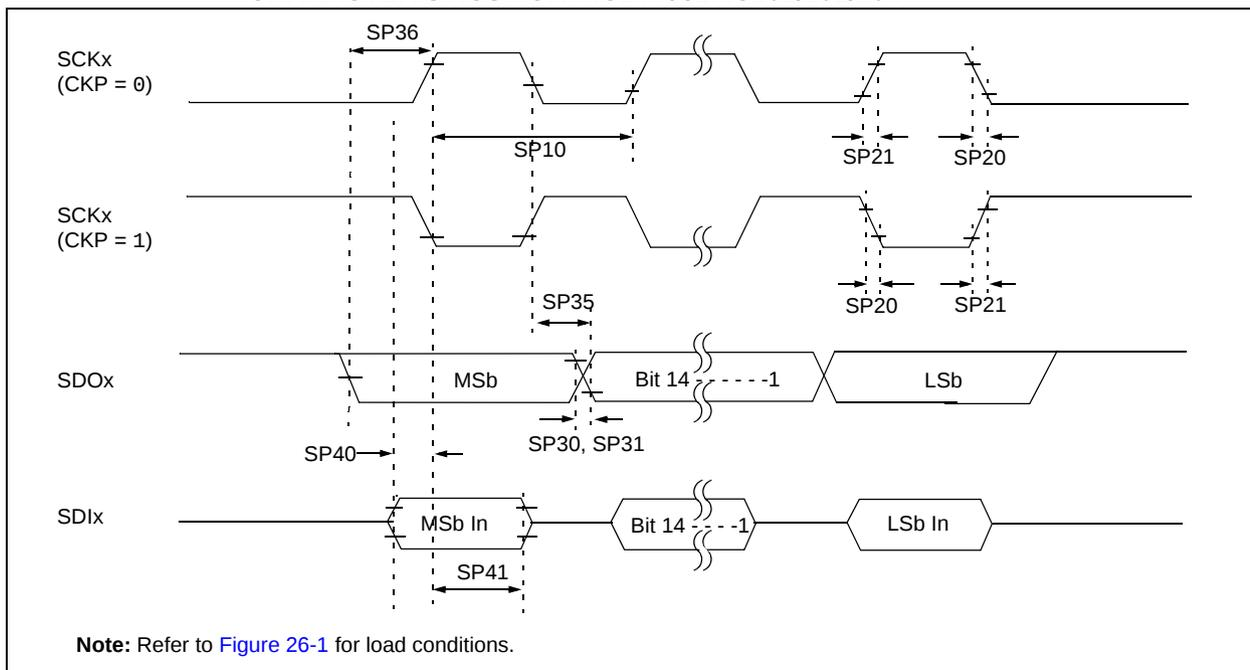
**TABLE 26-39: SPIx MASTER MODE (FULL-DUPLEX, CKE = 1, CKP = x, SMP = 1) TIMING REQUIREMENTS FOR PIC24FJ32MC101/102/104**
