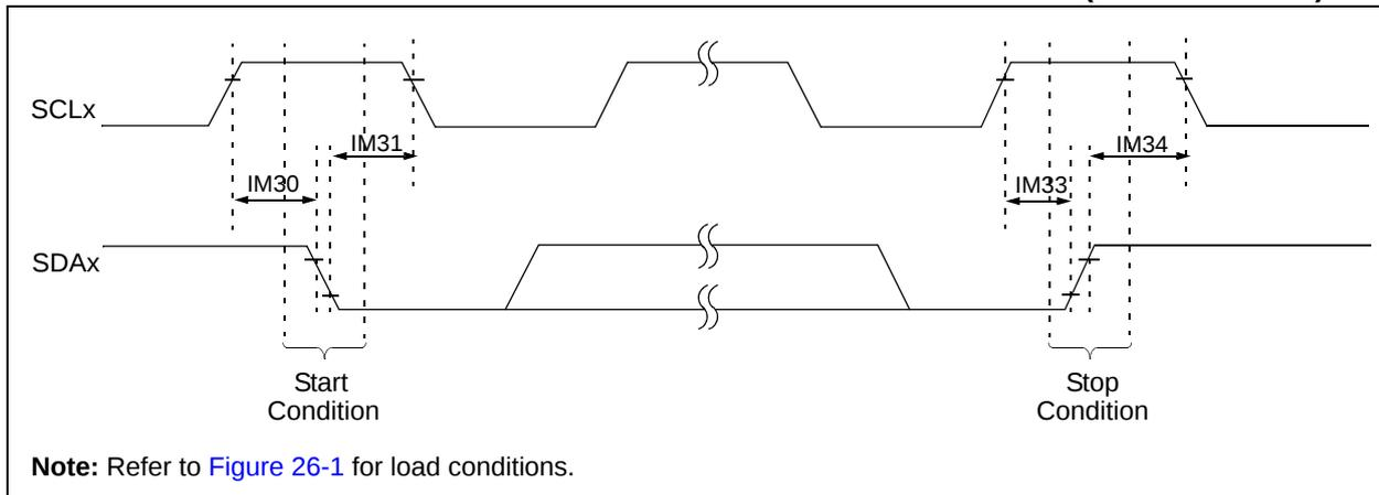
**FIGURE 26-28: I2Cx BUS DATA TIMING CHARACTERISTICS (MASTER MODE)**
