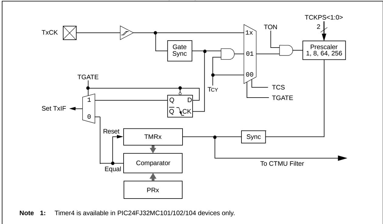
FIGURE 12-3: TIMER3 AND TIMER5<sup>(1)</sup> (16-BIT) BLOCK DIAGRAM
