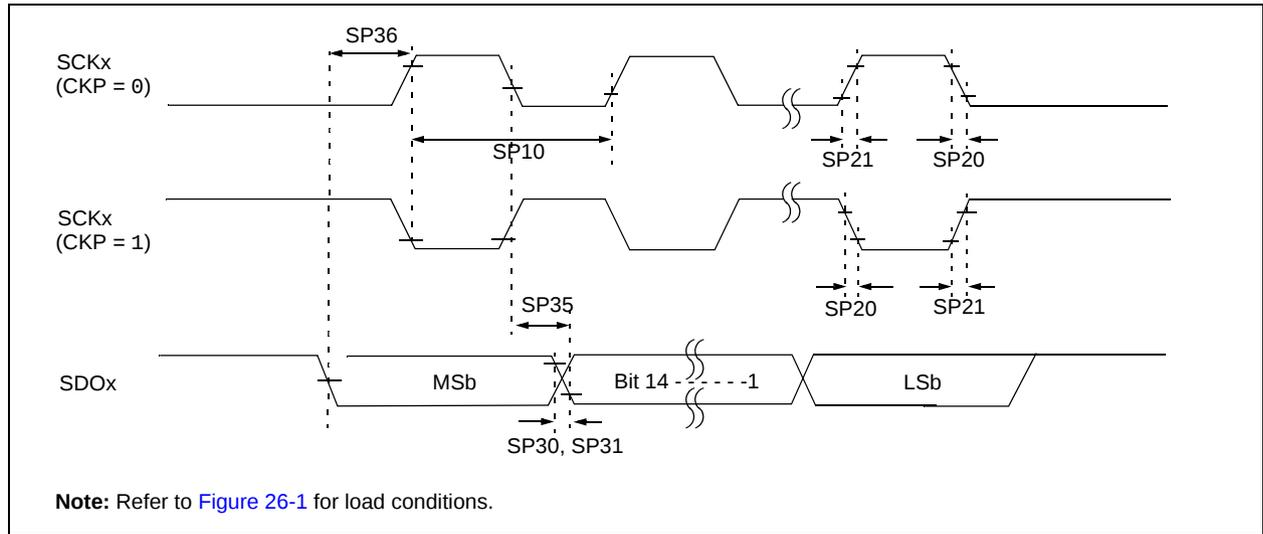
**TABLE 26-30: SPIx MASTER MODE (HALF-DUPLEX, TRANSMIT ONLY) TIMING REQUIREMENTS FOR PIC24FJ16MC101/102**
