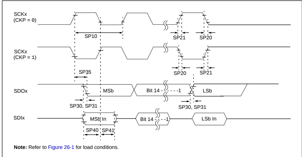
**TABLE 26-40: SPIx MASTER MODE (FULL-DUPLEX, CKE = 0, CKP = X, SMP = 1) TIMING REQUIREMENTS FOR PIC24FJ32MC101/102/104**
