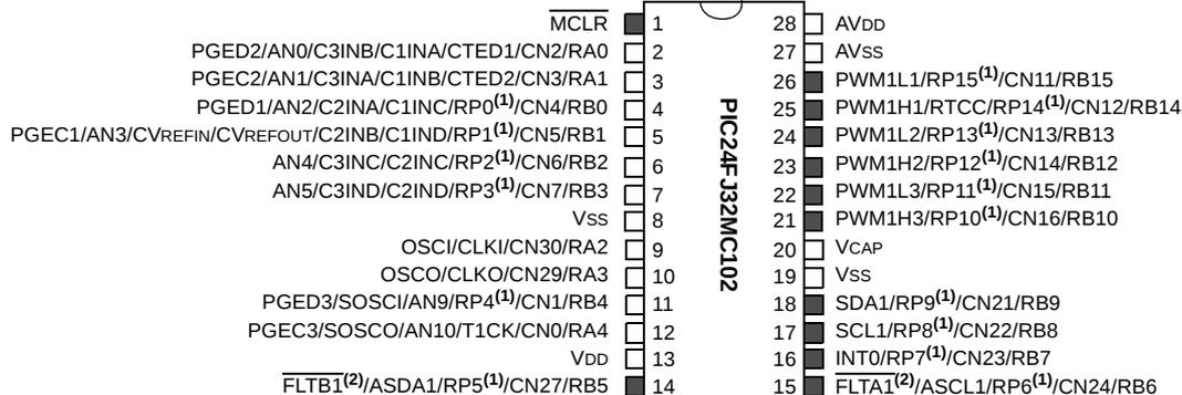
**Note 1:** The RPn pins can be used by any remappable peripheral. See [Table 1](#) for the list of available peripherals.
