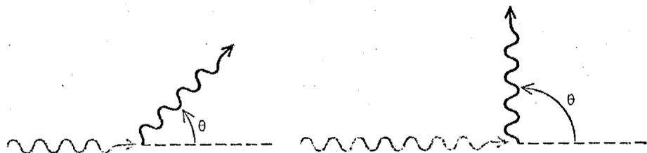
CERENKOV RADIATION would be emitted continuously by an electrically charged tachyon moving in a vacuum. The characteristic angle ( $\theta$ ) at which the photons (black) would be emitted would depend only on the speed of the tachyon: the faster the tachyon, the greater the angle. Ordinary charged particles, such as the electron, emit Cerenkov radiation only when they move through a substance faster than the speed of light in the substance.
