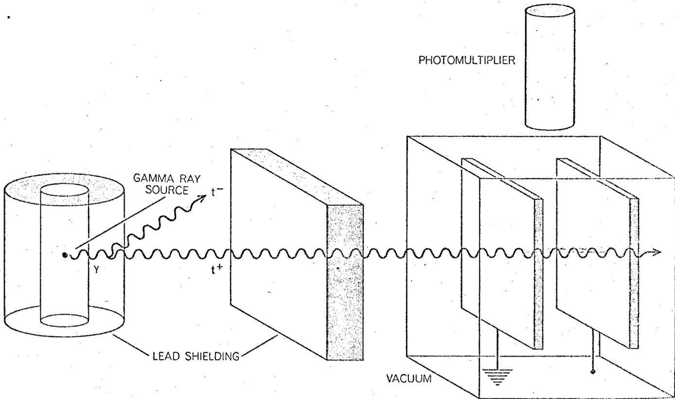
EXPERIMENT designed to detect charged tachyons by means of their Cerenkov radiation was carried out two years ago by Torsten Alväger and Michael N. Kreisler at Princeton University. They used a radioactive cesium source to provide high-energy gamma rays ( $\gamma$ ), which were allowed to hit a lead shield that prevented them from reaching the detection apparatus directly. Pairs of charged tachyons could be produced by the gamma ray photons in
